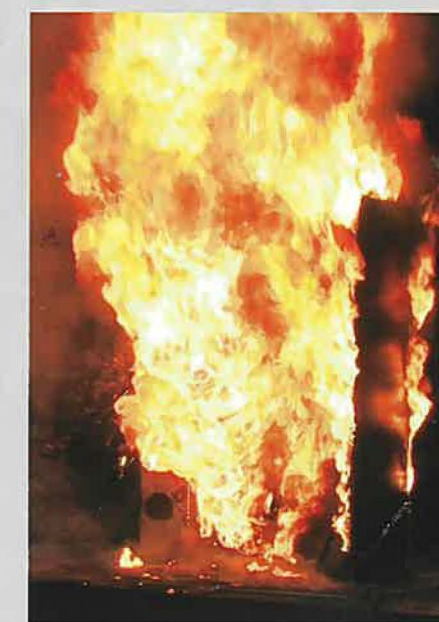
FIGURE 2. NMC fire development during large-scale free burn test: near time of ignition (left), near time of predicted sprinkler operation (centre), peak heat release rate (right).
