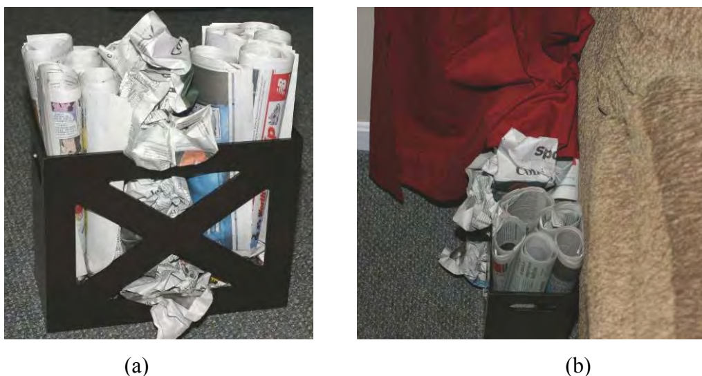
Figure 12: (a) Ignition source and (b) Magazine rack relative to loveseat and curtain.
