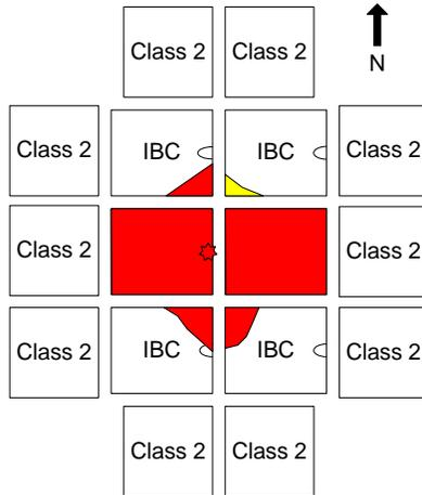
**Figure 3-4: Test 1 Damage - 1<sup>st</sup> Tier**
