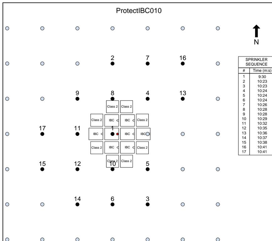
**Figure 3-26: Test 10 - Sprinkler Operation Pattern**
