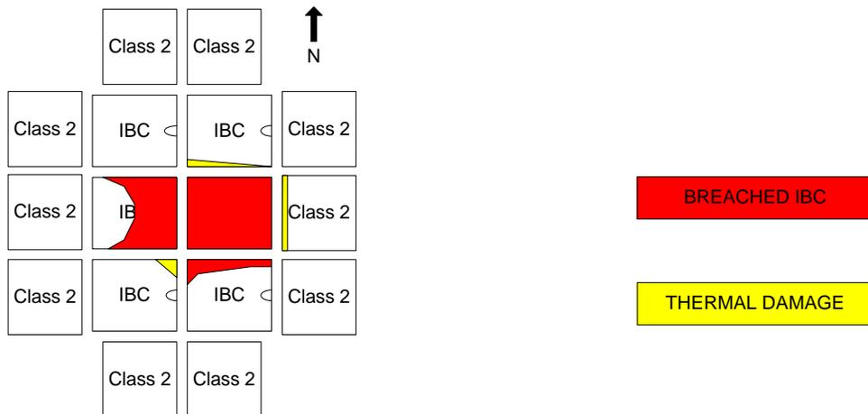
**Figure 3-5: Test 1 Damage - 2<sup>nd</sup> Tier**
