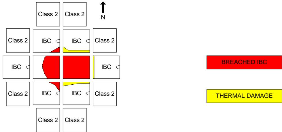
**Figure 3-11: Test 2 Damage - 2<sup>nd</sup> Tier**
