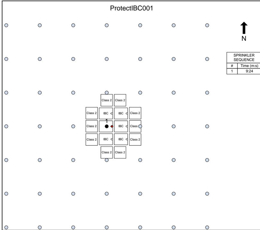
**Figure 3-2: Test 1 - Sprinkler Operation Pattern**
