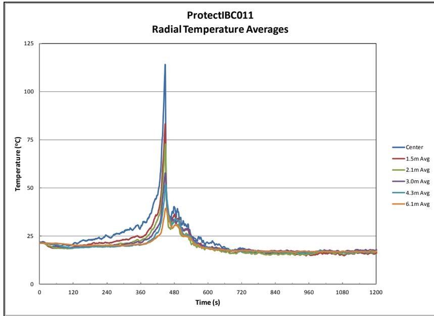
Figure A-11: Test 11 - Ceiling Gas Temperatures
