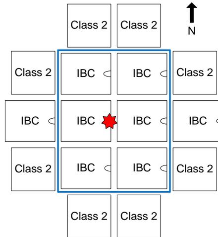
**Figure 2-16: Acceptable Damage Area for Stacked IBC Array**
