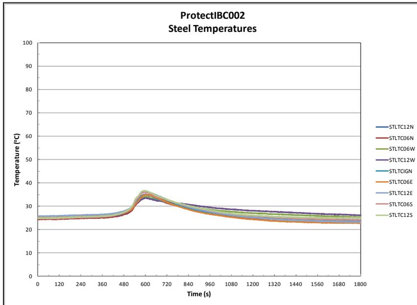
Figure A-4: Test 2 - Ceiling Steel Temperatures
