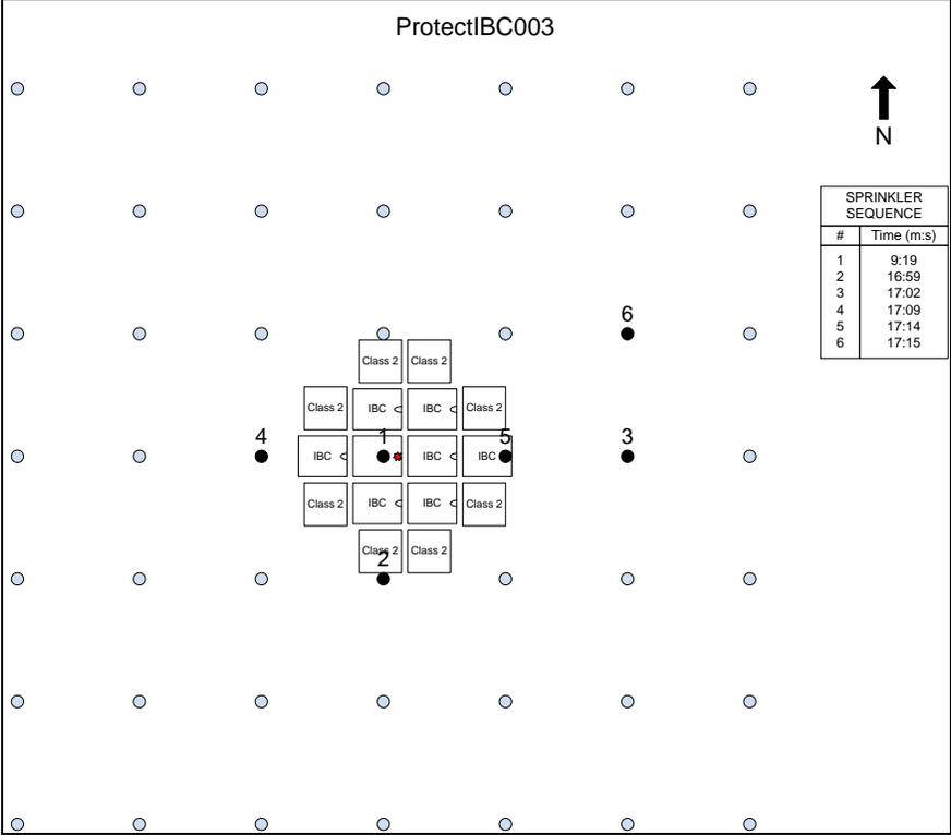
**Figure 3-13: Test 3 - Sprinkler Operation Pattern**
