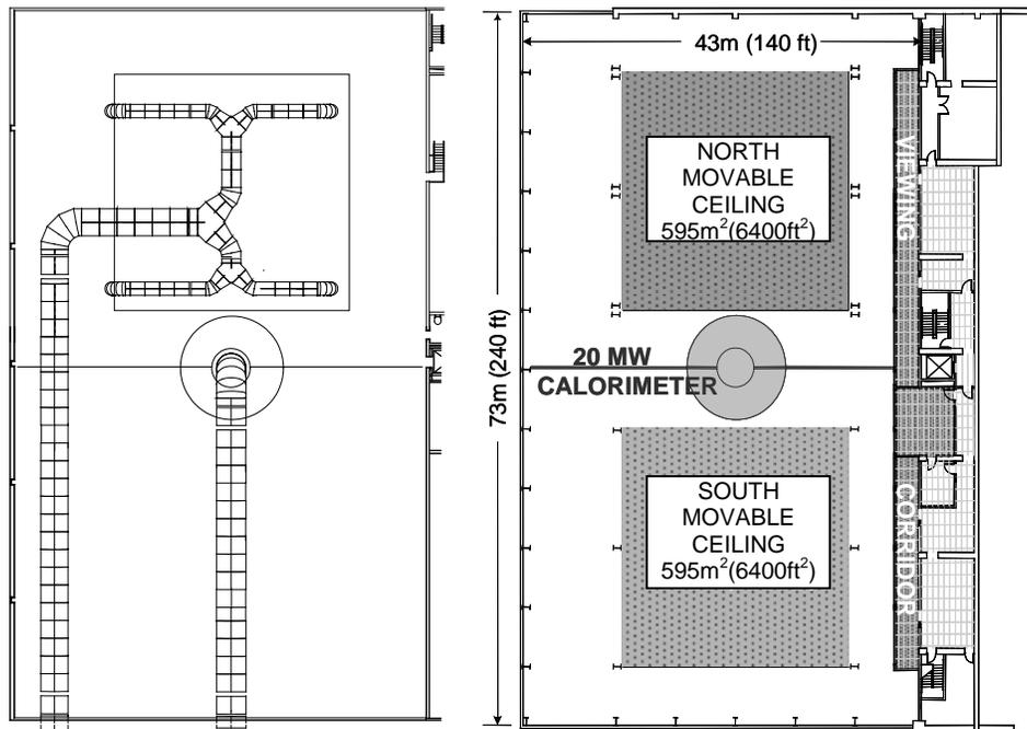
**Figure 2-1: Illustration of AECS ducting and LBL Test Locations**
