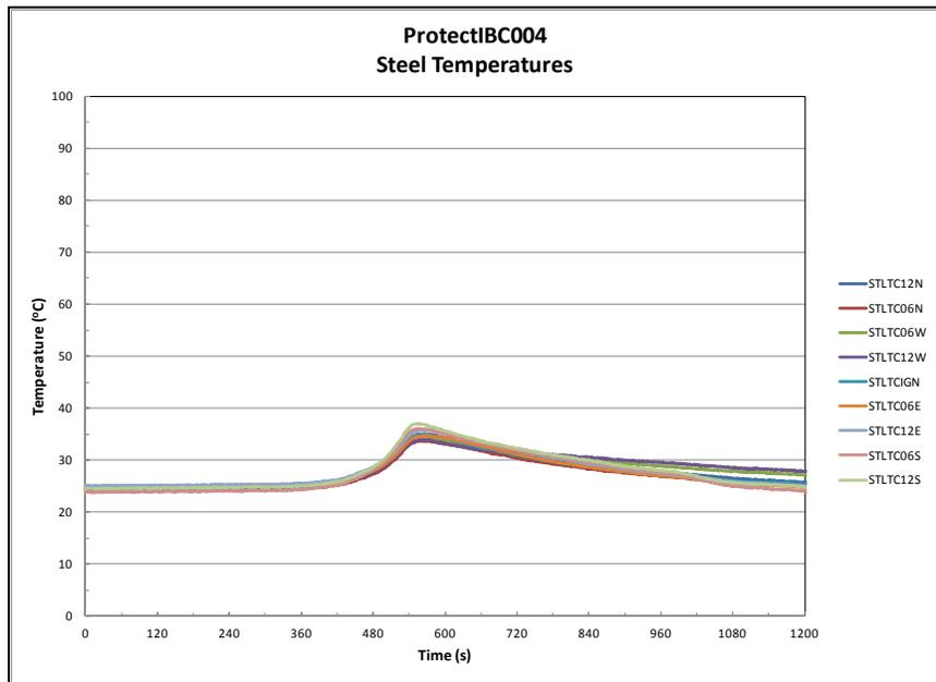
Figure A-8: Test 4 - Ceiling Steel Temperatures
