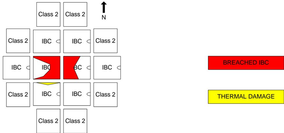
**Figure 3-24: Test 4 Damage - 2<sup>nd</sup> Tier**
