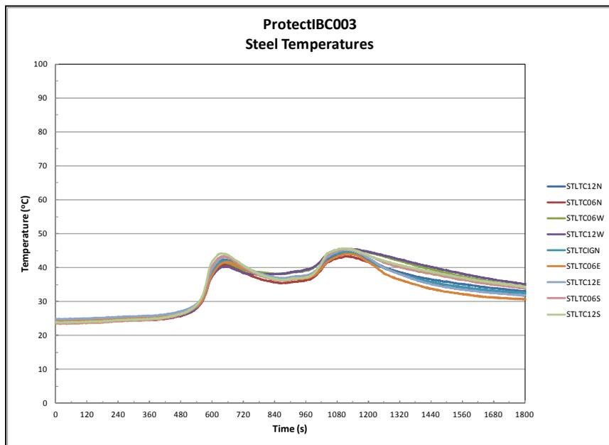
**Figure A-6: Test 3 - Ceiling Steel Temperatures**
