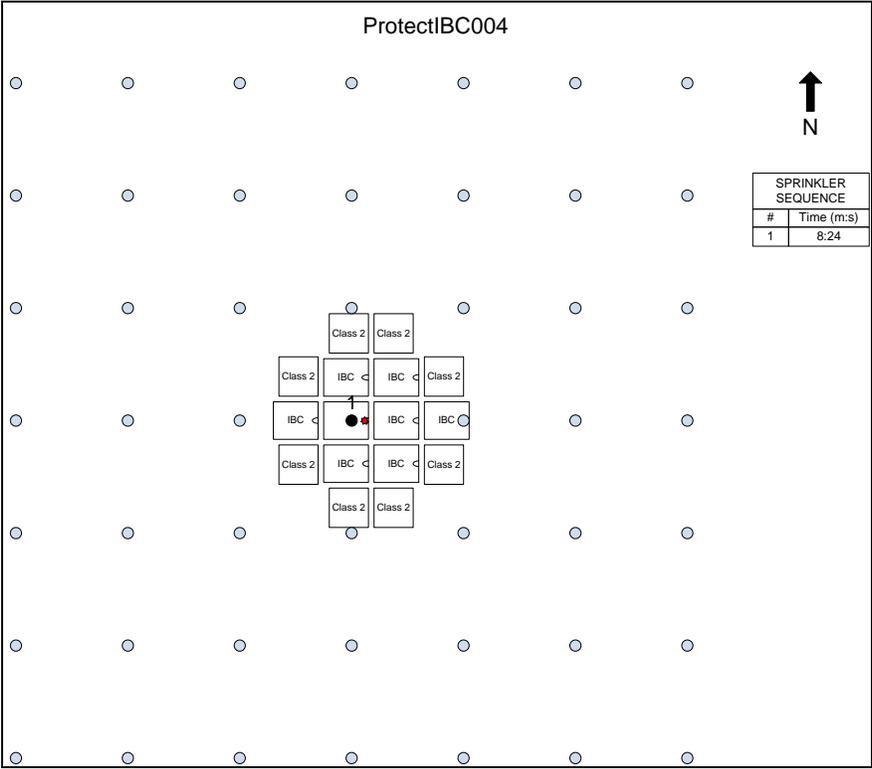
**Figure 3-20: Test 4 - Sprinkler Operation Pattern**
