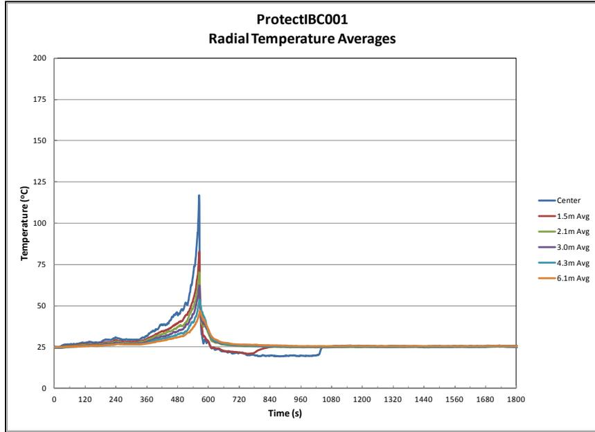
Figure A-1: Test 1 - Ceiling Gas Temperatures
