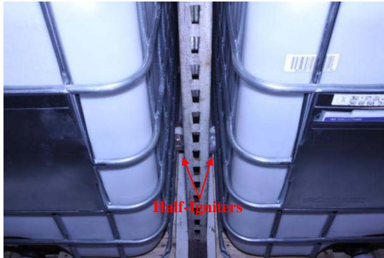
**Figure 2-15: Photo of Igniter Placement for Rack Storage Test**
