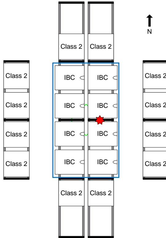
**Figure 2-17: Acceptable Damage Area for Rack Storage Array**
