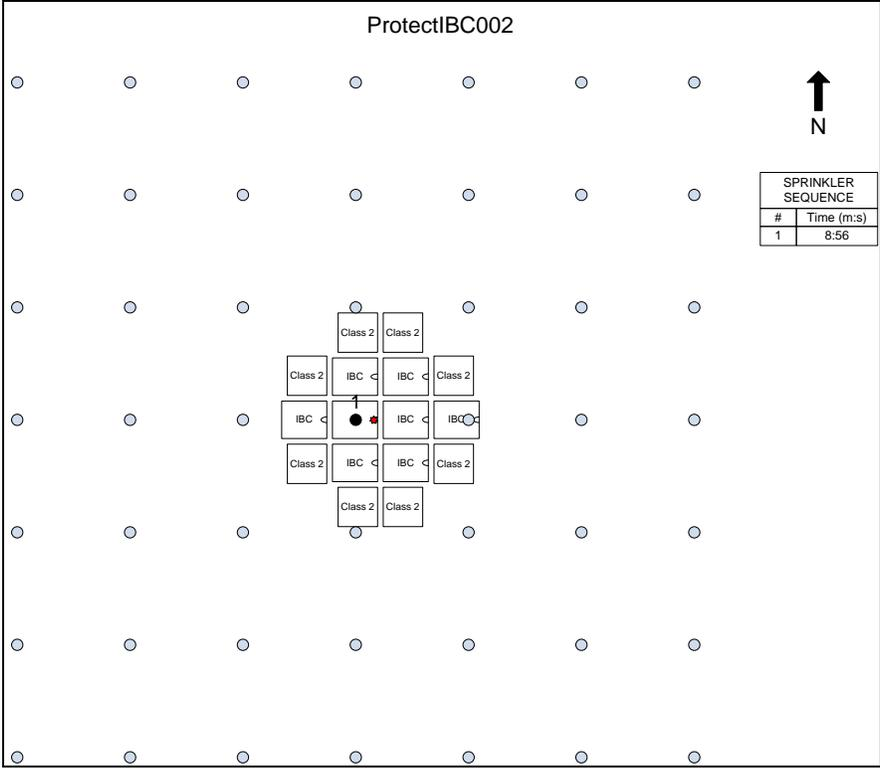
**Figure 3-7: Test 2 - Sprinkler Operation Pattern**
