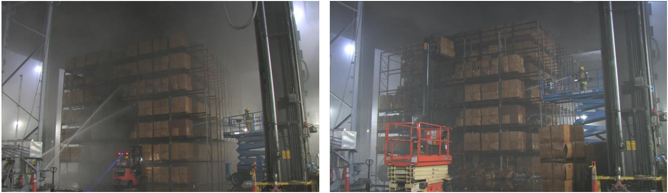
Figure 3-20: Images taken during the manual firefighting process after Test LS-1
