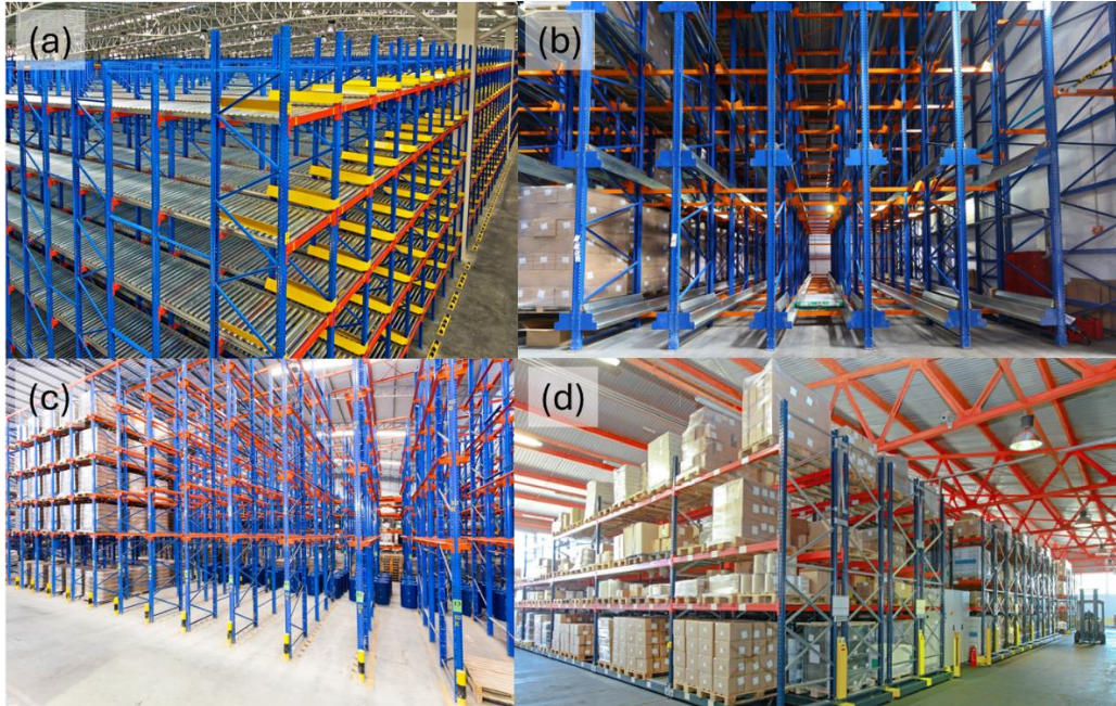
Figure 1-1: Commonly found multiple row racks in modern warehouses: (a) flow-through racks, (b) shuttle pallet systems, (c) drive-through racks, and (d) mobile racks
