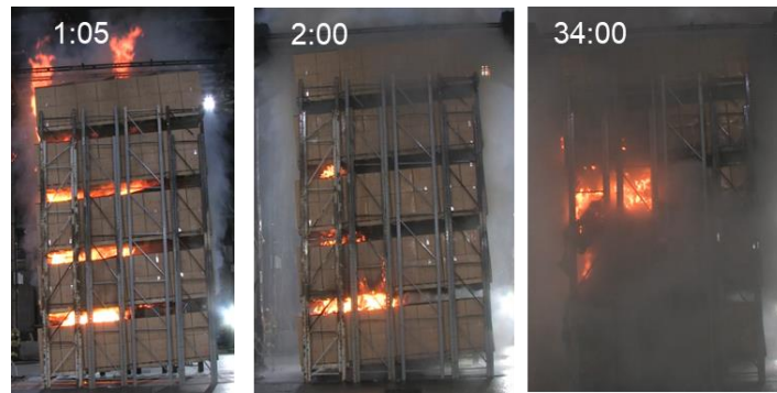
Figure 2-26: Images at various times during Test IS-7 in presence of sloped rack
