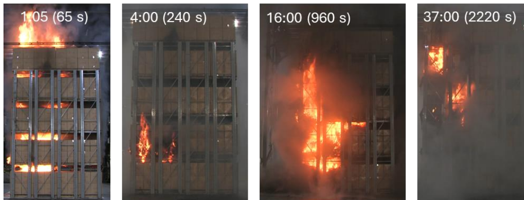
Figure 2-21: Images at various times during Test IS-4 using seamless CUP commodity under water application rate of 52 mm/min (1.28 gpm/ft 2 )
