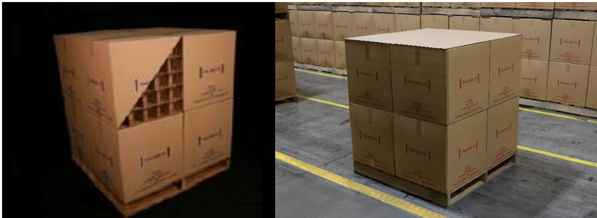
Figure 2-5: Images of standard CUP (left) and seamless CUP (right) commodities
