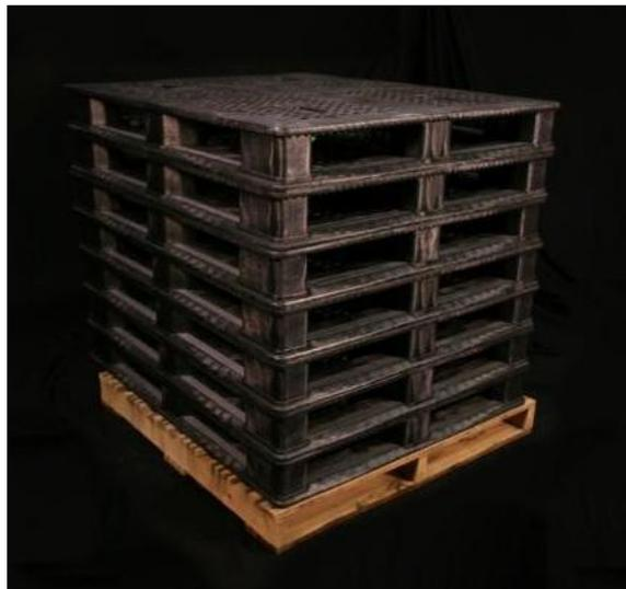
Figure 2-2: FM Global Standard Uncartoned Unexpanded Plastic (UUP) Test Commodity for Rack Storage Tests (Considered Exposed, Nonexpanded Group A Plastic per NFPA 13).
