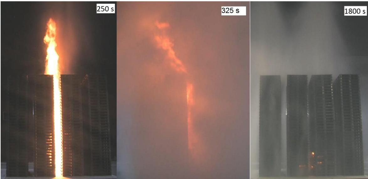
Figure 3-10: Photos of Test 6 from South Side at 250 s, 325 s and 1,800 s After Ignition.
