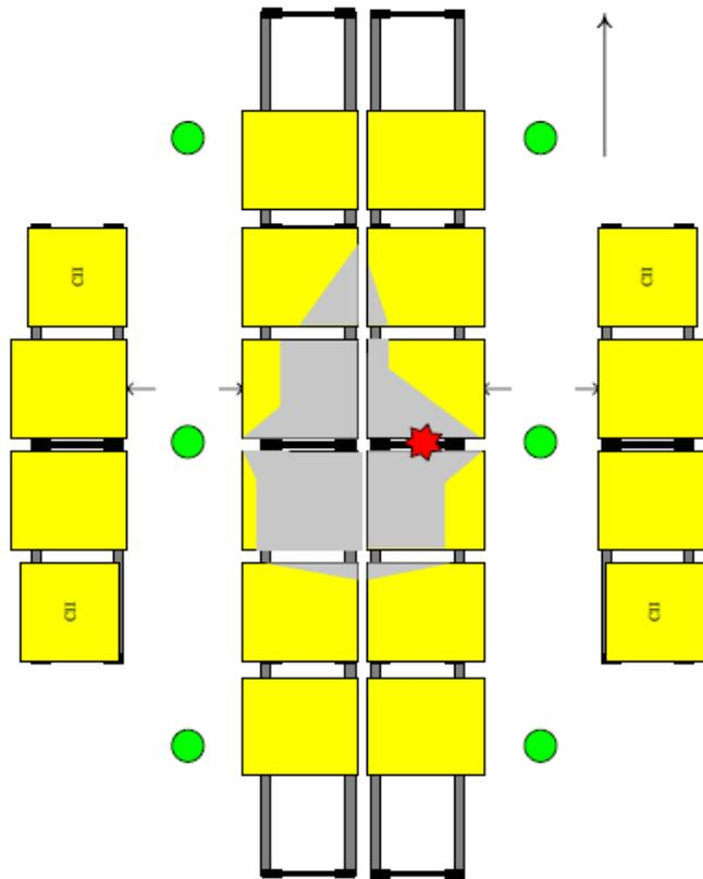
Figure 3-2: Extent of Fire Damage for Test 13.
