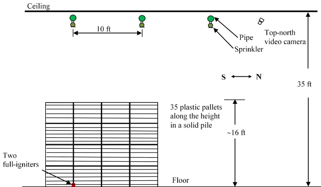
Figure 3-9: Plan and Elevation View of Test 6.
