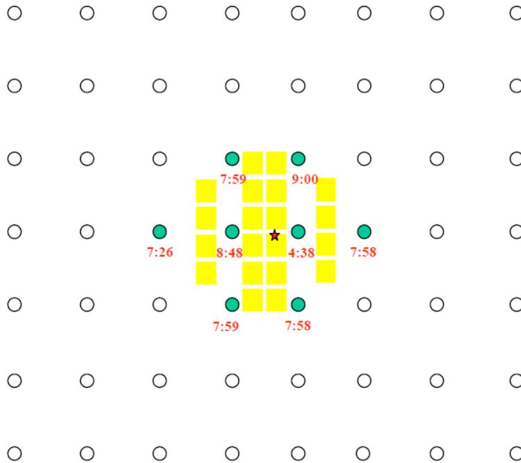
Figure 3-1: Sprinkler Actuation Sequence for Test 13.
