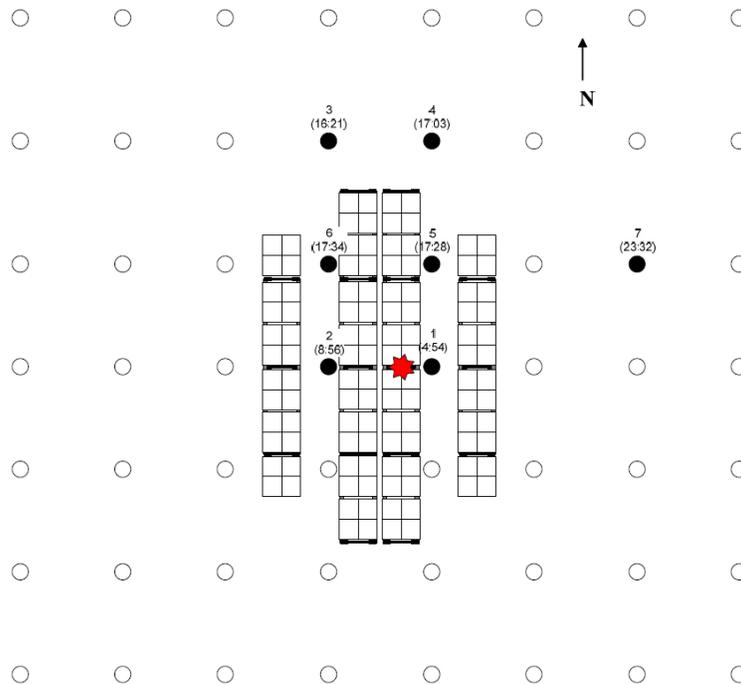
Figure 3-3: Sprinkler Actuation Sequence for Test 8.
