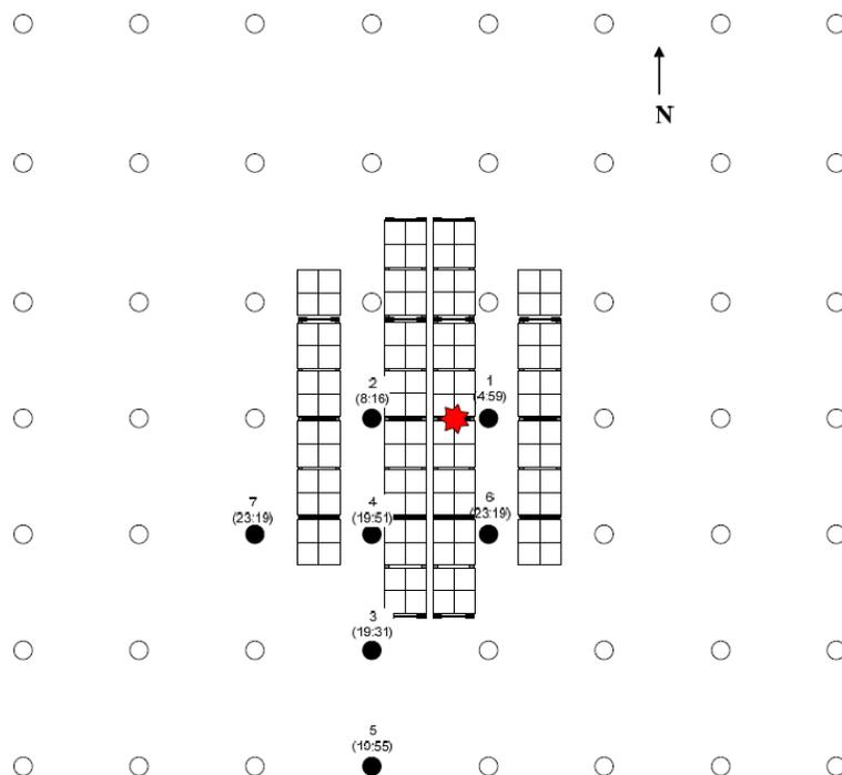
Figure 3-4: Sprinkler Actuation Sequence for Test 9.
