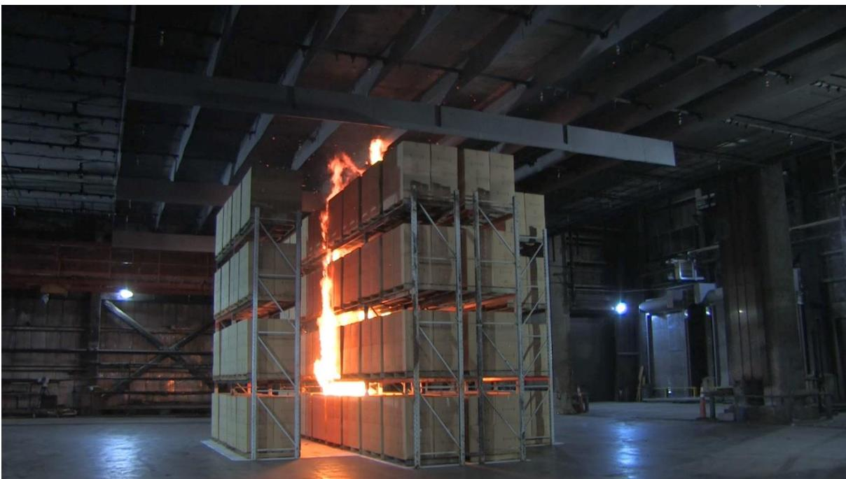
Figure B-12: Test #3 array at 1 min 15 s after ignition.
