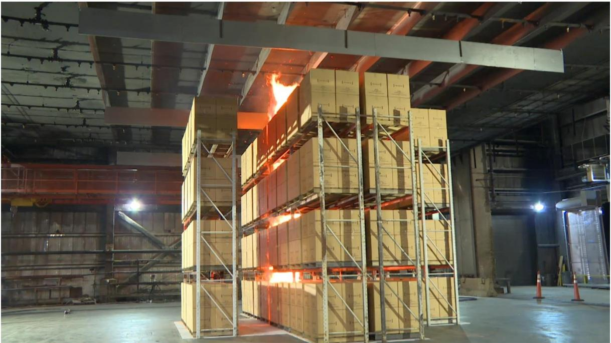
Figure B-6: Test #2 array at 1 min after ignition.
