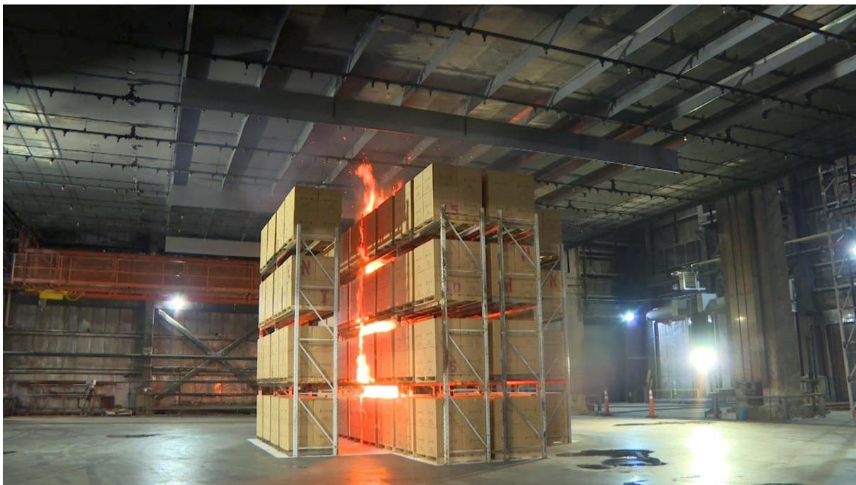
Figure B-2: Test #1 array at 1 min 15 s after ignition.
