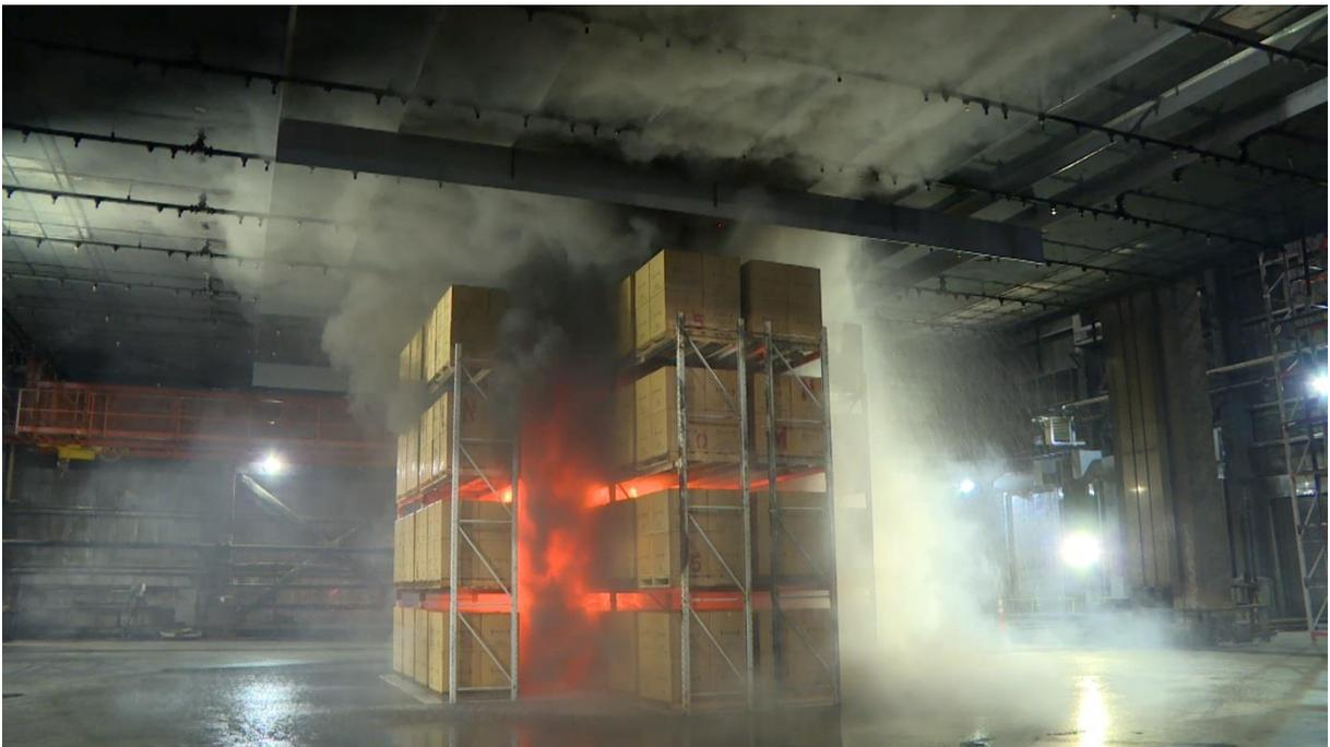
Figure B-4: Test #1 array at 1 min 45 s after ignition.
