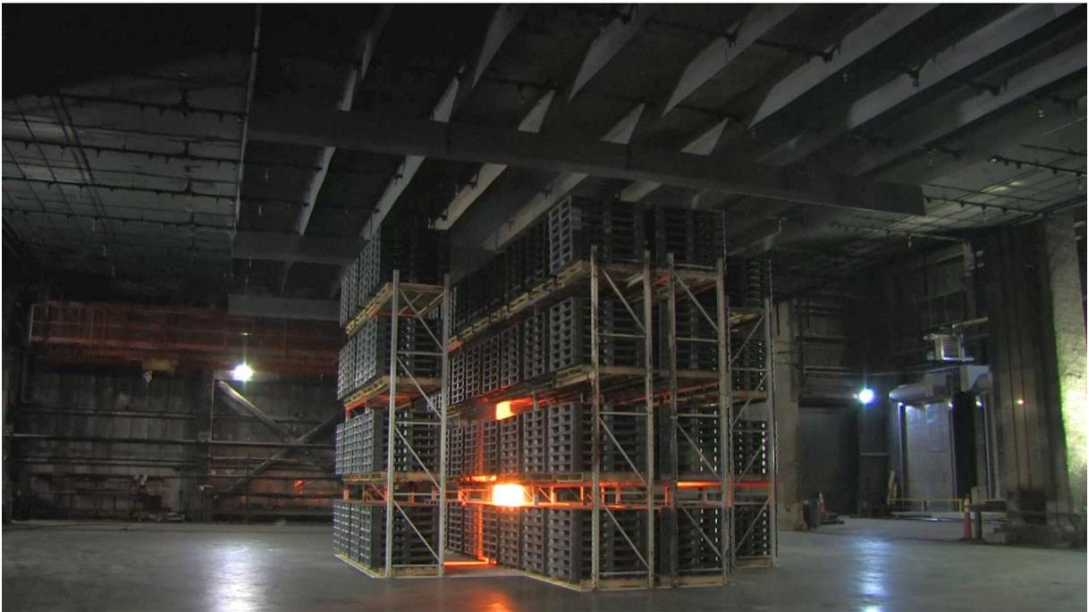
Figure B-16: Test #4 array at 5 min after ignition.
