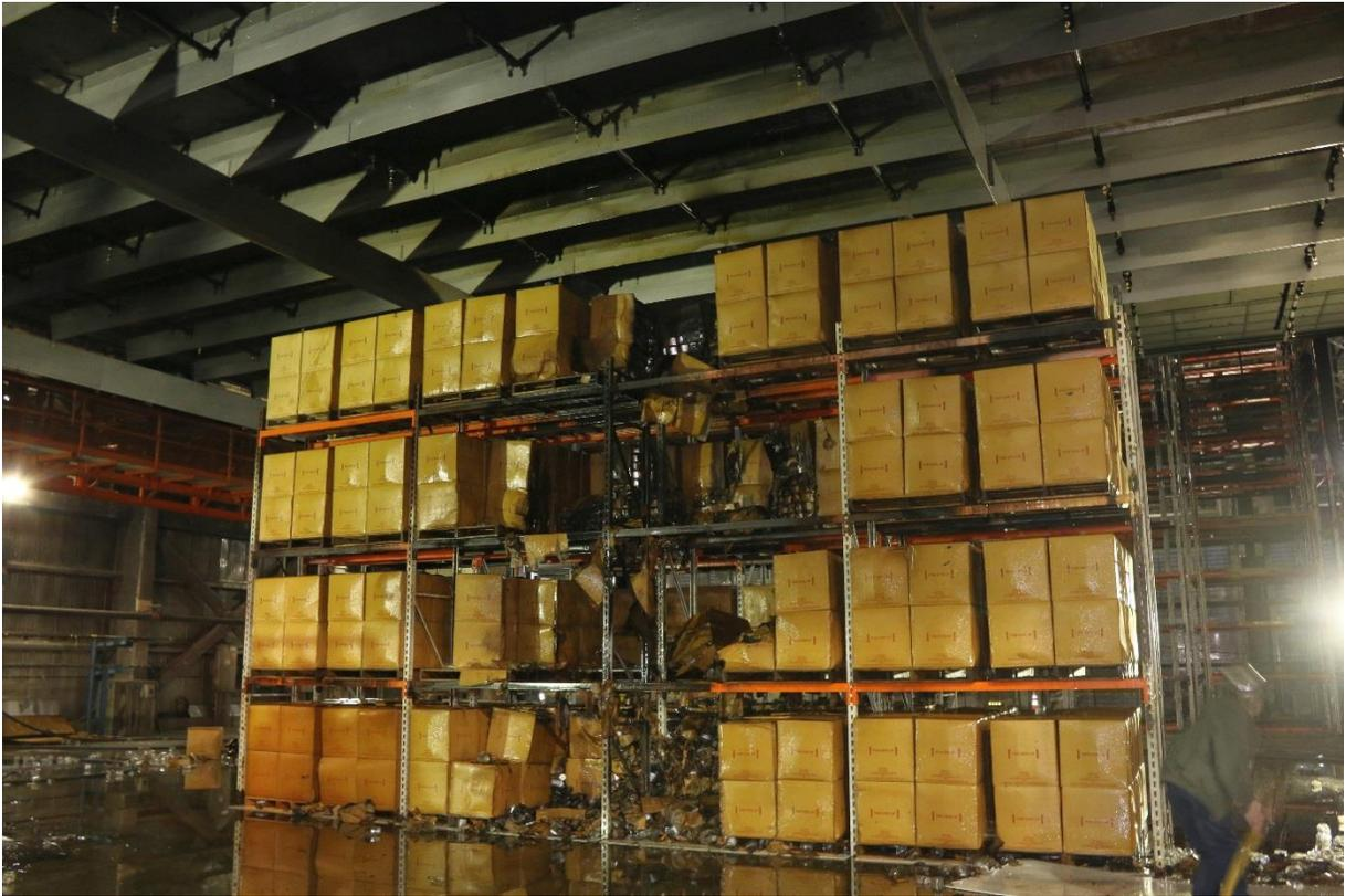
Figure B-15: Test #3 post-test photograph of the east face of the main array showing fire damage.
