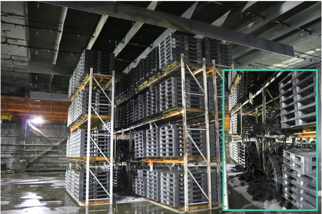
Figure B-20: Test #4 post-test photograph of the east face of the main array showing fire damage. Close-up of the damage area is shown in the inset.
