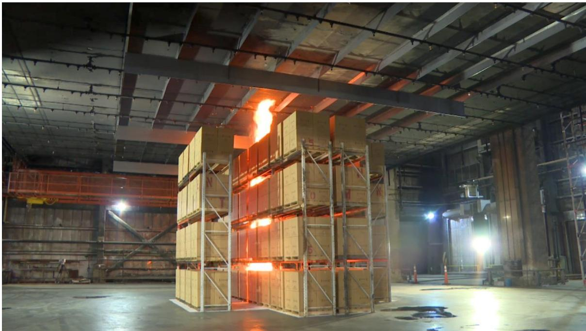
Figure B-1: Test #1 array at 1 min after ignition.
