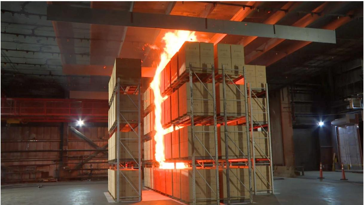
Figure B-8: Test #2 array at 1 min 30 s after ignition.
