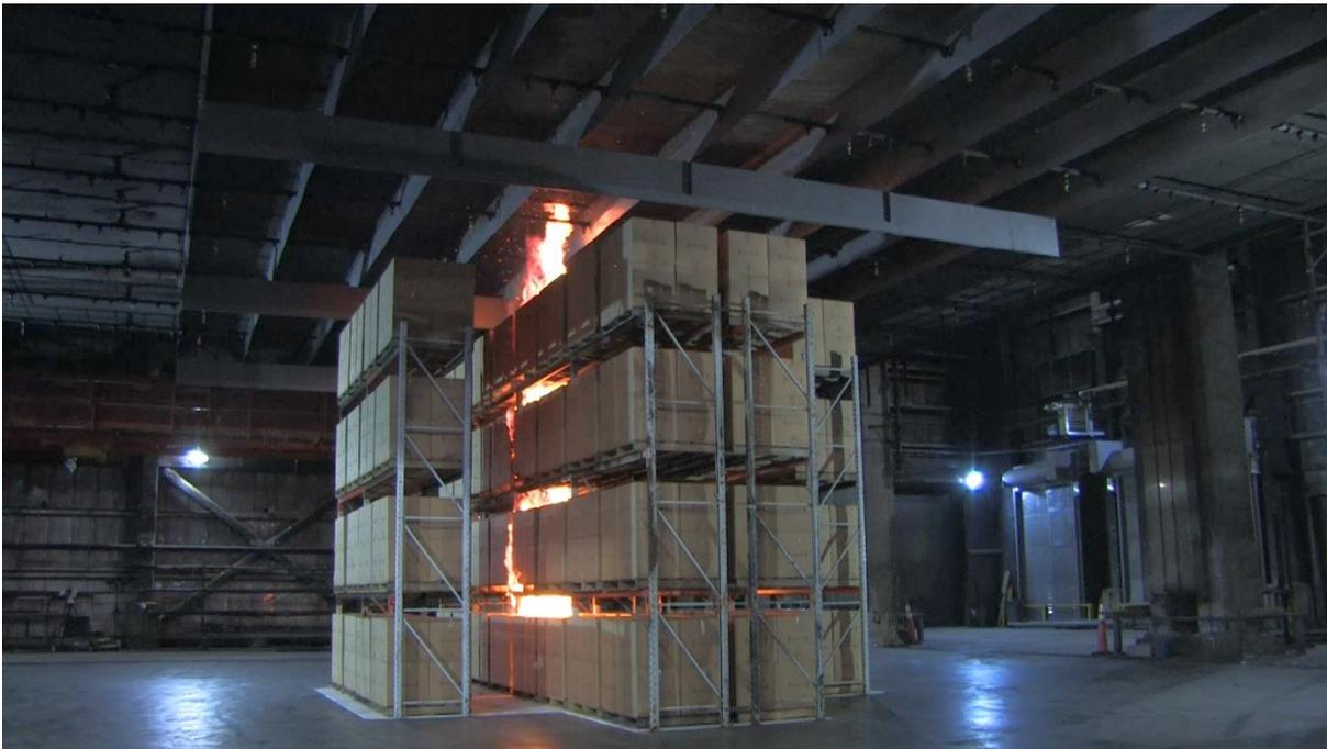
Figure B-11: Test #3 array at 1 min after ignition.
