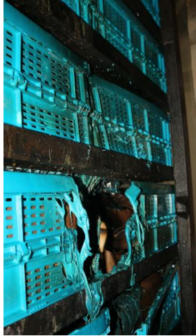
Figure 3-19: Post-test damage at 11% oxygen (a) and 14% oxygen (b) for the vented ML-ASRS with corrugated boxes within the containers.
