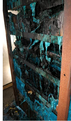
Figure 3-19: Post-test damage at 11% oxygen (a) and 14% oxygen (b) for the vented ML-ASRS with corrugated boxes within the containers.
