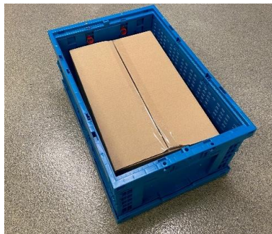
Figure 2-4: Corrugated box placed inside ML-ASRS container to evaluate effects on LOC_{FP} relative to empty containers.
