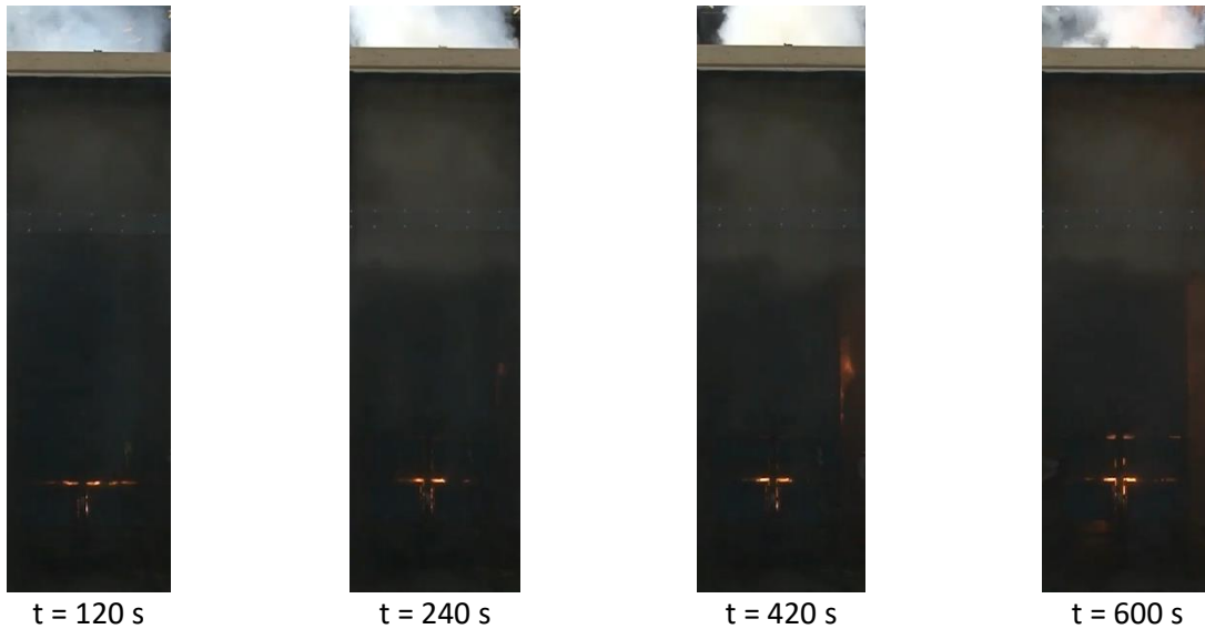
Figure 3-17: Images of fire development for vented ML-ASRS with corrugated contents at 12% O 2 at selected times after ignition.
