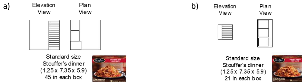
Figure 2-8: Internal packaging of frozen food meals within each a) standard corrugated box and b) wax-saturated box. The empty space in each box was filled with paper cups to prevent movement of the frozen food during setup. (Dimensions in in.)
