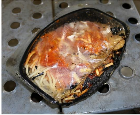
Figure 3-30: Damage to frozen food meal within first tier after the test at 13% oxygen.
