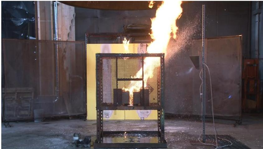
Figure 3-8: Two-carton test photo of non-flammable aqueous base product, 7% hydrocarbon propellant, direct-fill container.
