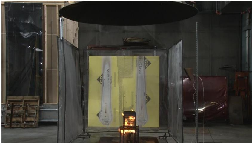
Figure 4-1: Single-can test photo of extra virgin olive oil, non-flammable (HFO1234ze) propellant in a bag-on-valve container.
