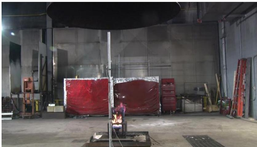
Figure 2-1: Single-can test photo of 50% ethanol base product, non-flammable propellant in a direct fill container.
