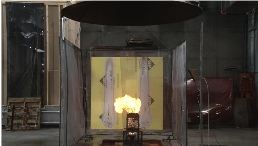
Figure 3-1: Single-can test photo of 100% ethanol base product, non-flammable propellant in a direct-fill container.
