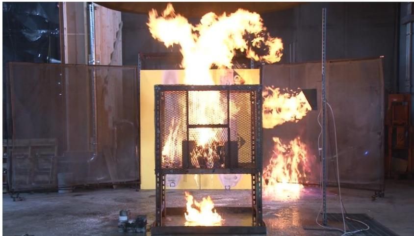
Figure 3-7: Two-carton test photo of 100% ethanol base product, non-flammable (HFO-1234ze) propellant in a bag-on-valve container.
