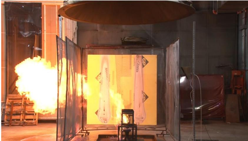
Figure 3-3: Single-can test photo of 100% ethanol base product, non-flammable (HFO-1234ze) propellant in a bag-on-valve container.
