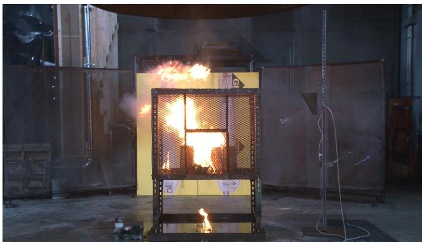
Figure 4-2: Two-carton test photo of extra virgin olive oil, non-flammable (HFO1234ze) propellant in a bag-on-valve container.
