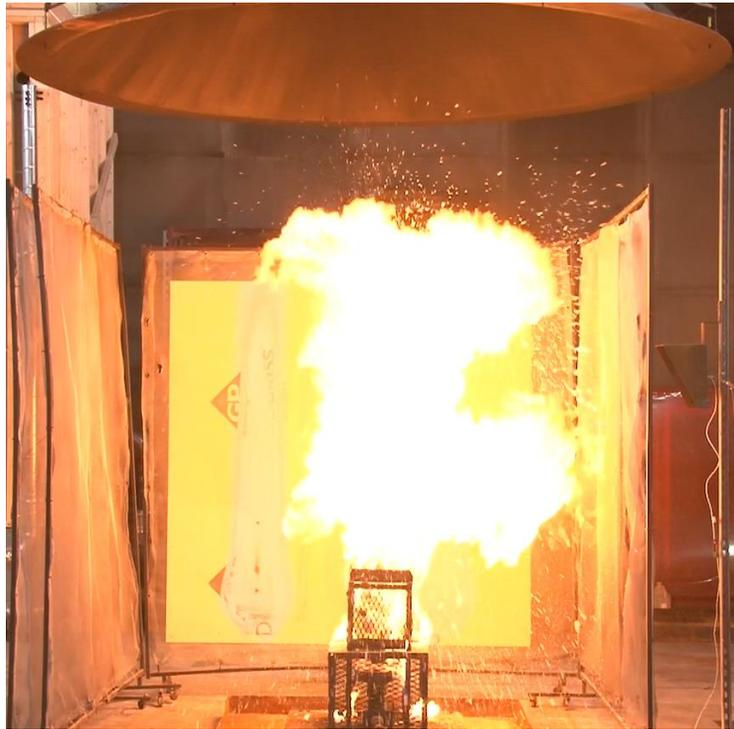
Figure A-3: Photo at time of rupture (13 s) in Test 4.
