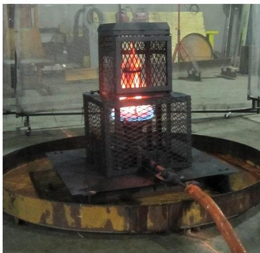
Figure A-1: Photo of the single-can test apparatus.
