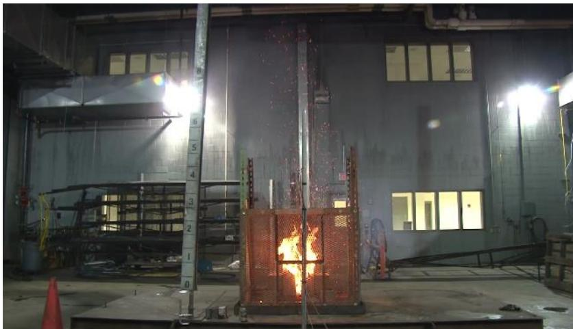
Figure 2-2: Two-carton test photo of 50% ethanol base product, non-flammable propellant in a direct fill container.
