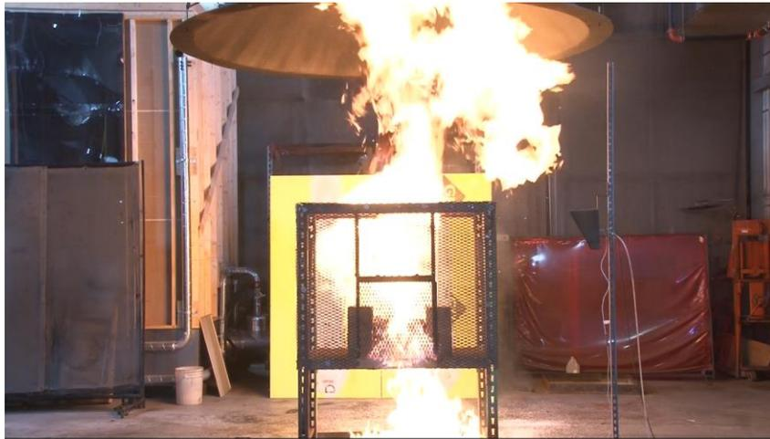
Figure 3-5: Two-carton test photo of 100% ethanol base product, non-flammable propellant in a direct-fill container.
