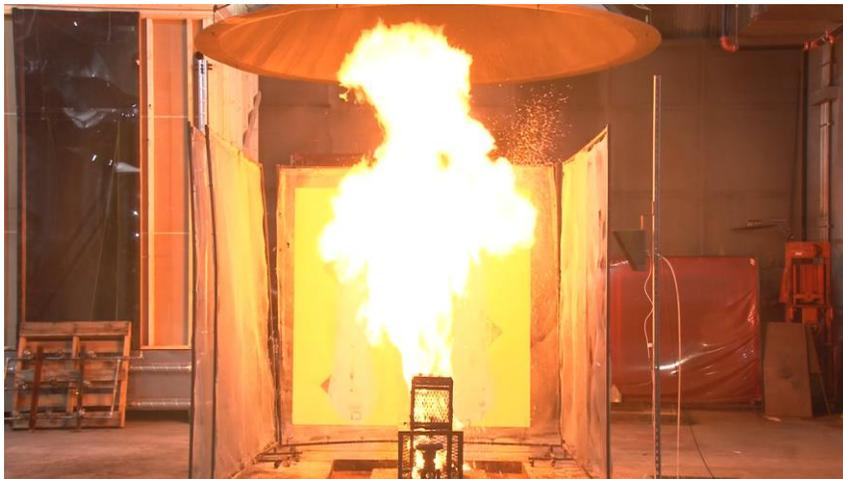
Figure 3-4: Single-can test photo of non-flammable aqueous base product, 7% hydrocarbon propellant, direct-fill container.
