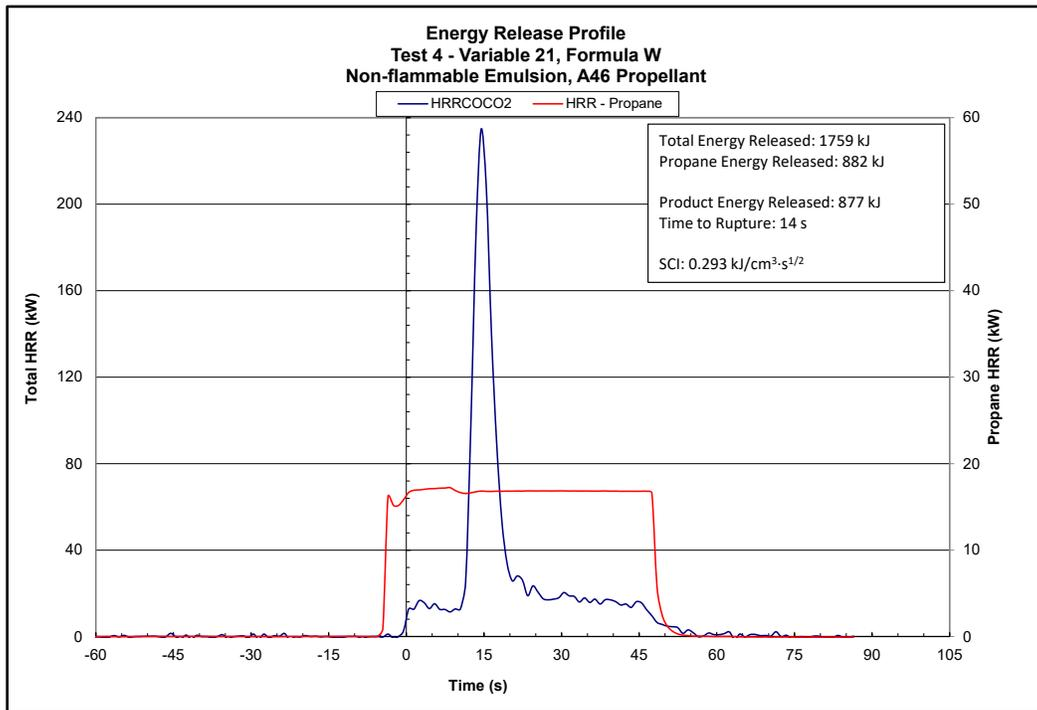
Figure A-4: Energy release profile for Test 4.
