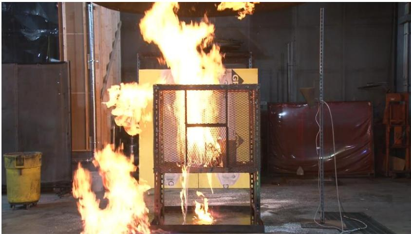
Figure 3-6: Two-carton test photo of 100% ethanol base product, non-flammable (N<sub>2</sub>) propellant in a bag-on-valve container.
