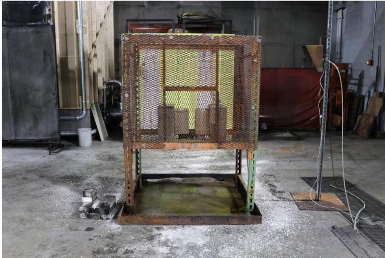
Figure B-2: Photo of two-carton test safety cage.
