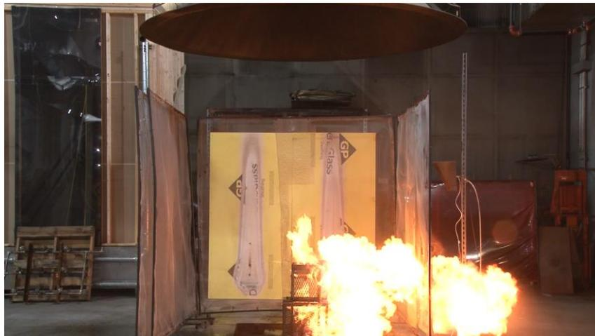
Figure 3-2: Single-can test photo of 100% ethanol base product, non-flammable (N<sub>2</sub>) propellant in a bag-on-valve container.
