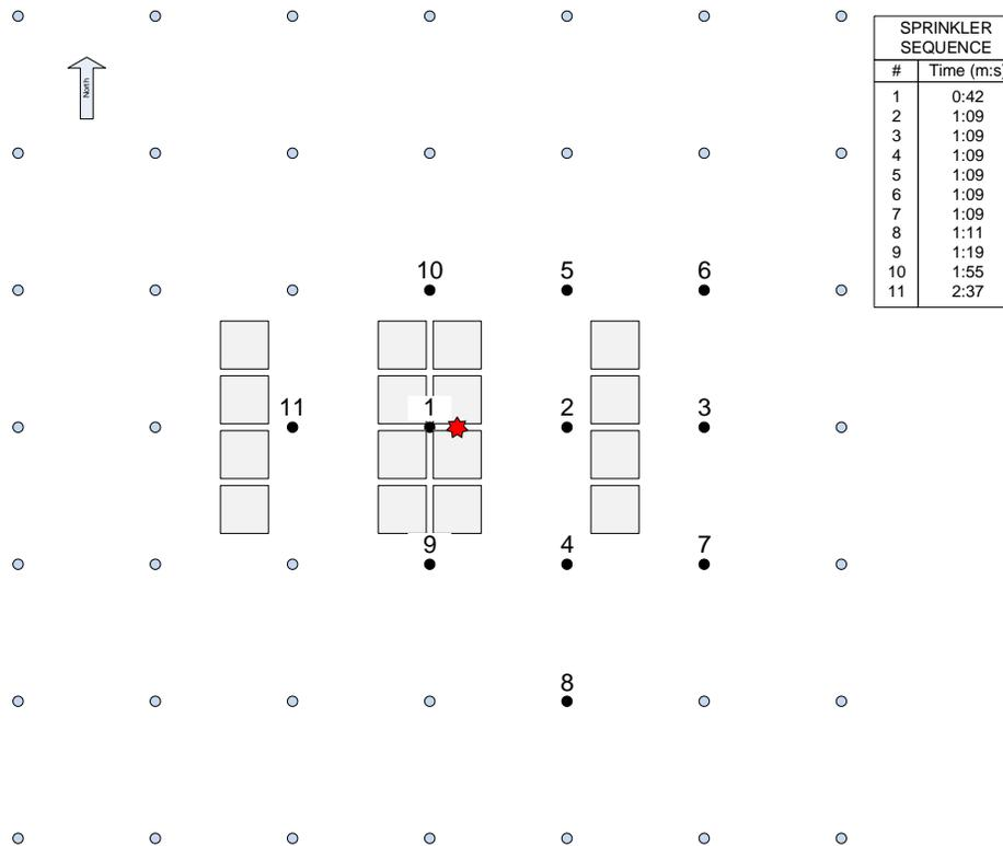
Figure 3.2.2-6: Sprinkler operation pattern – Test 1.
