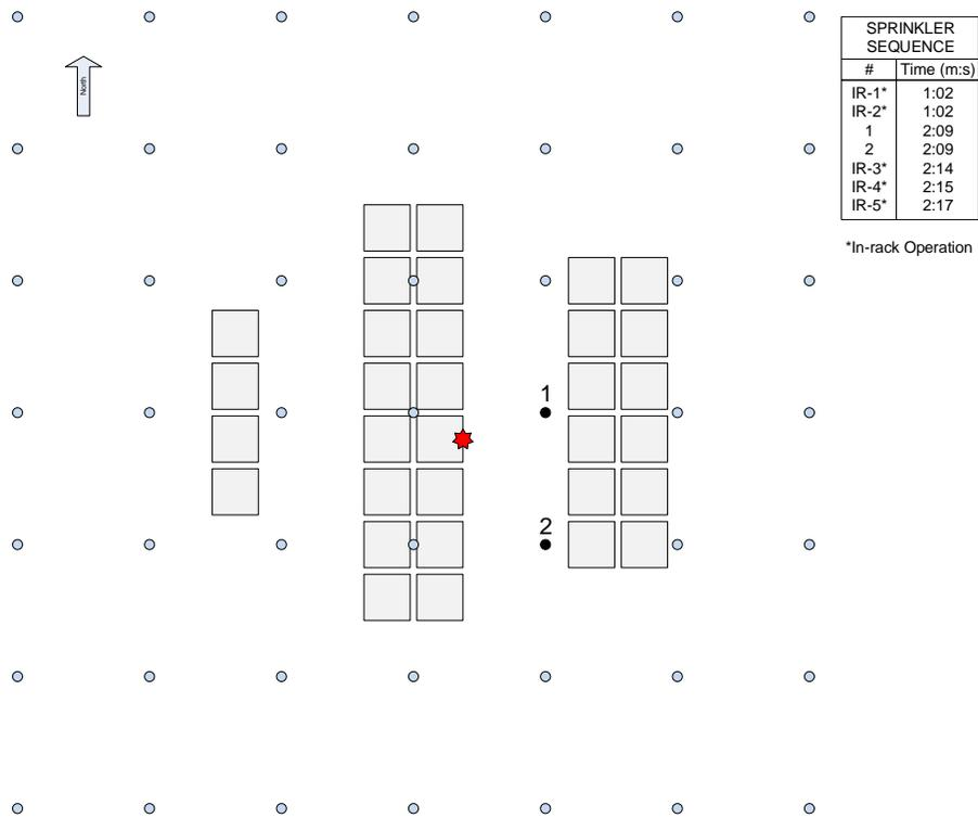
Figure 3.4.2-8: Ceiling sprinkler operation pattern – Test 3.
