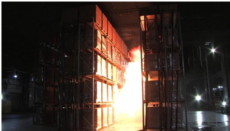
Figure 3.4.2-3: Photo of fire balls generated from plastic aerosol ruptures – Test 3 (2 min 5 s).
