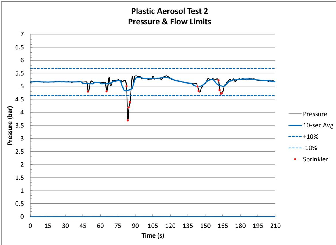
Figure B.2-3: Ceiling sprinkler pressure – Test 2.
