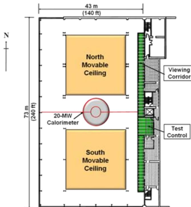
Figure 2.1-1: Illustration of FM Global Large Burn Laboratory test locations
