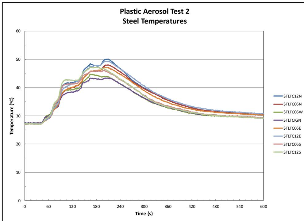
Figure B.2-2: Ceiling steel temperatures – Test 2.
