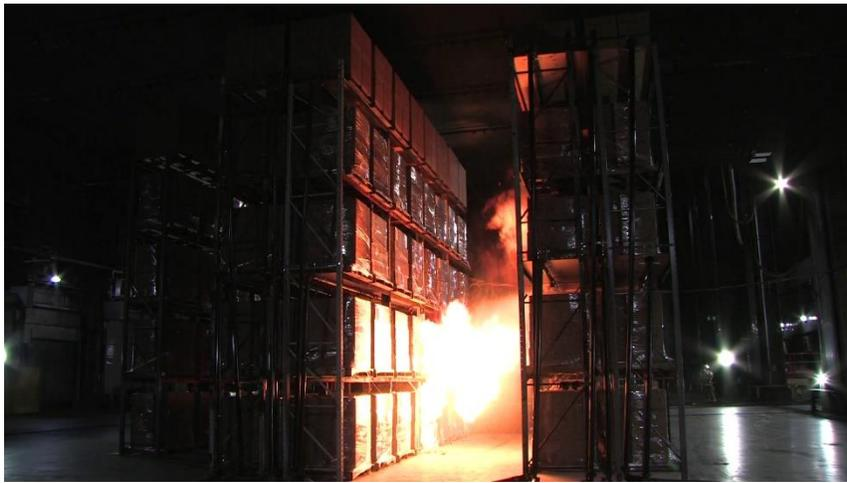
Figure 3.4.2-2: Photo of first in-rack operation – Test 3 (1 min 2 s).
