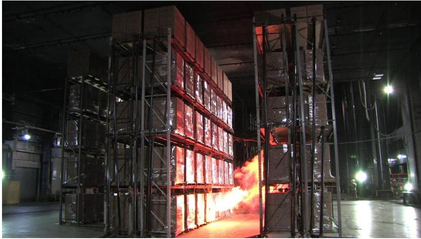
Figure 3.4.2-1: Photo of first aerosol rupture – Test 3 (37 s).
