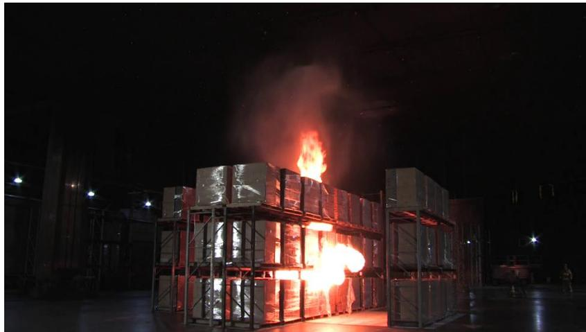
Figure 3.3.2-1: Photo of first sprinkler operation – Test 2 (49 s).
