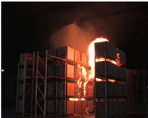
Figure 3.2.2-3: Photo of fire ball from aerosol rupture – Test 1 (1 min 7 s).
