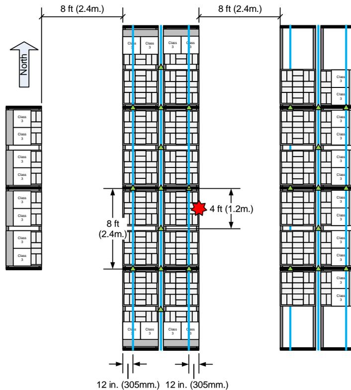
Figure 3.4.1-1: Plan view schematic of the test array – Test 3 (top layer of CUP not indicated).
