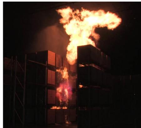
Figure 3.2.2-4: Photo of fire balls reaching ceiling level – Test 1 (1 min 10 s).
