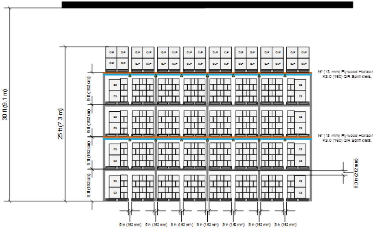
Figure 3.4.1-2: Elevation view schematic of main array – Test 3. Green triangles indicate IRAS location.
