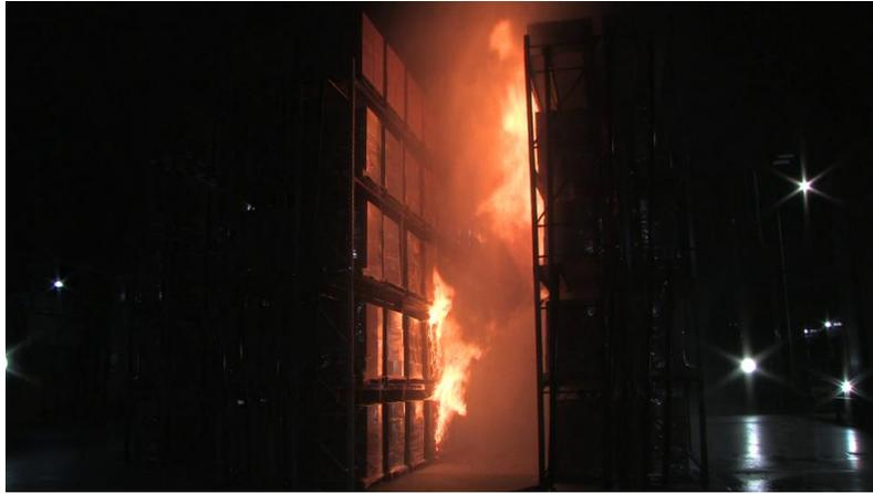
Figure 3.4.2-4: Photo of first ceiling sprinkler operation – Test 3 (2 min 9 s).
