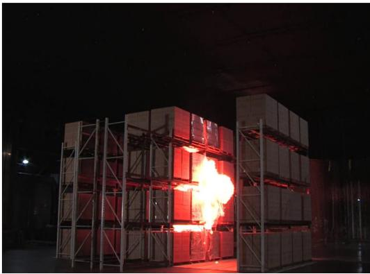
Figure 3.2.2-1: Photo of first rupture – Test 1 (36 s).
