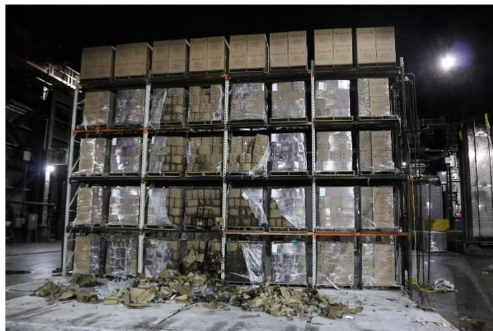
Figure 3.4.2-6: Post-test photo of array – Test 3 (target array removed).
