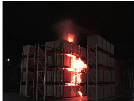
Figure 3.2.2-2: Photo of first sprinkler operation – Test 1 (42 s).
