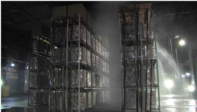
Figure 3.4.2-5: Photo of controlled fire – Test 3 (10 min).
