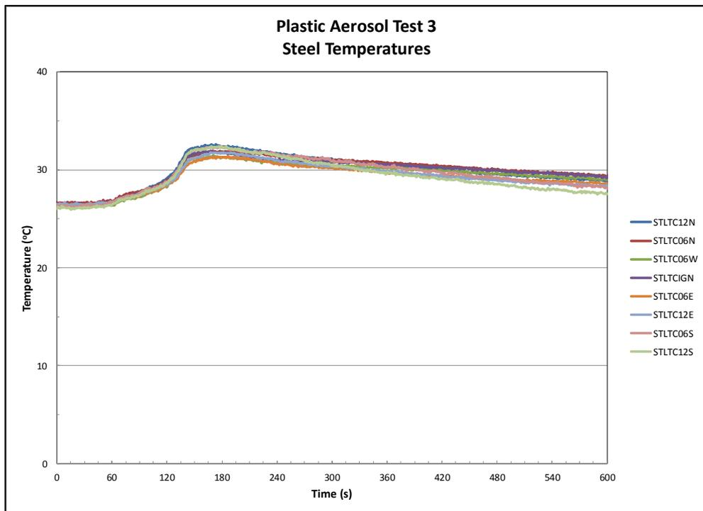
Figure B.3-2: Ceiling steel temperatures – Test 3.
