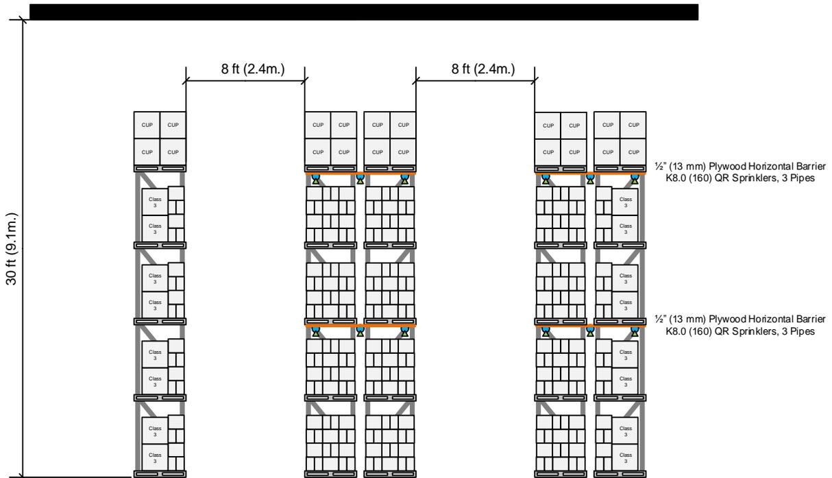
Figure 3.4.1-3: Side elevation view schematic of the test array – Test 3.
