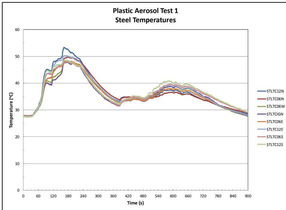
Figure B.1-2: Ceiling steel temperatures – Test 1.
