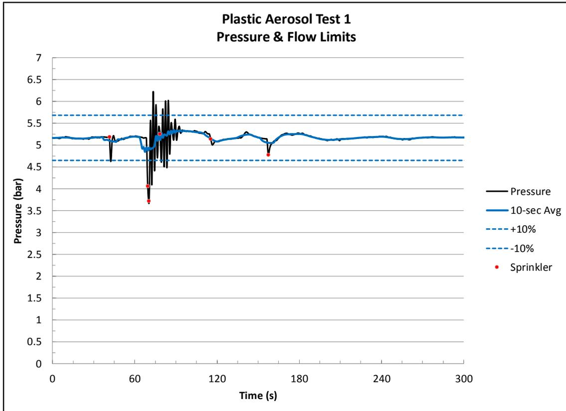
Figure B.1-3: Ceiling sprinkler pressure – Test 1<sup>9</sup>.
