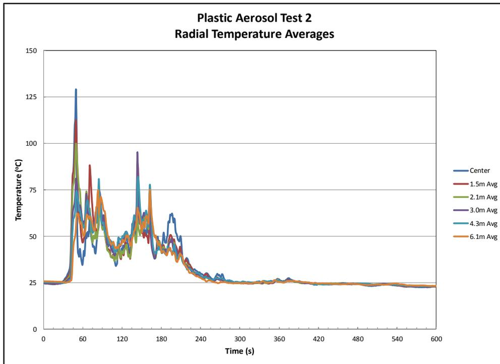
Figure B.2-1: Ceiling radial temperature averages – Test 2.
