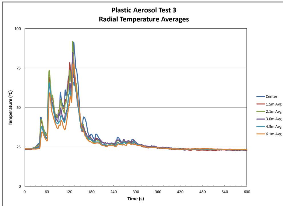
Figure B.3-1: Ceiling radial temperature averages – Test 3.
