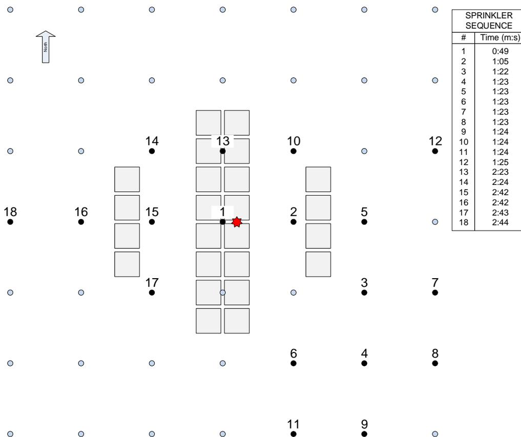
Figure 3.3.2-4: Sprinkler operation pattern – Test 2.
