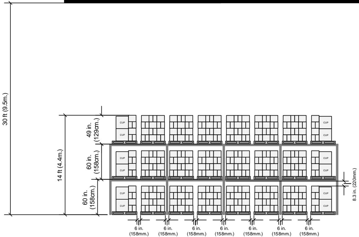
Figure 3.3.1-2: Elevation view schematic of the main array – Test 2.
