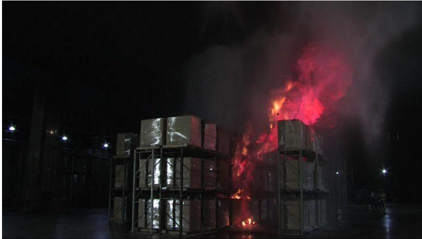
Figure 3.3.2-2: Photo of product involvement – Test 2 (1 min 23 s).
