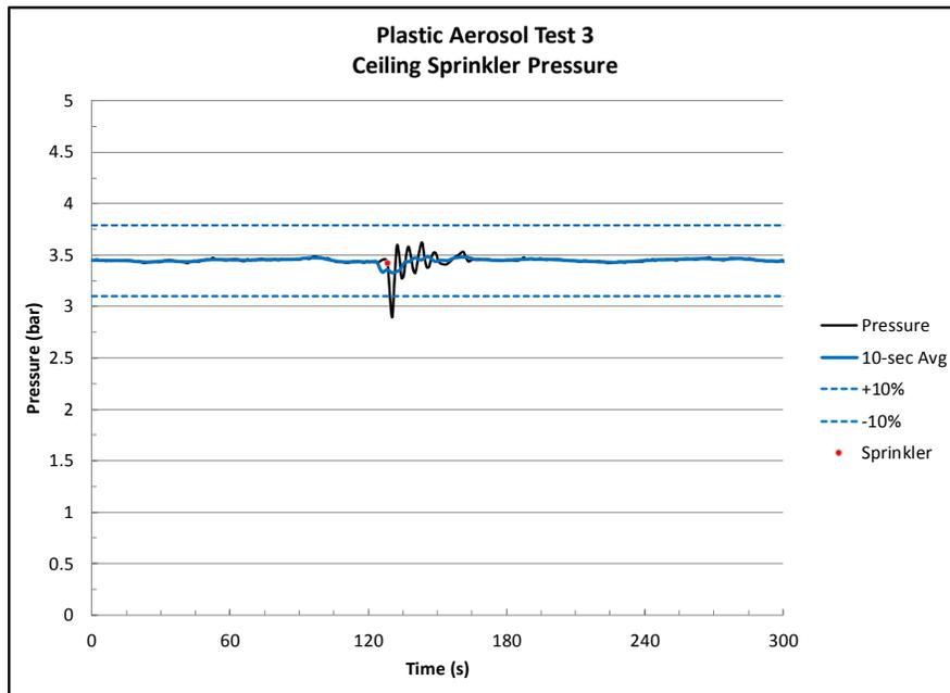
Figure B.4-1: Ceiling Sprinkler Pressure – Test 3.
