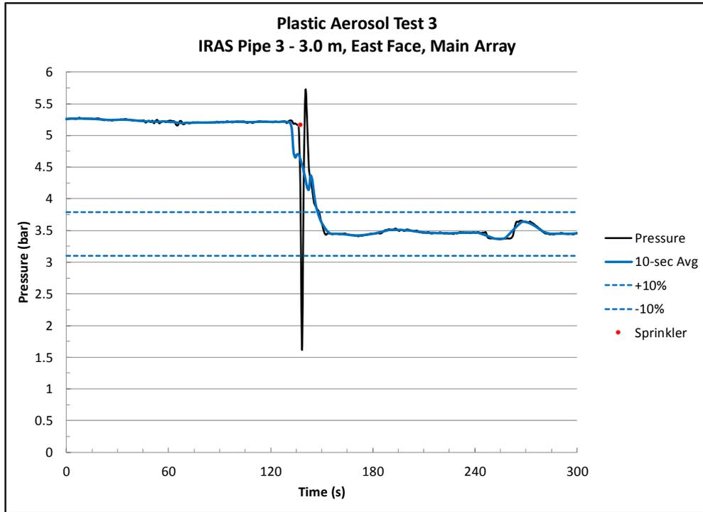
Figure B.4-3: IRAS Pipe 3 Sprinkler Pressure – Test 3.
