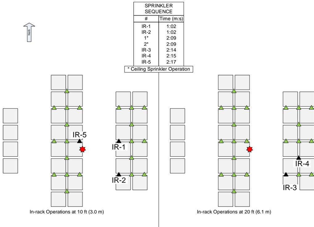
Figure 3.4.2-7: In-rack sprinkler operation pattern – Test 3.
