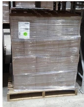
Figure 3.1.2.1-2: Pallet load of cartoned aerosol product.
