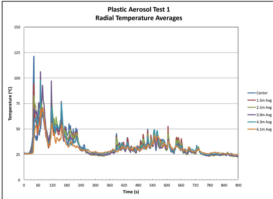
Figure B.1-1: Ceiling radial temperature averages – Test 1.
