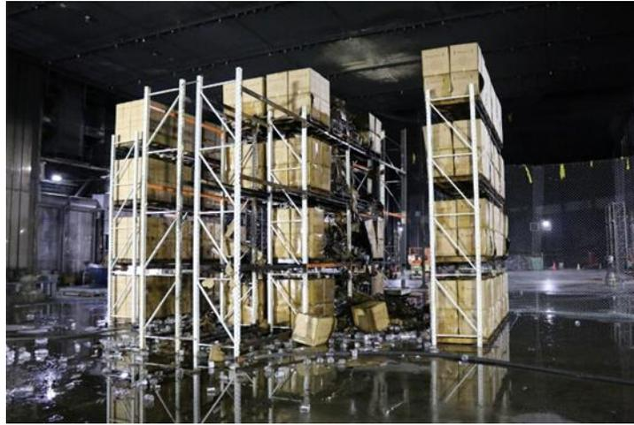
Figure 3.2.2-5: Post-test photo of array – Test 1.
