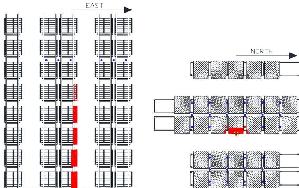
Figure 3.1.3.4.3-2: Test 4 Post Test Damage: (Left) Side Elevation View of Main and Two Target Arrays, (Right) Plan View of Maximum Extent of Damage.
