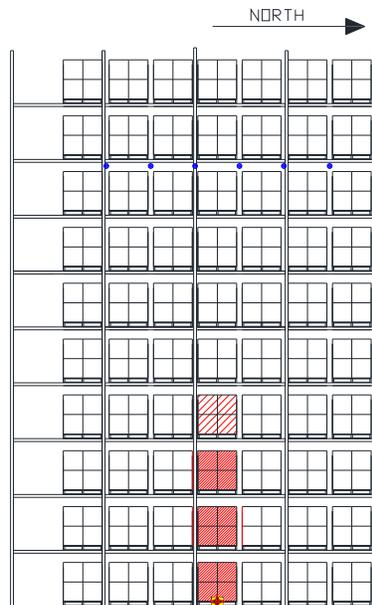
Figure 3.1.3.6.3-1: Test 6 Post Test Damage: Ignition Face of Main Array.
