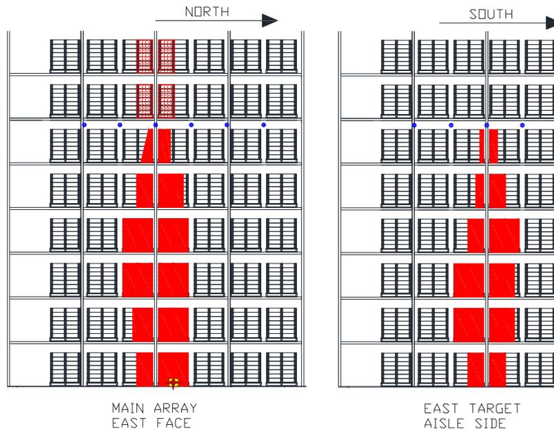
Figure 3.1.3.3.3-1: Test3 Post Test Damage: (Left) Ignition Face of Main Array, (Right) Target Facing Ignition.
