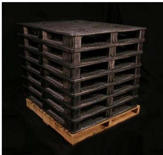
Figure 3.2.2.2-1: FM Global Standard Uncartoned Unexpanded Plastic (UUP) Commodity.
