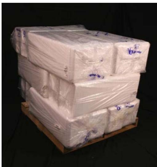
Figure 3.1.2.2.1-1: FM Global Standard Uncartoned Expanded Plastic (UEP) Commodity.
