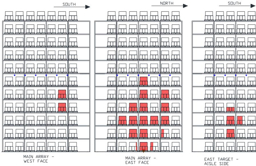
Figure 3.1.3.1.3-1: Test 1 Post Test Damage: (Left) West Face of Main Array, (Center) Ignition Face of Main Array, (Right) Target Facing Ignition.
