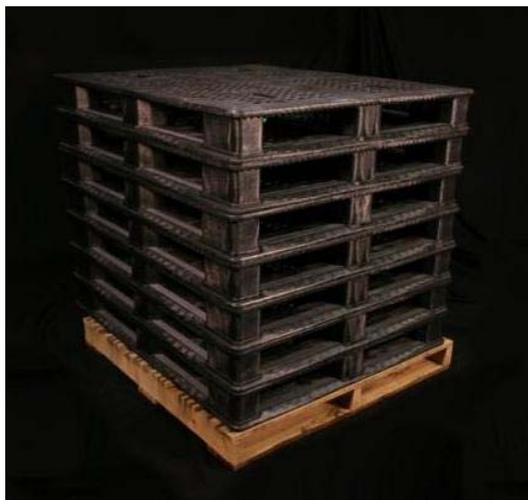
Figure 3.1.2.2.3-1: FM Global Standard Uncartoned Unexpanded Plastic (UUP) Commodity.
