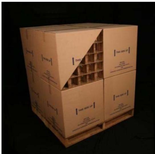
Figure 3.1.2.2.2-9: FM Global Standard Cartoned Unexpanded Plastic (CUP) Commodity.
