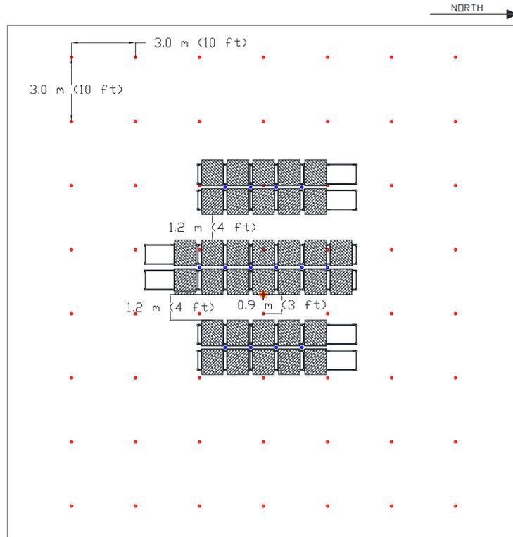
Figure 2.3.3-1: Test 7 ignition location relative to ceiling level sprinklers.
