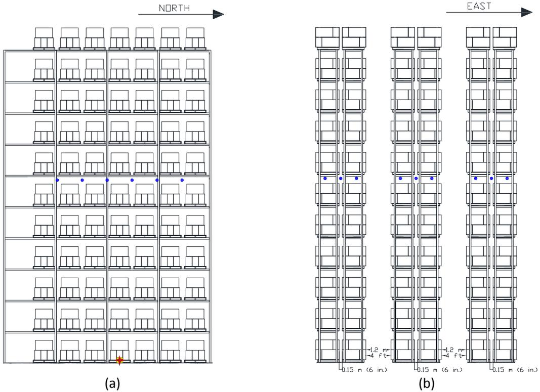
Figure 3.1.2.1-1: Test 1 Rack Storage Configuration, (a) Front Elevation View of East Side of Main Array, (b) Side Elevation View of Main and Two Target Arrays.
