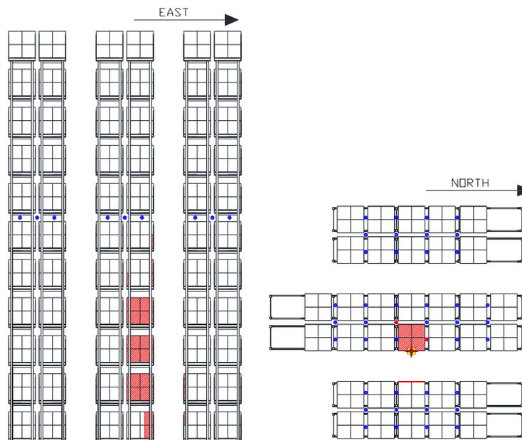
Figure 3.1.3.2.3-2: Test 2 Post Test Damage: (Left) Side Elevation View of Main and Two Target Arrays, (Right) Plan View of Maximum Extent of Damage.
