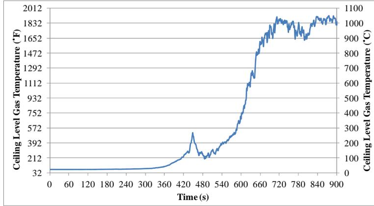
Figure 3.2.3.1.2-3: Test 7 ceiling level gas temperature.
