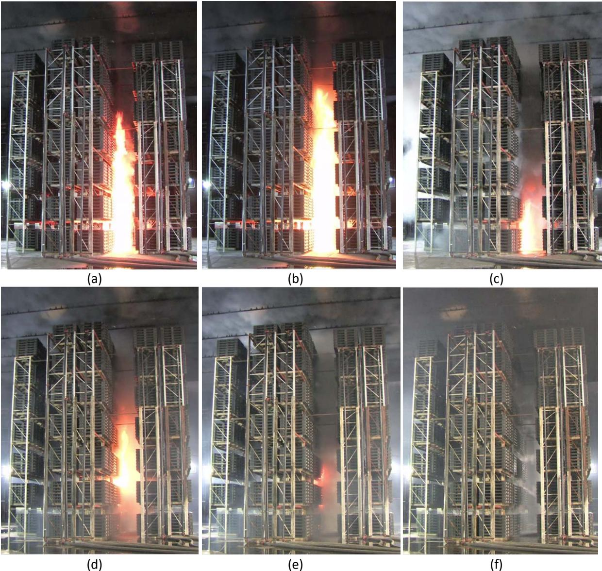
Figure 3.2.3.2.1-1: Test 9 images: (a) 06:42, time of 1<sup>st</sup> IRAS activation, (b) 07:05, time of 3<sup>rd</sup> IRAS activation, (c) 07:50, reduced fire severity, 45 seconds after 3<sup>rd</sup> IRAS activation (d) 15:22, time of 4<sup>th</sup> and final IRAS activation, (e) 15:40, fire severity decreased, (f) 20:00, fire is suppressed.
