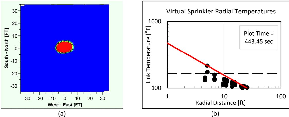
Figure 3.2.3.2.2-2: Estimation of extent of ceiling level sprinkler activations for  $74^\circ\text{C}$  ( $165^\circ\text{F}$ ) standard-response sprinklers for the time step which yielded the maximum radius (a) Temperature contour plot showing region of potential activations (red region), (b) Log-log plot of sprinkler link temperature as a function of radial distance from ceiling center.
