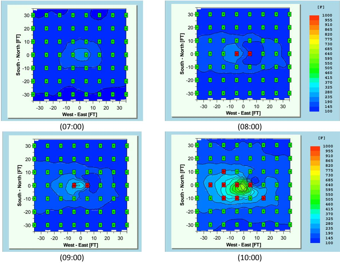
Figure 3.2.3.1.2-1: Test 7 ceiling level gas temperature contours: 07:00 through 10:00.
