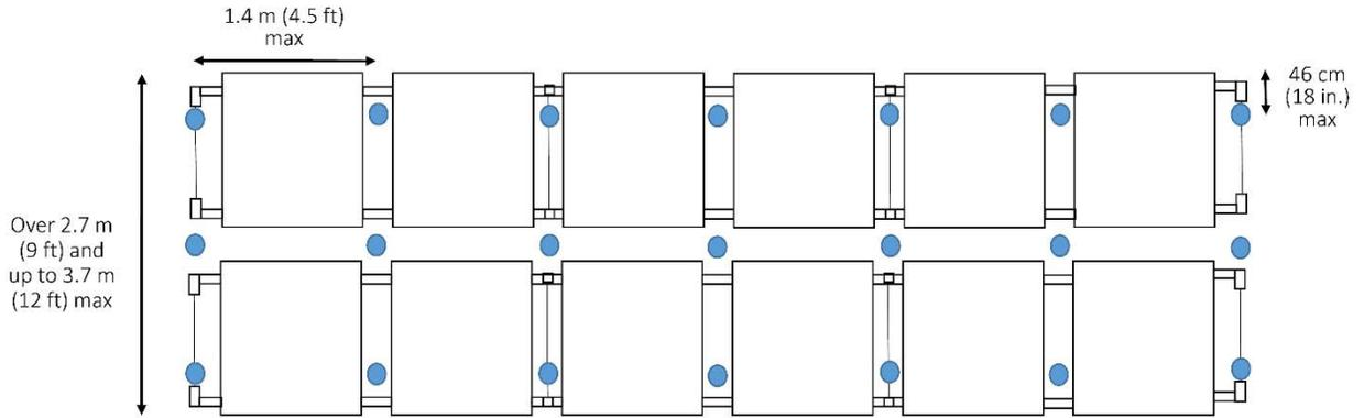
Figure 5.1-5: IRAS arrangement for open-frame, double-row racks over 2.7 m (9 ft) and up to 3.7 m (12 ft) deep.
