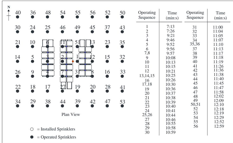
Figure 3.2.3.1.1-2: Test 7 ceiling level sprinkler activation location and sequence of operation.
