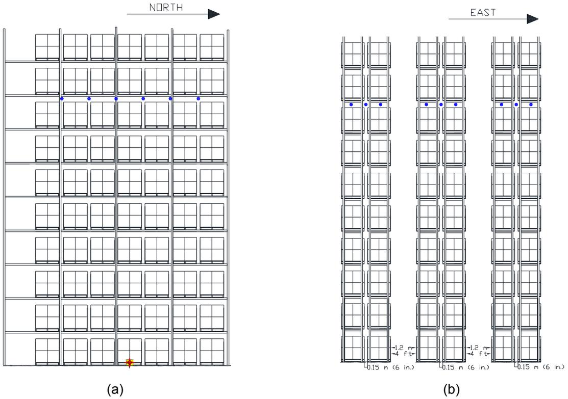
Figure 3.1.2.1-7: Test 6 Rack Storage Configuration, (a) Front Elevation View of East Side of Main Array, (b) Side Elevation View of Main and Two Target Arrays.
