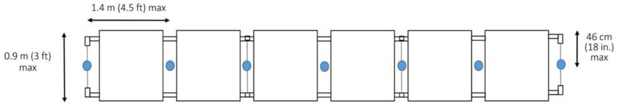
Figure 5.1-1: IRAS arrangement for open-frame, single-row racks up to 0.9 m (3 ft) deep.
