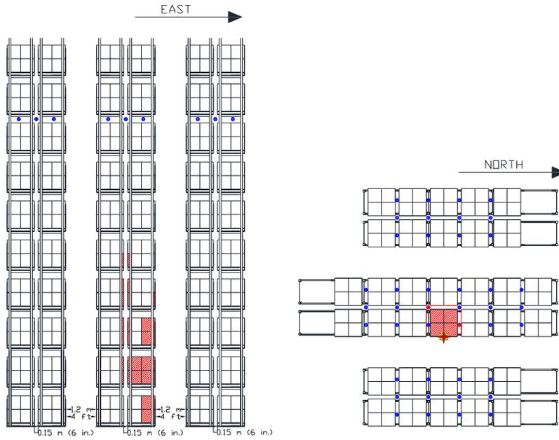
Figure 3.1.3.6.3-2: Test 6 Post Test Damage: (Left) Side Elevation View of Main and Two Target Arrays, (Right) Plan View of Maximum Extent of Damage.
