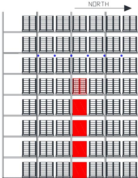
Figure 3.1.3.4.3-1: Test 4 Post Test Damage: Ignition Face of Main Array.
