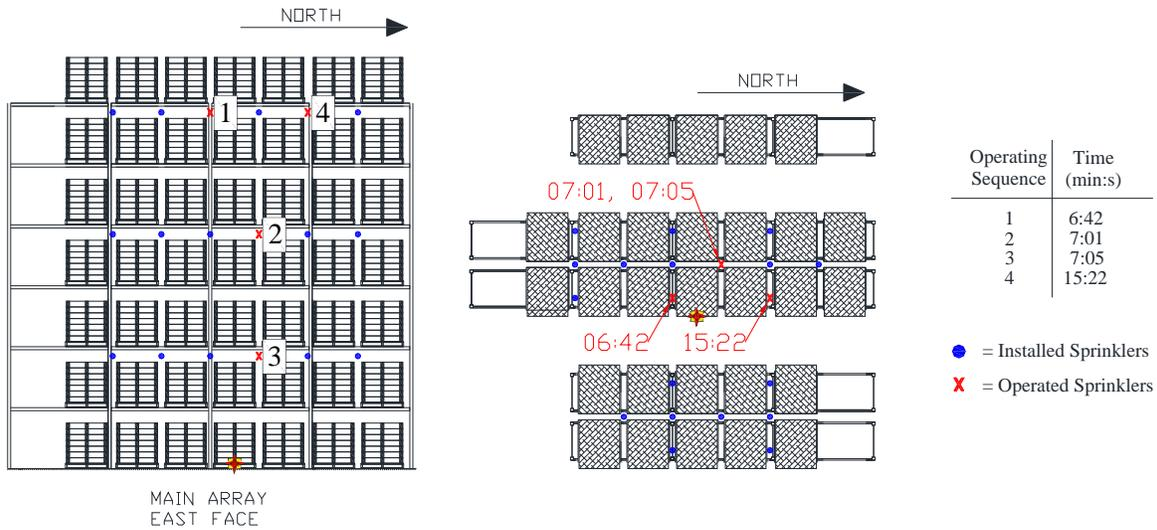
Figure 3.2.3.2.1-2: Test 9 in-rack sprinkler activation location and sequence of operation.
