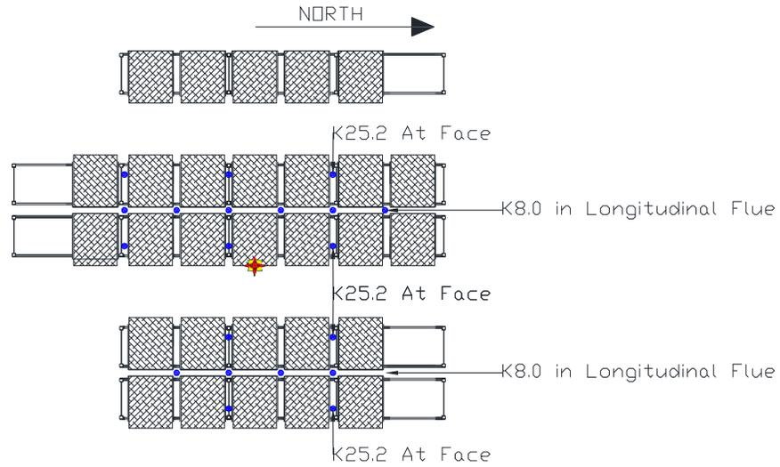
Figure 3.2.2.1-3: Test 9 plan view of main and target arrays separated by 1.2 m (4 ft) aisles.
