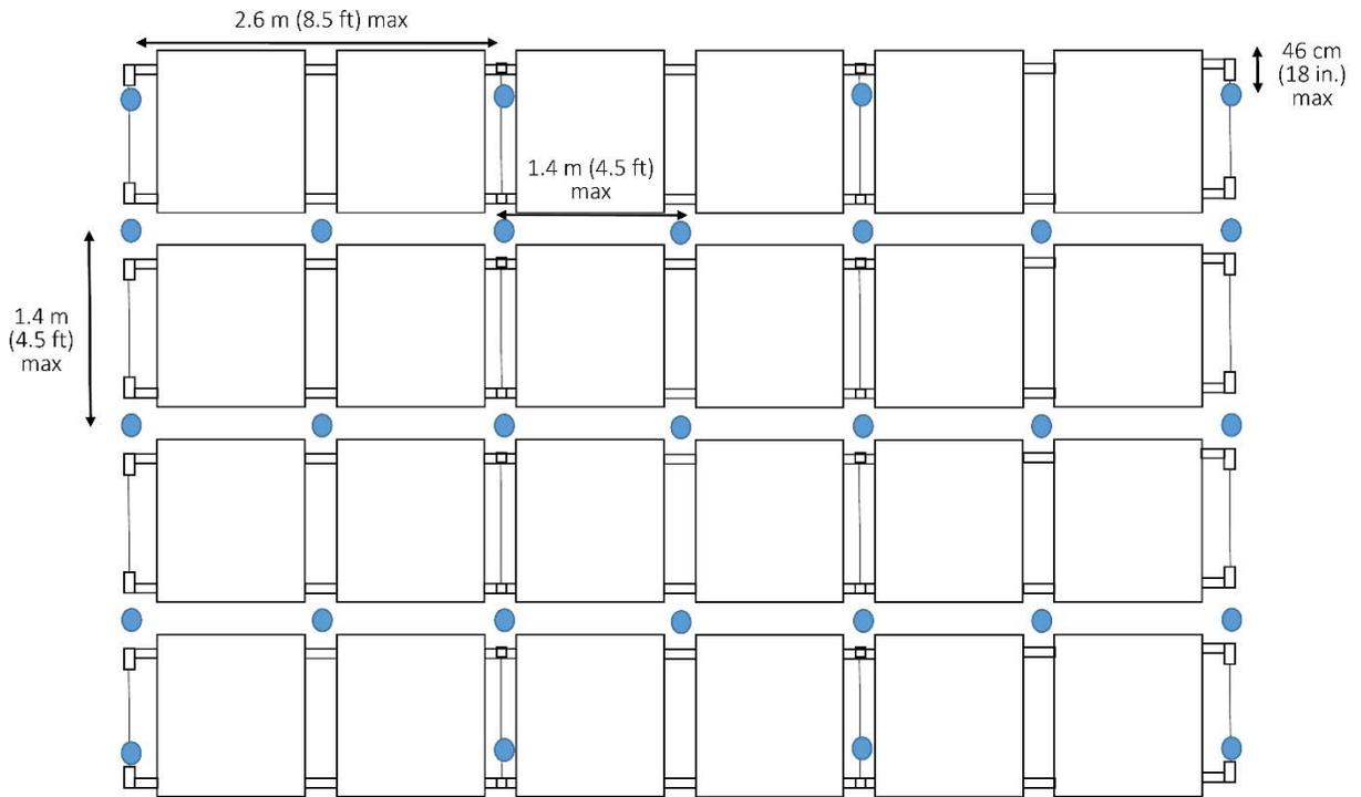
Figure 5.1-6: IRAS arrangement for open-frame, multiple-row racks.
