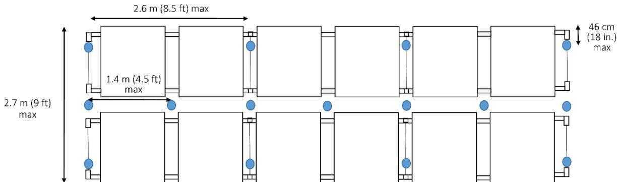
Figure 5.1-4: IRAS arrangement for open-frame, double-row racks up to 2.7 m (9 ft) deep.
