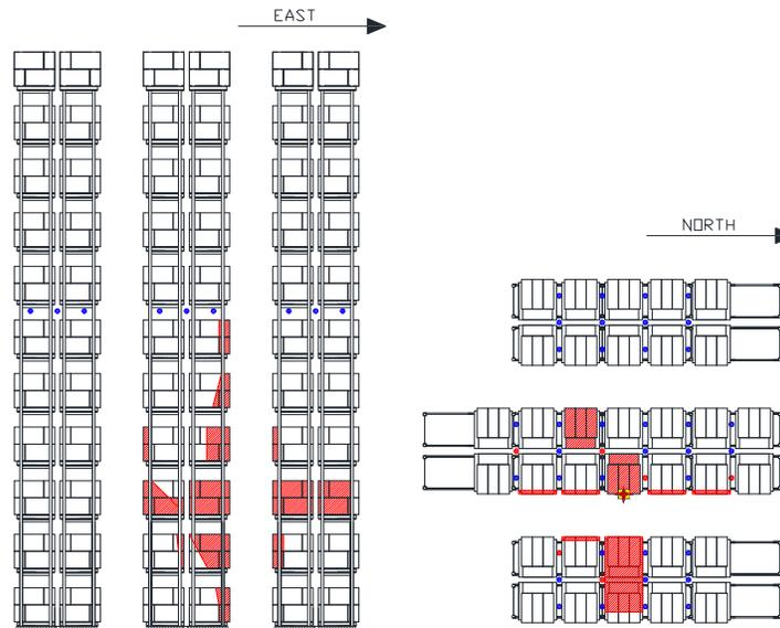
Figure 3.1.3.1.3-2: Test 1 Post Test Damage: (Left) Side Elevation View of Main and Two Target Arrays, (Right) Plan View of Maximum Extent of Damage.
