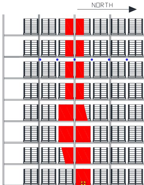
Figure 3.1.3.5.3-1: Test 5 Post Test Damage: Ignition Face of Main Array.
