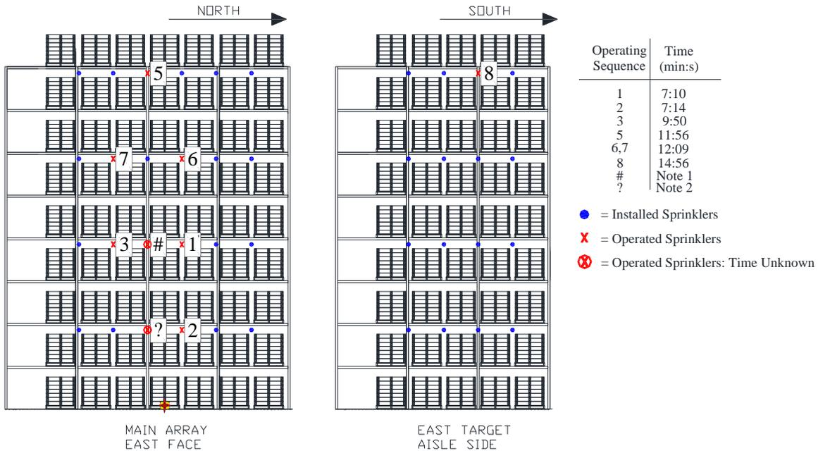
**Note 1:** Post test inspection revealed that this sprinkler had activated; however, its activation did not report to the data acquisition system. Based on the pressure in the pipe, it is believed that this sprinkler activated simultaneously with either the first (07:10) or third (09:50) IRAS activation bringing the total number of in-rack activations to four.
