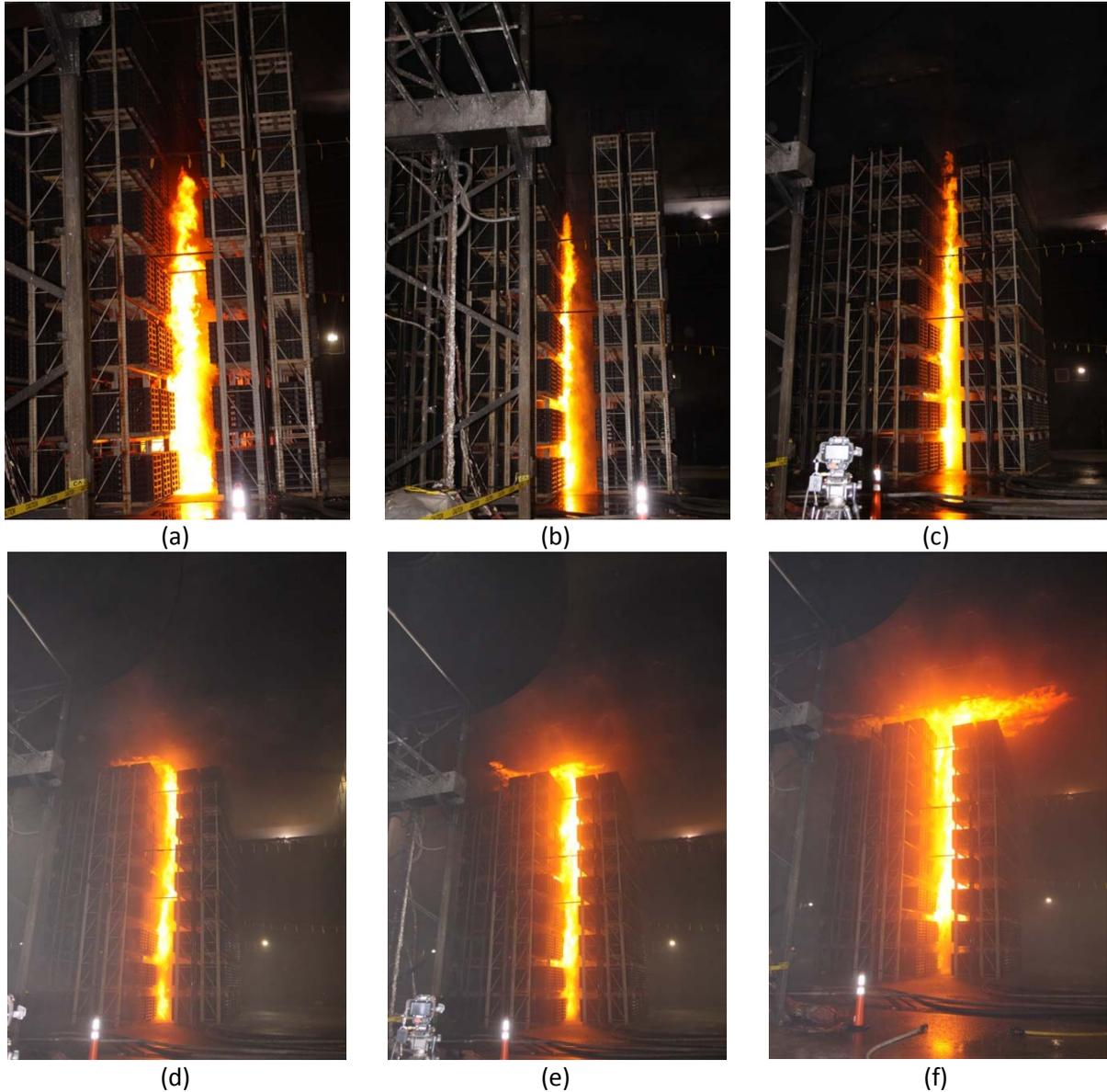
Figure 3.2.3.1.1-1: Test 7 images of fire test: (a) 07:18, eight and five seconds after the 1<sup>st</sup> IRAS and 1<sup>st</sup> ceiling level sprinkler activation, respectively, (b) 09:18, flames reach top of main array, (c) 10:13, 10 ceiling sprinklers active, (d) 11:32, 41 ceiling sprinklers active, (e) 12:10, east target ignites, (f) 14:18, state of fire prior to test termination. [Note: different view angles and scale]
