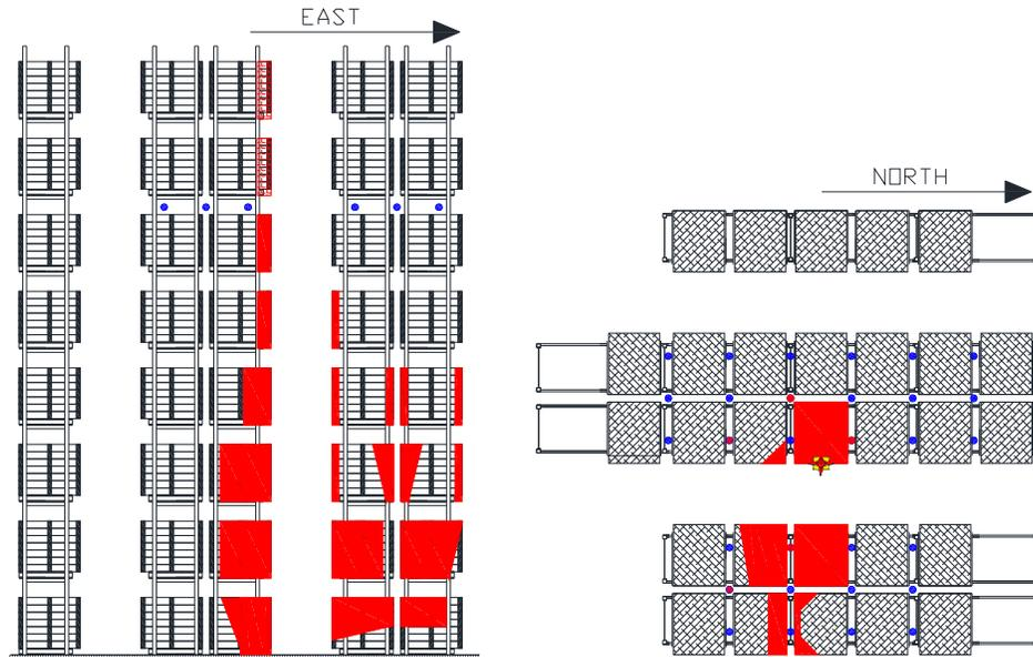
Figure 3.1.3.3.3-2: Test 3 Post Test Damage: (Left) Side Elevation View of Main and Two Target Arrays, (Right) Plan View of Maximum Extent of Damage.
