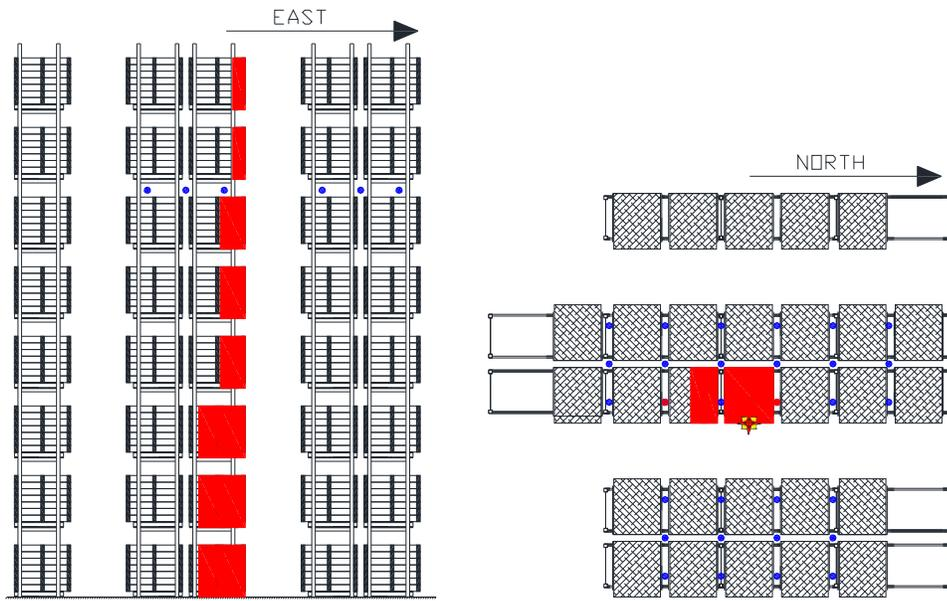
Figure 3.1.3.5.3-2: Test 5 Post Test Damage: (Left) Side Elevation View of Main and Two Target Arrays, (Right) Plan View of Maximum Extent of Damage.
