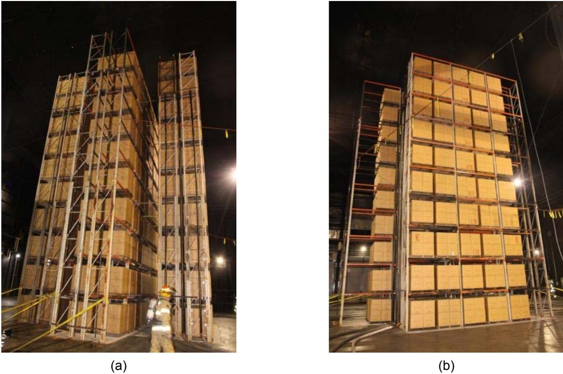
Figure 3.1.2.1-8: Test 6 Pre-Test Images of Arrays, (a) Front Elevation View of East Target Array, (b) Side Elevation View of Main and Two Target Arrays.
