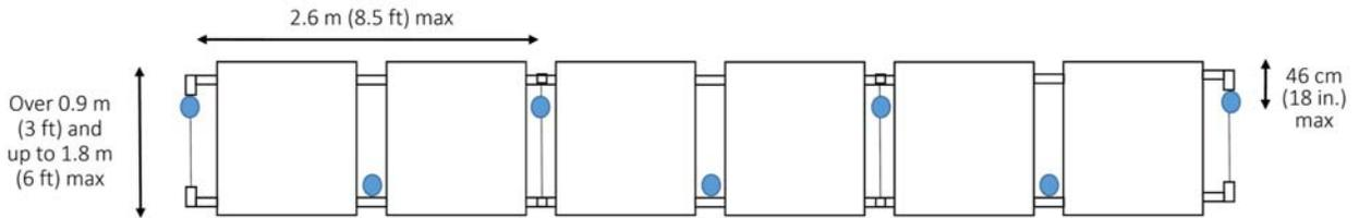
Figure 5.1-2: IRAS arrangement for open-frame, single-row racks over 0.9 m (3 ft) and up to 1.8 m (6 ft) deep.
