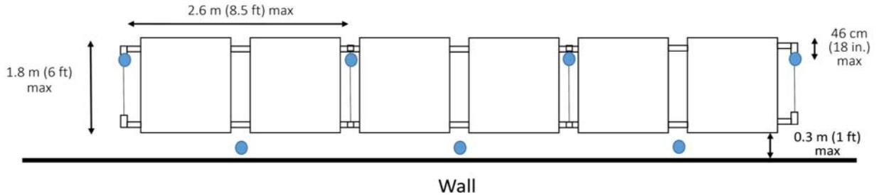
Figure 5.1-3: IRAS arrangement for open-frame, single-row racks over 0.9 m (3 ft) and up to 1.8 m (6 ft) deep located within 0.3 m (1 ft) of a wall.
