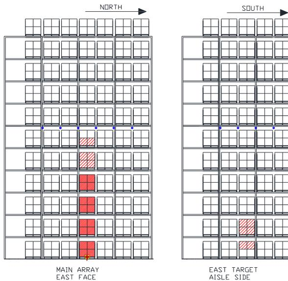
Figure 3.1.3.2.3-1: Test 2 Post Test Damage: (Left) Ignition Face of Main Array, (Right) Target Facing Ignition.
