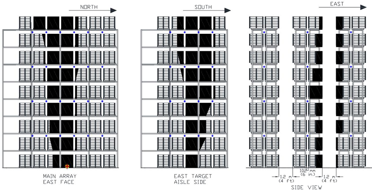
Figure 3.2.3.1.3-1: Test 7 fire damage to main and east target array.
