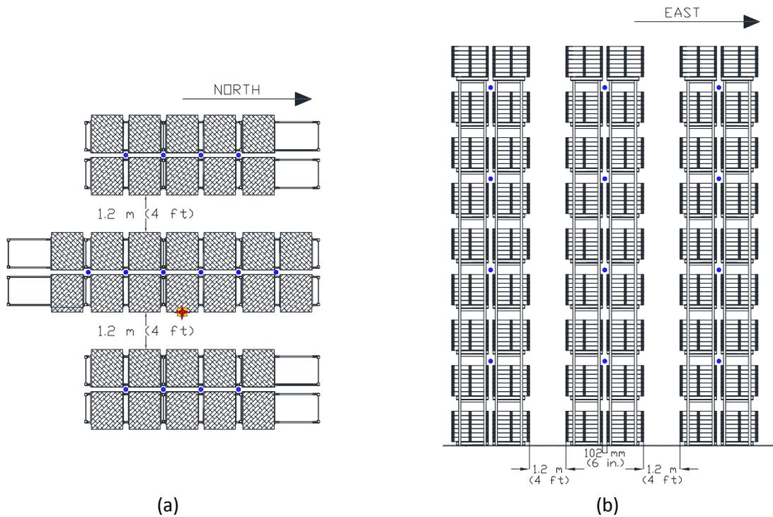
Figure 3.2.2.1-1: (a) Test 7 (a) plan view of main and target arrays IRAS, (1.2 m [4 ft] horizontal spacing) shown within longitudinal flue, (b) side elevation view of main and target arrays separated by 1.2 m (4 ft) aisles. IRAS, (3.0 m [10 ft] vertical spacing), shown within longitudinal flue.
