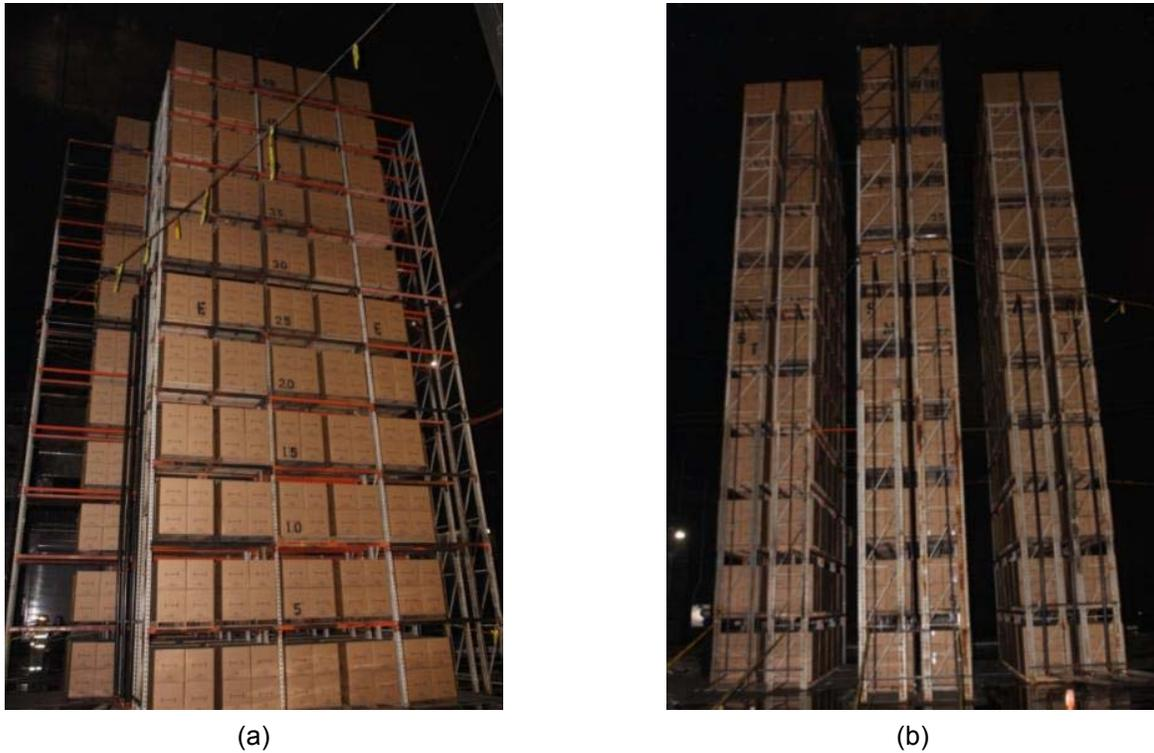
Figure 3.1.2.1-4: Test 2 Pre-Test Images of Arrays, (a) Front Elevation View of East Target Array, (b) Side Elevation View of Main and Two Target Arrays.
