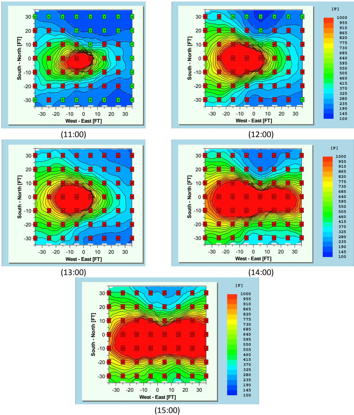
Figure 3.2.3.1.2-2: Test 7 ceiling level gas temperature contours: 11:00 through 15:00 test termination.
