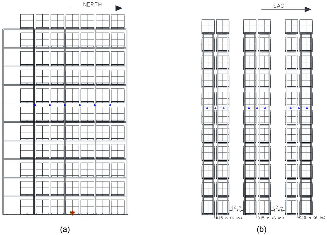
Figure 3.1.2.1-3: Test 2 Rack Storage Configuration, (a) Front Elevation View of East Side of Main Array, (b) Side Elevation View of Main and Two Target Arrays.
