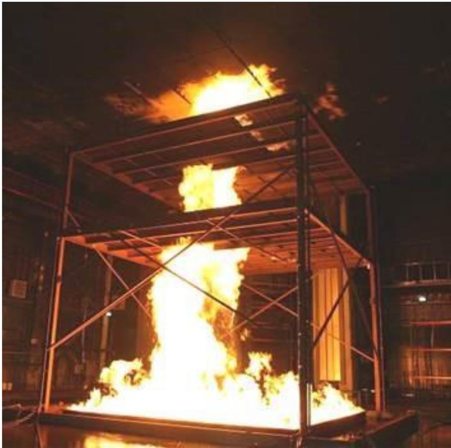
Figure 1-1: Ethanol pool fire underneath a two-level grated mezzanine [1].
