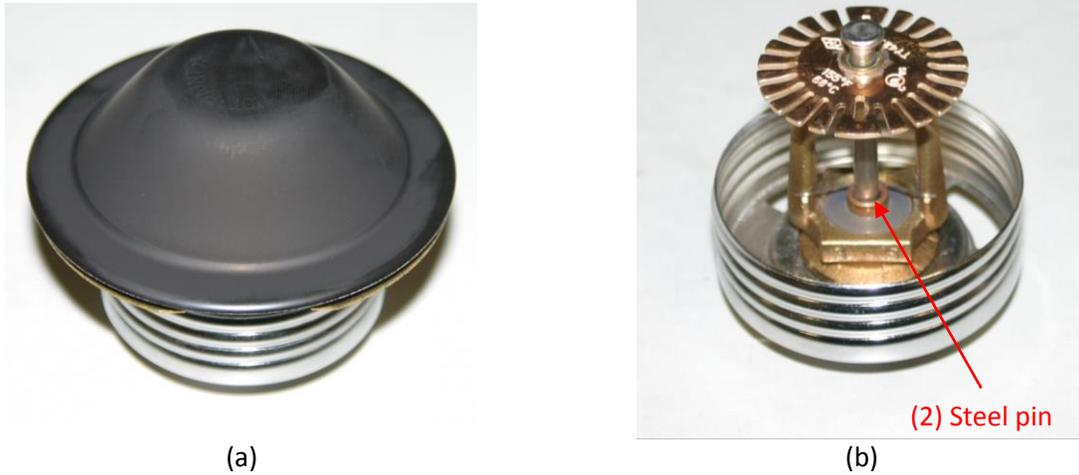
Figure 3-3: RAS B with a high emissivity coating applied to the escutcheon (1) (a). Glass bulb removed and replaced by a solid steel pin (2) (b)<sup>1</sup> (page 18).
