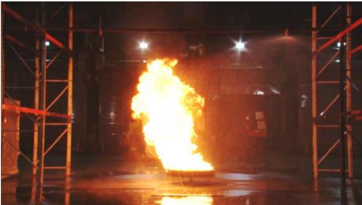
Figure 4-5: Flame leaning caused by activated RAS sprinkler on the right resulting in the activation of the conventional sprinkler.
