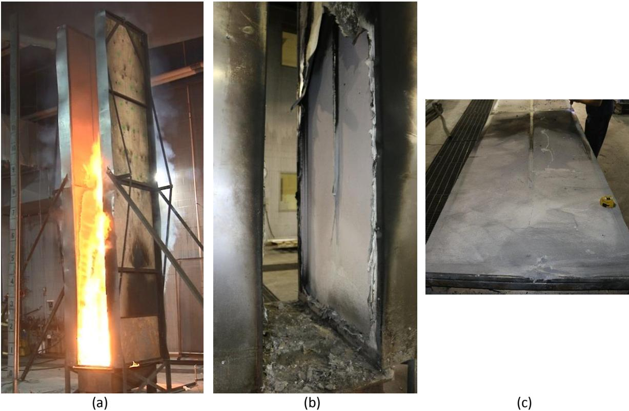
Figure 6-7: Pictures from Test #5: FR-core ACM with WRB-coated gypsum (a) peak propagation during test; (b) post-test assembly; and (c) post-test WRB-coated gypsum.
