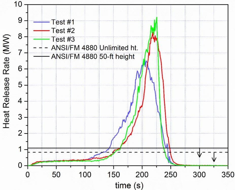
Figure 6-2: Chemical HRR results for combustible core ACM wall assemblies.
