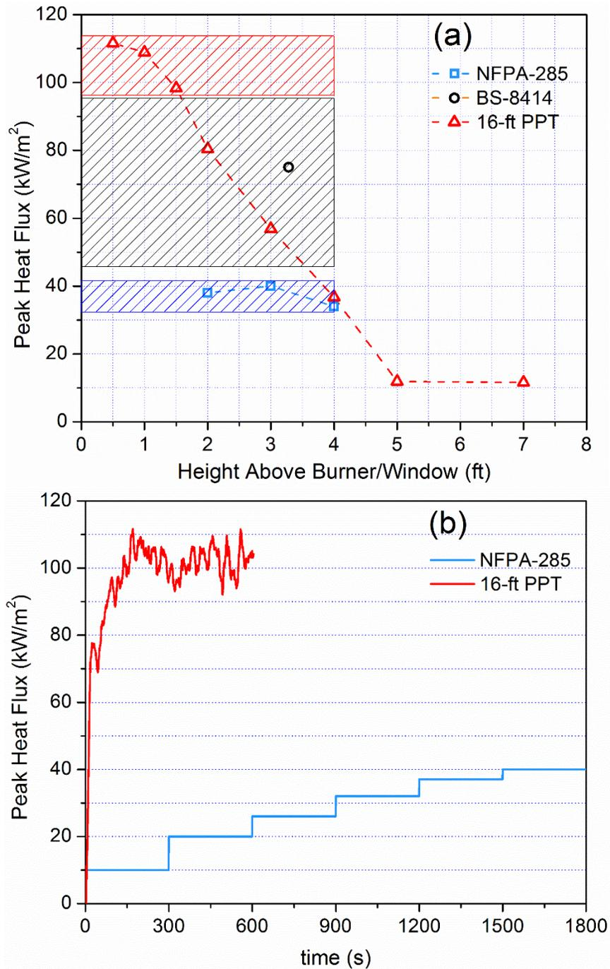
Figure 3-5: Comparison of heat fluxes to wall assembly in the three fire tests (a) heat flux as a function of height above the burner or window and shaded peak calibration heat flux range (b) peak calibration heat flux as a function of time for 16-ft PPT and NFPA-285.
