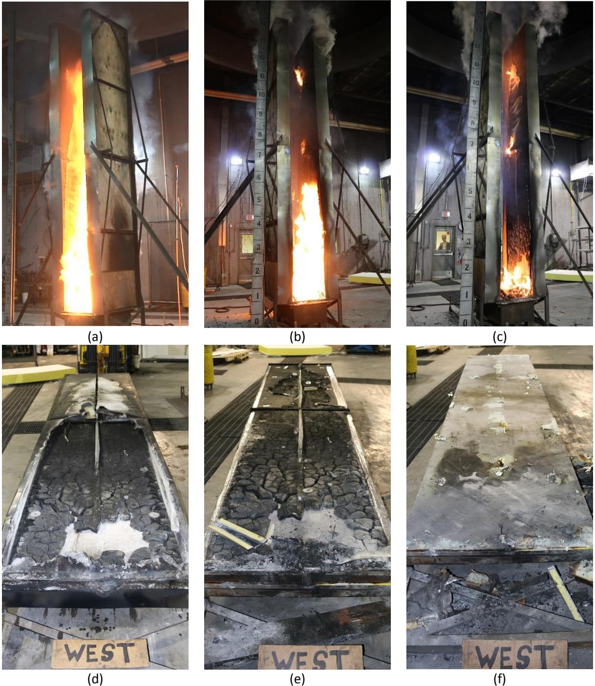
Figure 6-8: Pictures from Test #6: FR-core ACM with PIR1 and WRB-coated non-combustible backing (a) peak propagation during test at 415 s; (b) before propane shut-off at 900 s into test; (c) at 1200 s before test termination; (d) post-test assembly; (e) post-test insulation; and (f) post-test WRB-coated gypsum.
