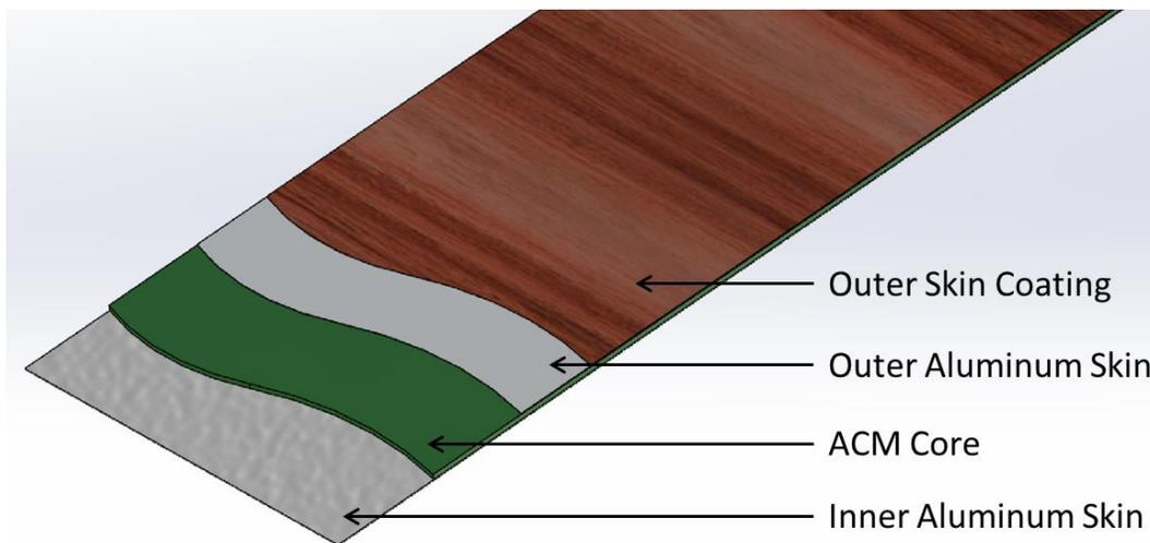
Figure 2-2: Cross-section of an ACM/MCM panel.
