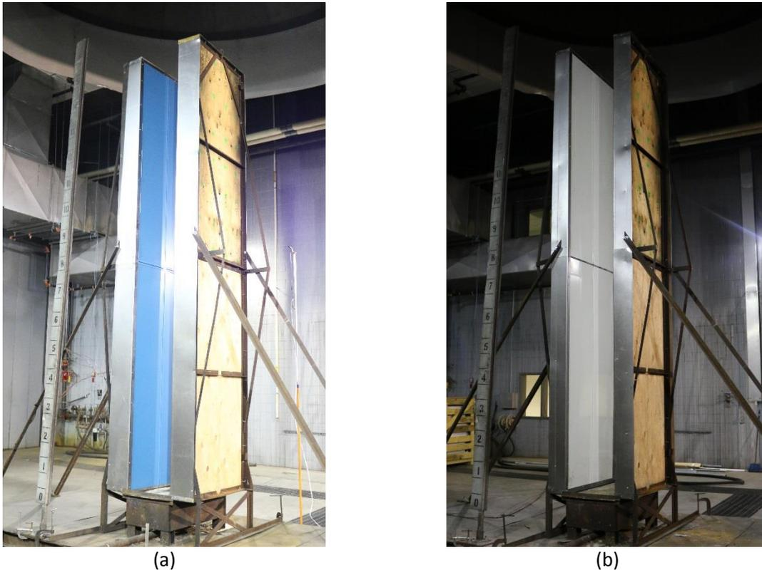
Figure 5-3: Examples of final ANSI/FM 4880 ACM wall assembly setups.
