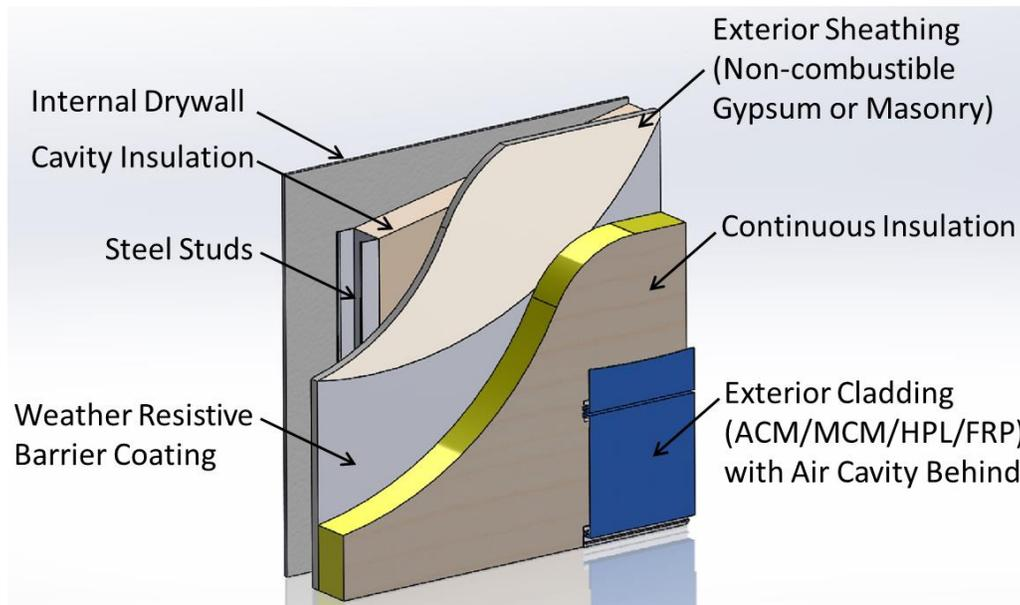
Figure 2-1: Example of a complete cladding assembly system. The external wall assembly is from exterior sheathing to exterior cladding.
