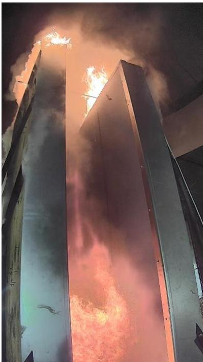
Figure 6-4: Cavity fire spread in Test #2: PP-core ACM with PIR1 and WRB-coated gypsum.
