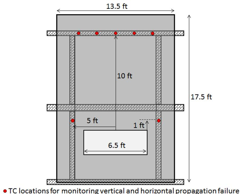
Figure 3-1: Schematic of setup and dimensions in NFPA-285 (not to scale).
