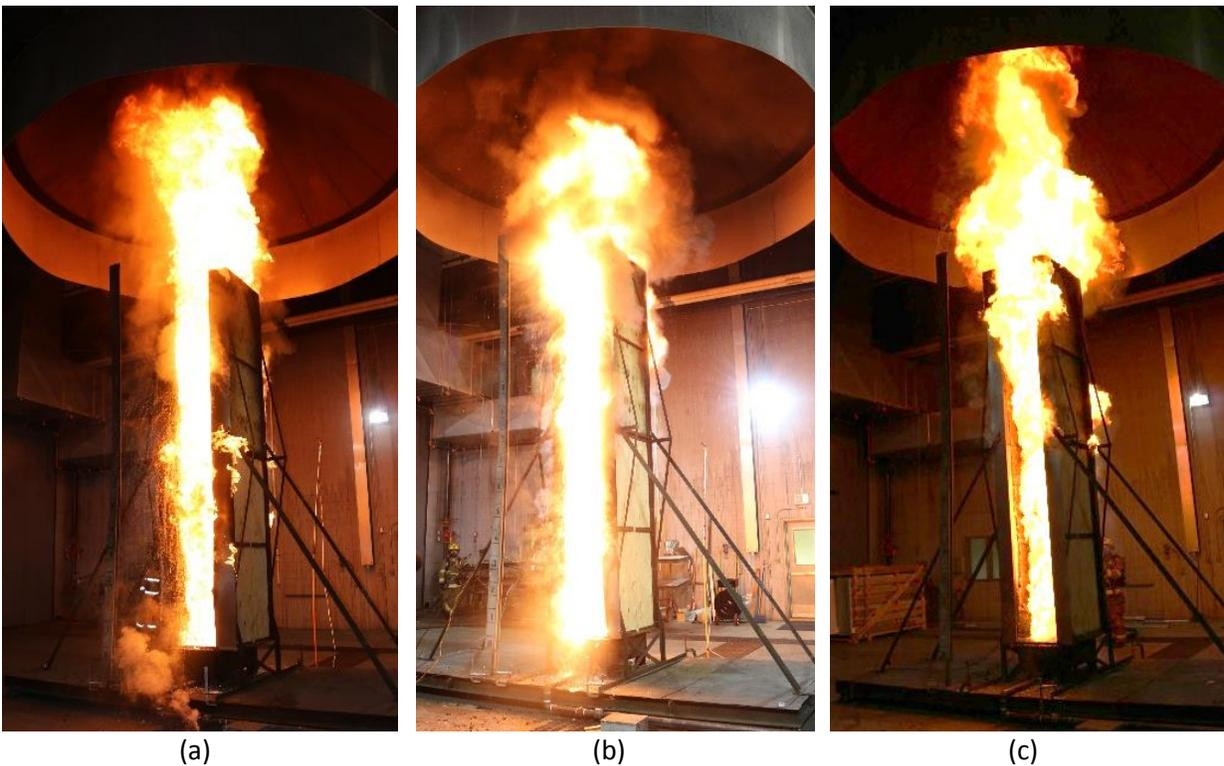
Figure 6-1: Images from the 16-ft PPTs at approximately 4 minutes from the ignition (a) Test #1: PP-core ACM with WRB-coated gypsum; (b) Test #2: PP-core ACM with PIR1 and WRB-coated gypsum; and (c) Test #3: PE-core ACM with non-combustible gypsum.
