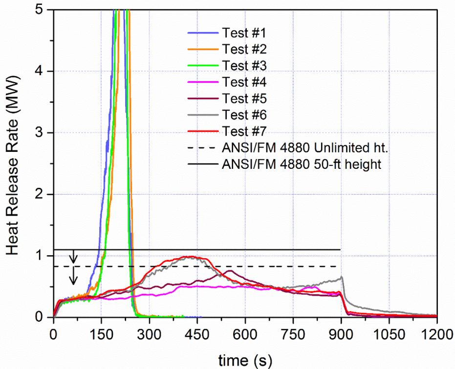
Figure 6-10: Chemical HRR profiles for all tests conducted using the 16-ft PPT procedure of ANSI/FM 4880.
