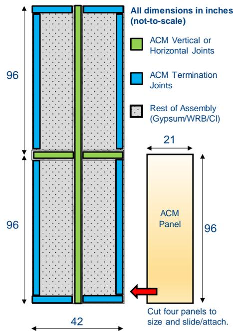
Figure 5-1: ACM layout on wall assembly for each frame of the 16-ft PPTs (dimensions in inches).
