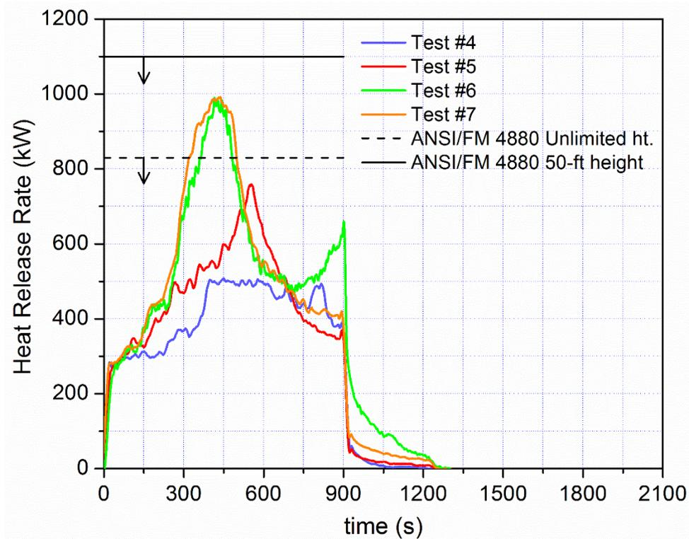
Figure 6-5: Chemical HRR results for FR-core ACM wall assemblies.
