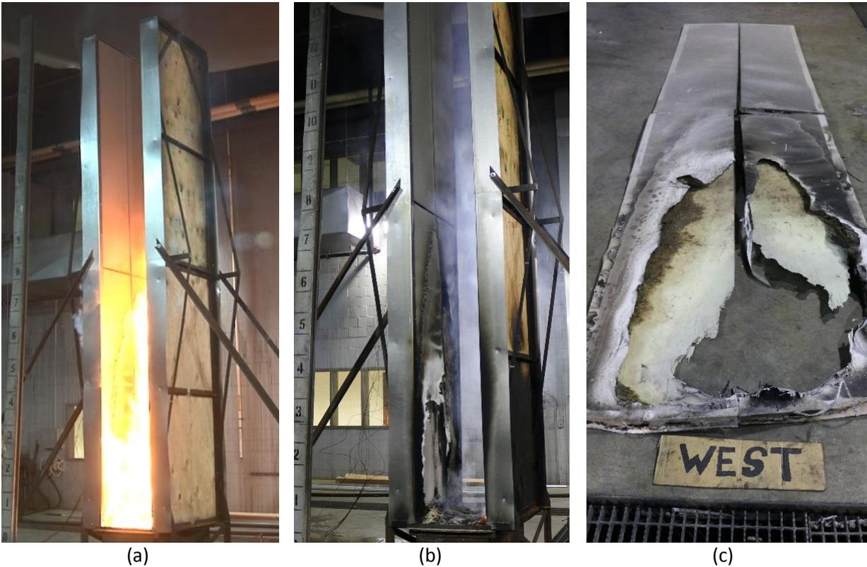
Figure 6-6: Pictures from Test #4: FR-core ACM with non-combustible backing (a) peak propagation during test; (b) post-test assembly; and (c) post-test panel.
