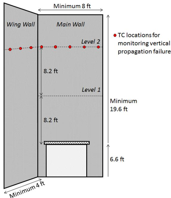
Figure 3-2: Schematic of wall specimen and dimensions in BS-8414-1 (not to scale).
