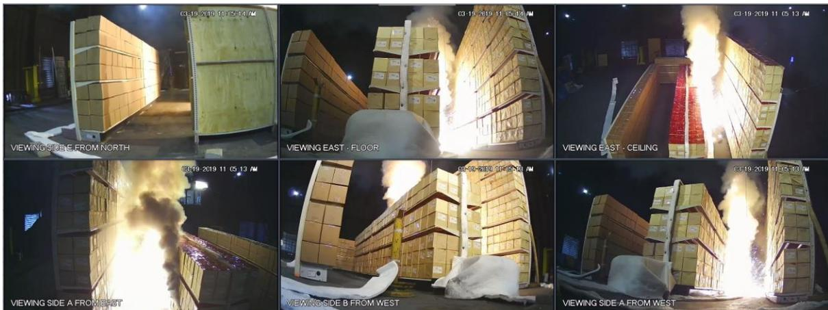
Figure A-21: Test 2 at 00:50: fire and smoke production intensifying in Side A with flames extending approximately 2.1 m (7 ft) above top of commodity.
