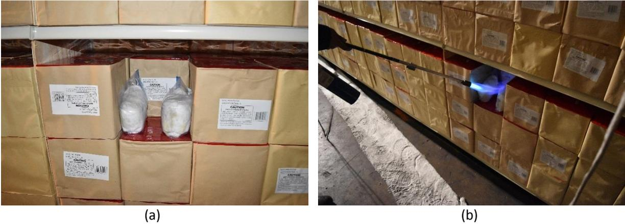
Figure 2-24: Ignition within the test array (a) close up showing ignitor placement, (b) ignition by application of propane torch.
