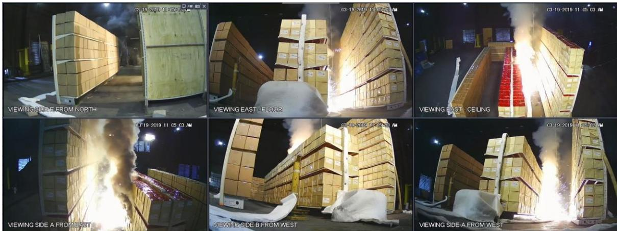
Figure A-20: Test 2 at 00:40: flames present on the face of Side A at ignition location.
