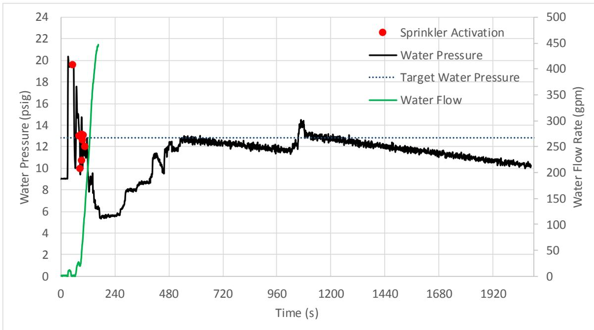
Figure 3-2: Test 1 water pressure and flow rate.
