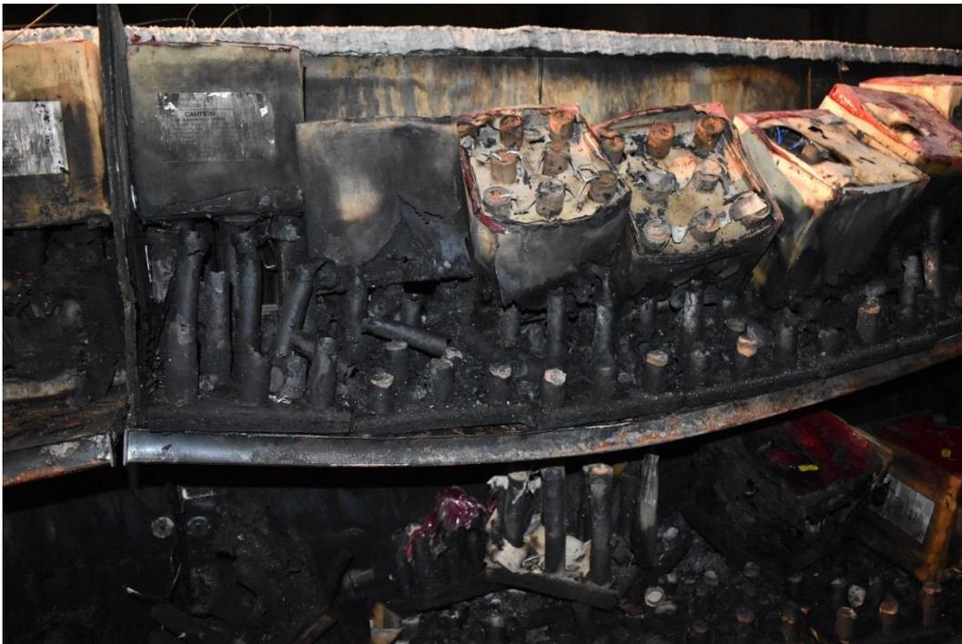
Figure C-6: Test 1 damage to top shelf commodity in Side A vertically aligned with ignition location (which was in bottom shelf).
