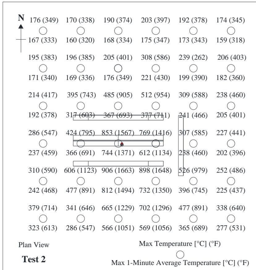
Figure B-32: Test 2 maximum instantaneous and 1-min average ceiling-level gas temperatures.
