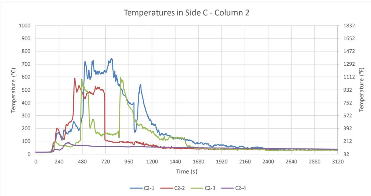
Figure B-50: Test 2 temperatures in Side C: Column 2.
