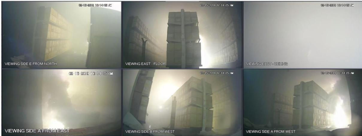
Figure A-12: Test 1 at 02:30: sprinklers continue to operate; the fire involves Side A and C.
