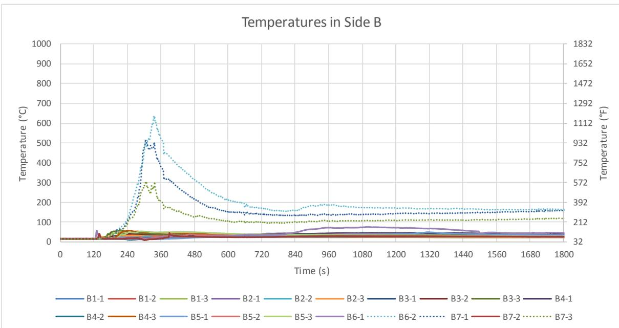
Figure B-44: Test 2 temperatures in Side B. Note that TCs B6-3 malfunctioned during the test and suspect data have not been plotted.
