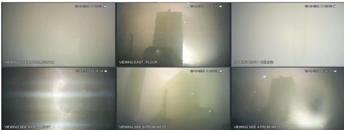
Figure A-30: Test 2 at 02:30: fire confined to Sides A and C, visibility decreasing.
