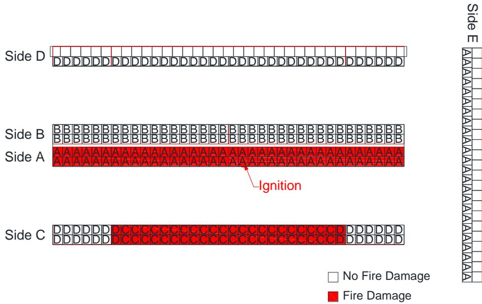
Figure 3-3: Test 1 plan view of maximum extent of fire damage.
