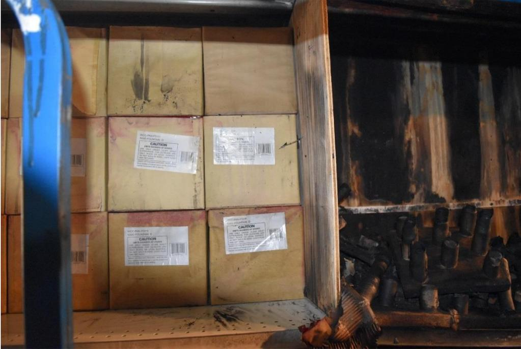
Figure C-11: Test 1 showing example of unburned commodity on one side of flame break and burned commodity on the other. Location in Side C. Note some commodity has been removed as part of the post-test deconstruction process.
