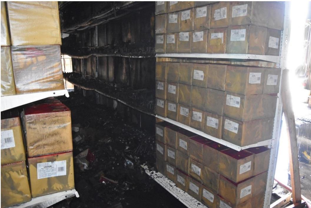
Figure C-24: Test 2 Side C looking toward east, shelves 1-3, fire damage reached transverse flame break on shelves 1-3 but did not burn through them.
