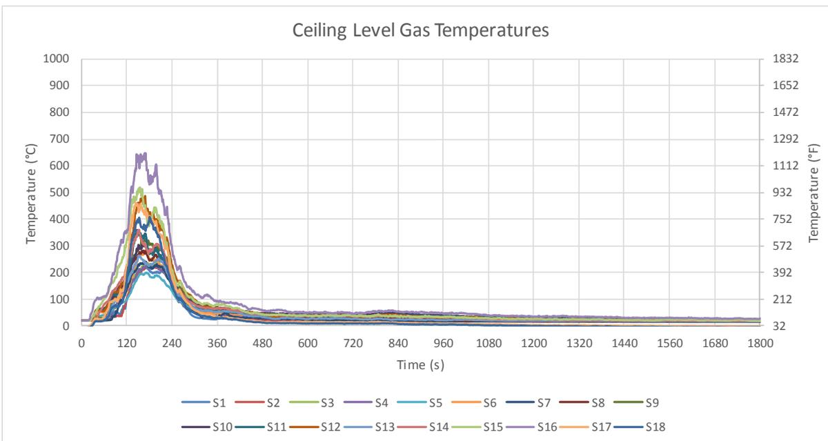
Figure B-1: Test 1 ceiling-level gas temperatures at TC locations 1-18.
