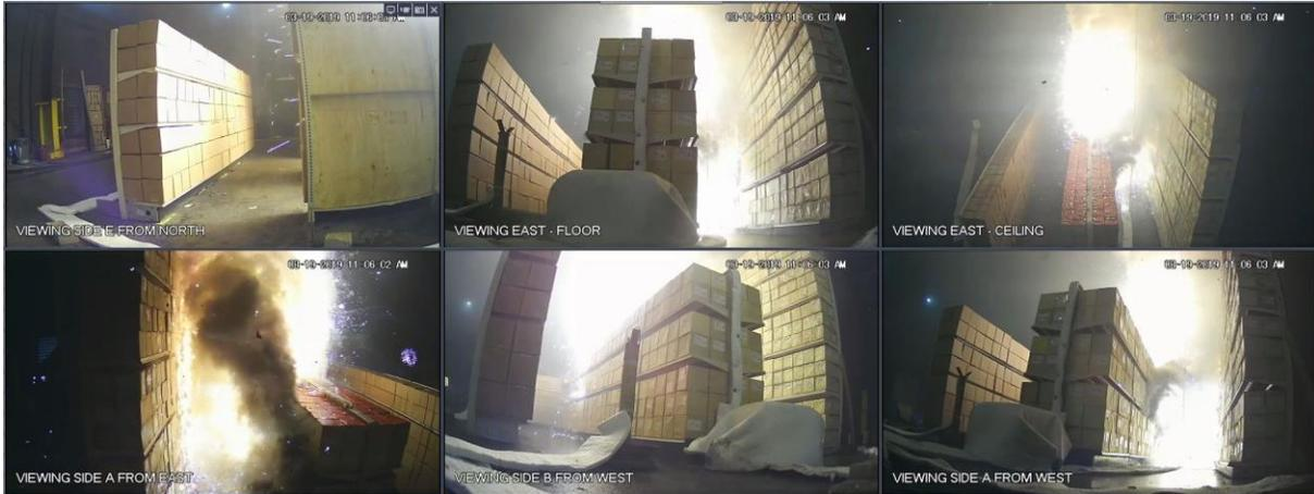
Figure A-25: Test 2 at 01:40: one sprinkler operating and fire and smoke production continue to intensify.
