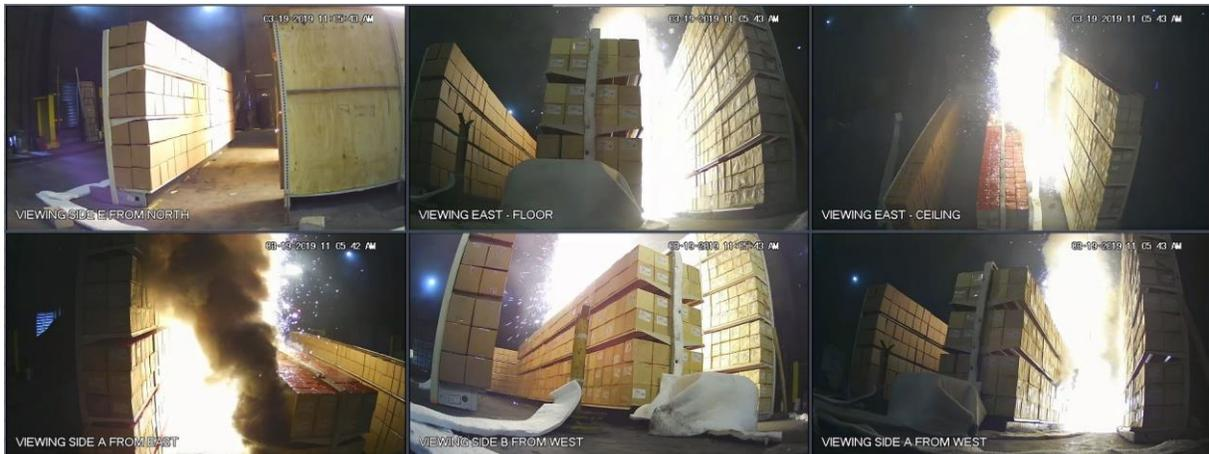
Figure A-23: Test 2 at 01:20: fire and smoke production intensifying in Side A, sparks being projected throughout lab space and showering down on top of Side B, Side C ignited at 01:19.
