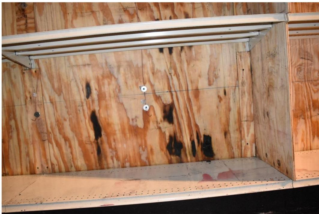
Figure C-16: Test 1 Side B after commodity has been removed showing localized area of burn through of longitudinal flame break in bottom shelf directly behind ignition location.
