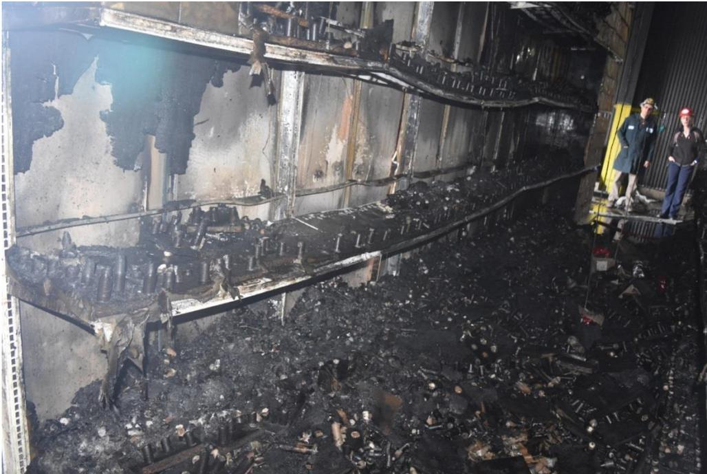
Figure C-22: Test 2 Side C looking toward west, shelves 1-3, showing sheet rock that backs longitudinal flame break which is nearly completely consumed in this region, transverse flame breaks consumed on west, intact on east, fire damage at eastern end in shelves 1-4.
