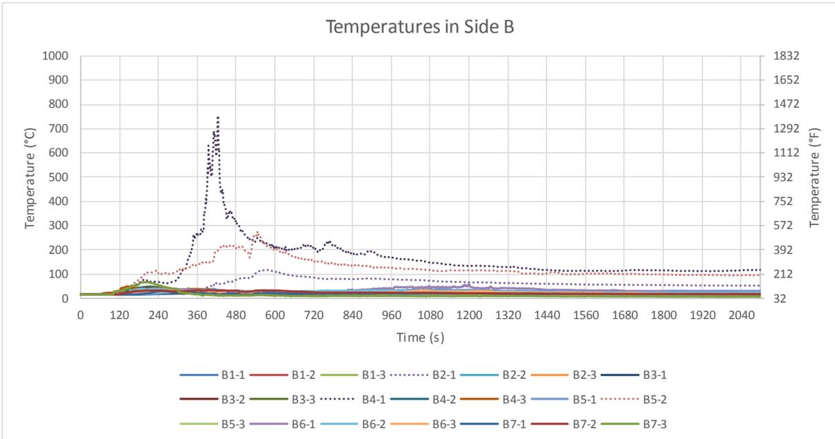
Figure B-15: Test 1 temperatures in Side B. Elevated temperatures are witnessed in the absence of fire on Side B. The longitudinal flame break on Side B had been minorly breached allowing the transport of hot gases. Refer to Section C.1 in Appendix C.
