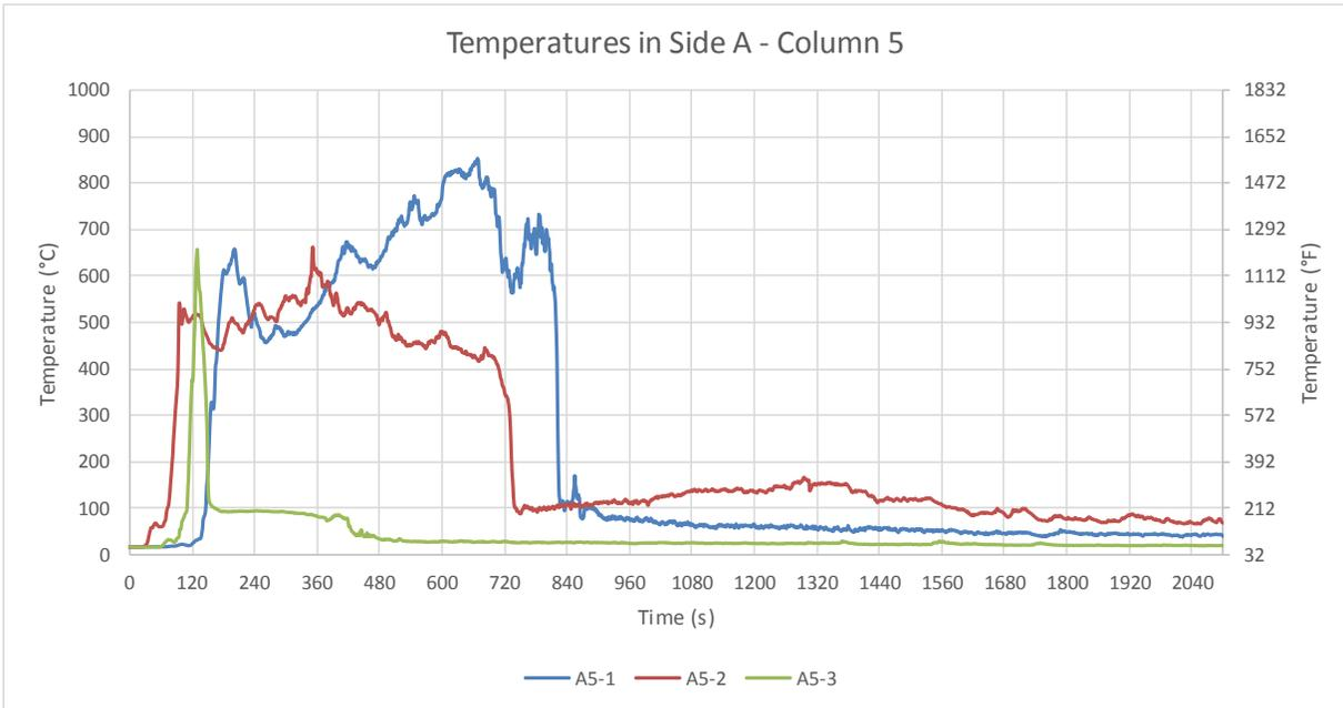
Figure B-11: Test 1 temperatures in Side A: Column 5.
