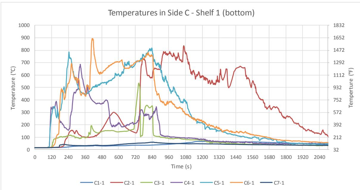
Figure B-16: Test 1 temperatures in Side C: Shelf 1 (bottom).
