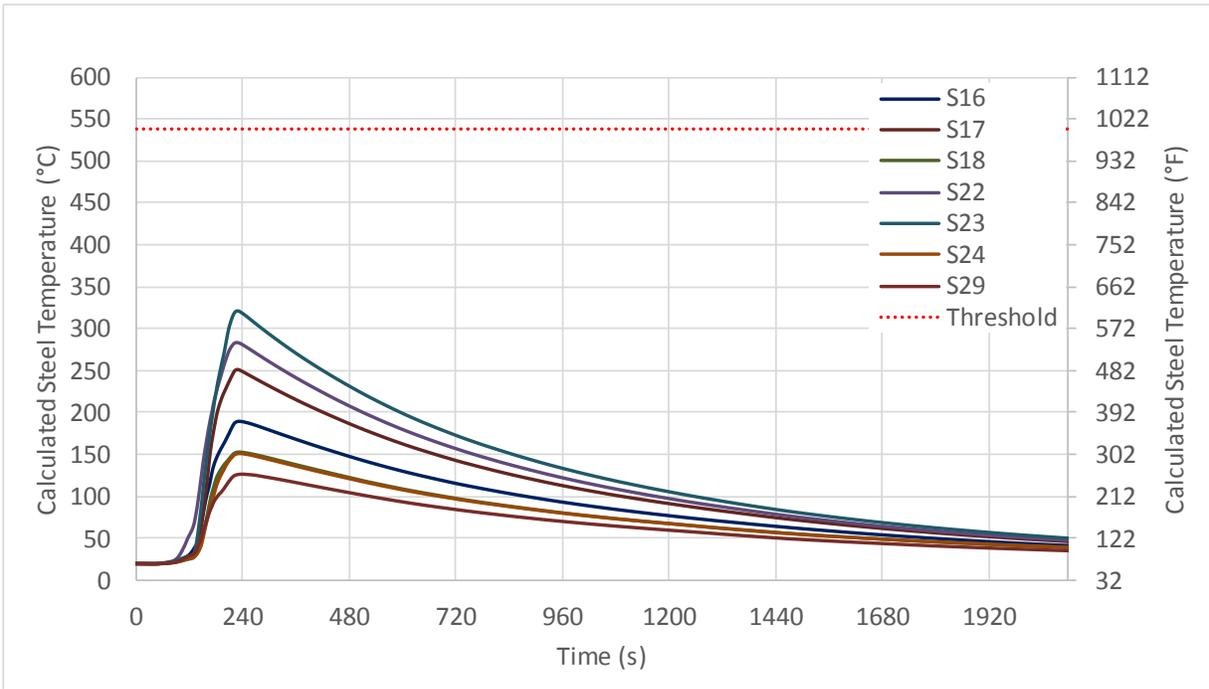
Figure 3-10: Test 2 calculated ceiling-level steel temperatures for locations where gas temperatures exceeded 538°C (1000°F).
