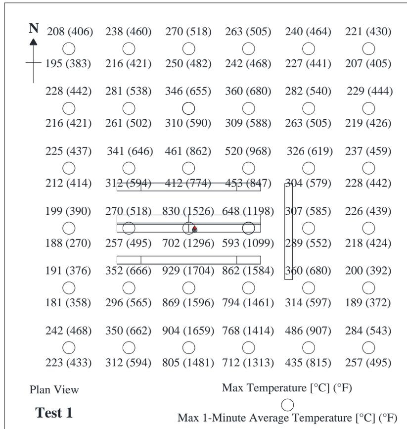
Figure B-3: Test 1 maximum instantaneous and 1-min average ceiling-level gas temperatures.
