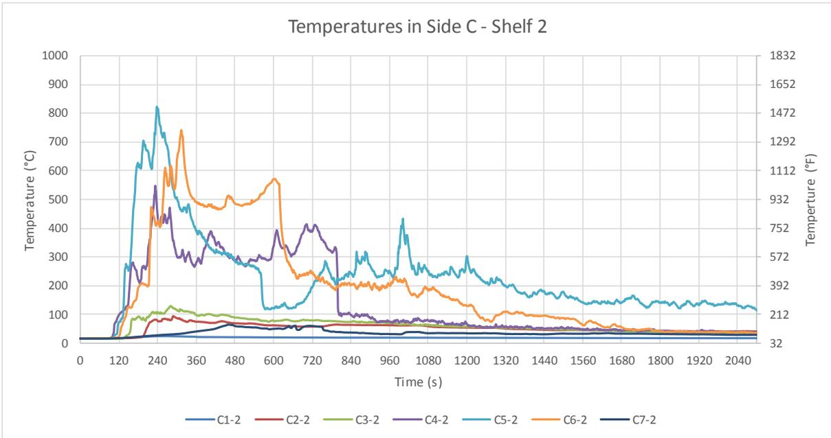
Figure B-17: Test 1 temperatures in Side C: Shelf 2.
