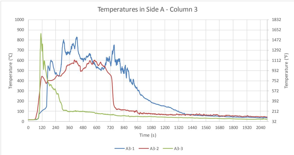
Figure B-9: Test 1 temperatures in Side A: Column 3.
