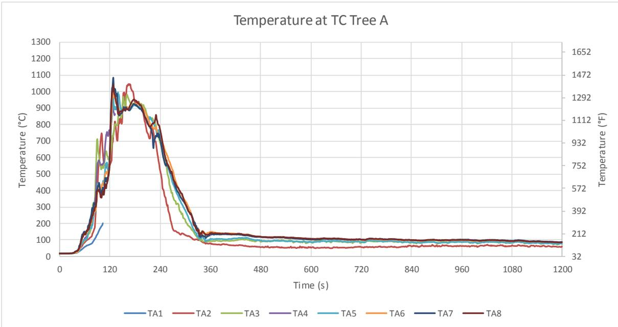
Figure B-57: Test 2 temperatures at TC Tree A. Note that TCs TA1 and TA4 malfunctioned during the test and suspect data have not been plotted. Their functionality was checked post-test and found to be inoperative. High temperatures are a result of the proximity of the fire to the TC tree and are not indicative of vertical temperature profiles in other regions of the test array. Note different temperature scale.
