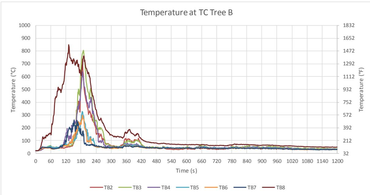
Figure B-29: Test 1 temperatures at TC Tree B. TC TB1 malfunctioned and the data is not presented. Increase in temperature at TB2-TB7 after 01:40 is likely due to the arrival of the flame front. Their magnitude prior to this time are an indication of vertical temperature profiles not directly exposed to the fire plume. In hindsight it would have been advantageous to install a TC tree in the aisle space between Sides B and D to provide gas temperature for regions not directly exposed to the fire.
