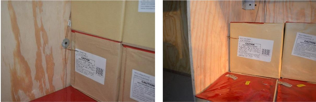
Figure 2-27: TC installation in shelving units (a) TC along perpendicular flame break, (b) TC located on transverse flame break. TCs located such that bead is 5.1 cm (2 in.) from the flame break.
