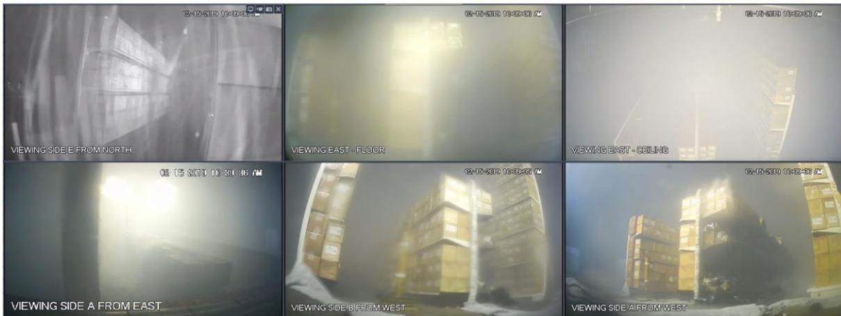
Figure A-18: Test 1 at 28:00: camera 1 in infrared shows water droplets, cameras 2, 5 and 6 show fire damage in bottom and middle shelf of Side A.
