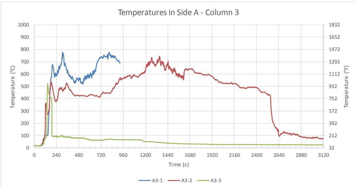
Figure B-38: Test 2 temperatures in Side A: Column 3. Note that TC A3-1 malfunctioned during the test and suspect data have not been plotted. Its functionality was checked post-test and found to be inoperative.
