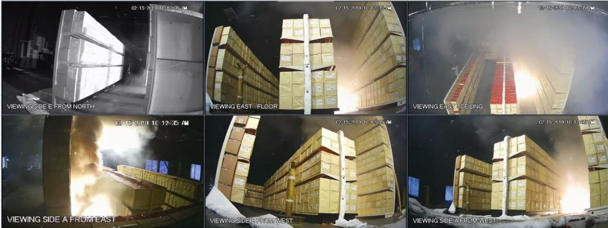
Figure A-3: Test 1 at 01:00: 3 s after 1<sup>st</sup> sprinkler activation, fire and smoke production intensifying in ignition region.
