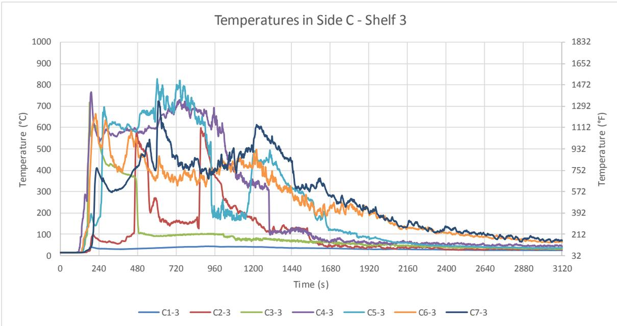
Figure B-47: Test 2 temperatures in Side C: Shelf 3.
