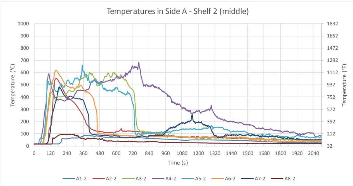
Figure B-5: Test 1 temperatures in Side A: Shelf 2 (middle).
