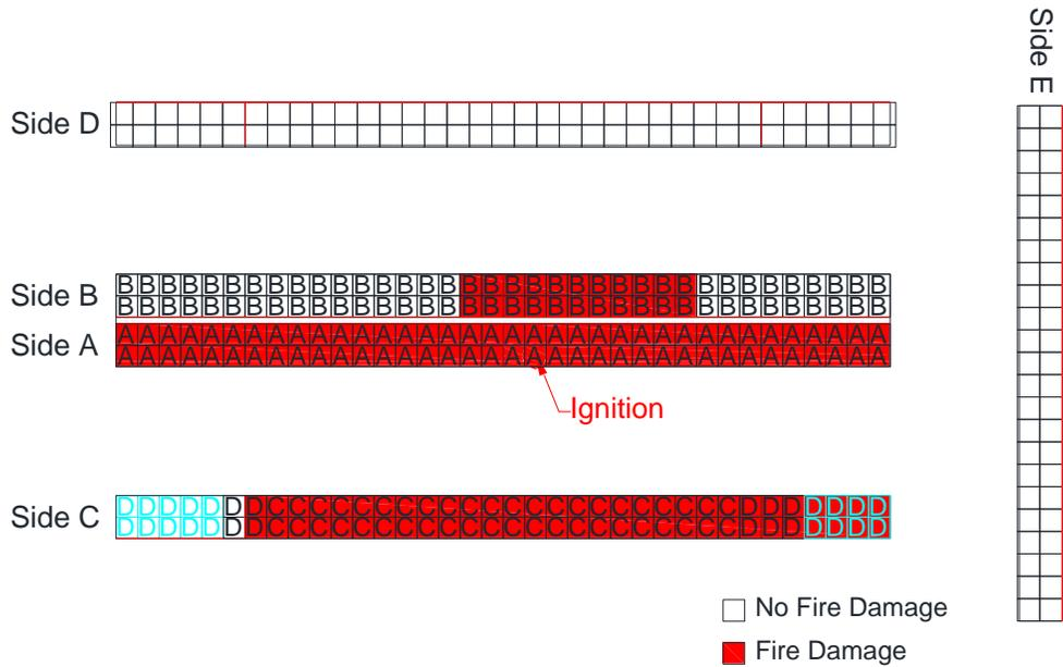
Figure 3-8: Test 2 plan view of maximum extent of fire damage.
