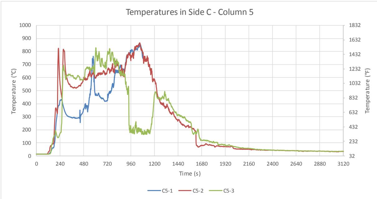
Figure B-53: Test 2 temperatures in Side C: Column 5. Note that TC C5-1 malfunctioned during the test and suspect data have not been plotted. Its functionality was checked post-test and found to be inoperative.
