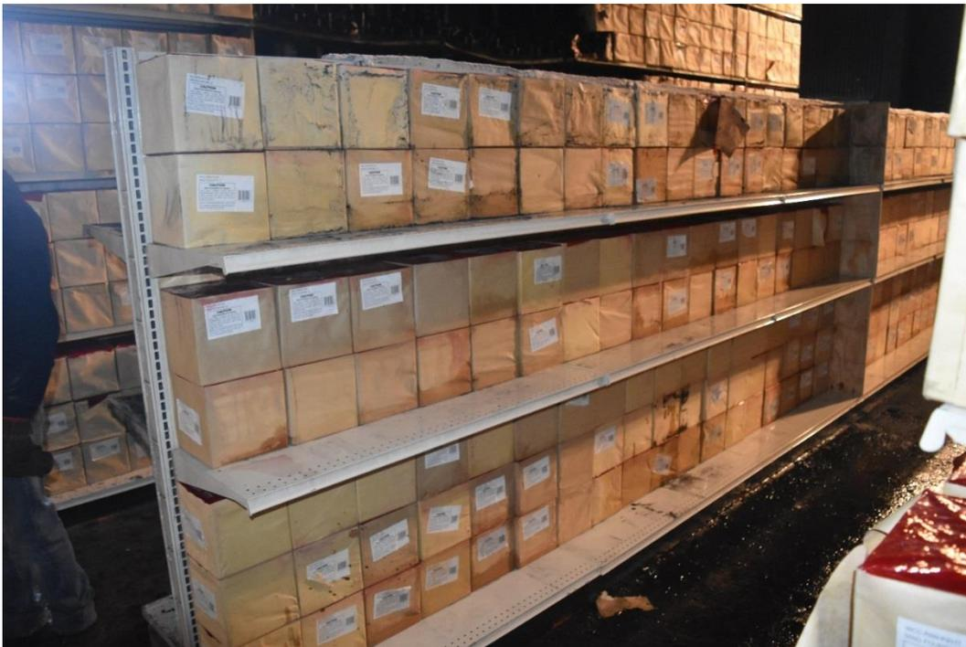
Figure C-14: Test 1 Side B. Front row of commodity has been removed during the post-test deconstruction process to inspect for potential fire damage. Side B sustained no fire damage to the commodity.
