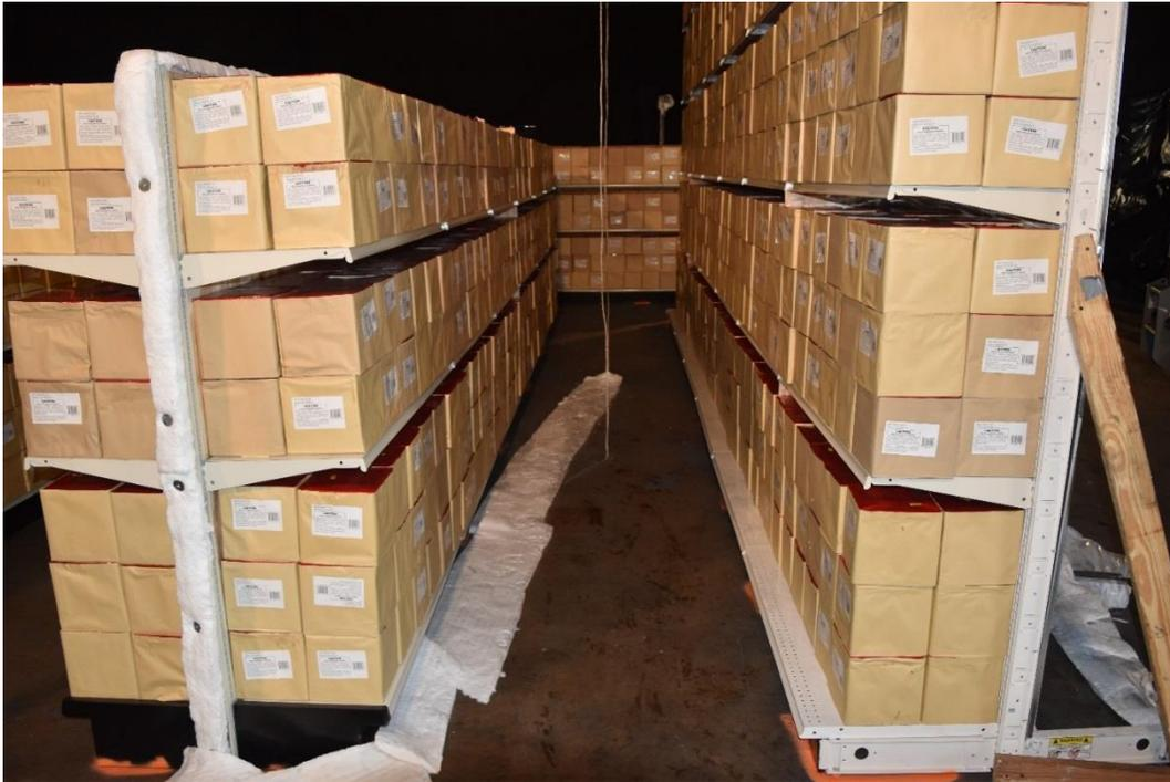
Figure 2-17: Final construction of test array looking eastward down ignition aisle (between Sides A and C).
