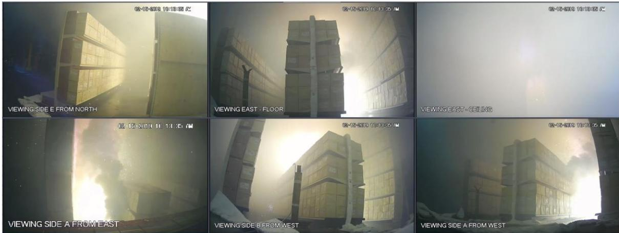
Figure A-9: Test 1 at 02:00: sprinklers continue to operate, fire and smoke production intensifying.
