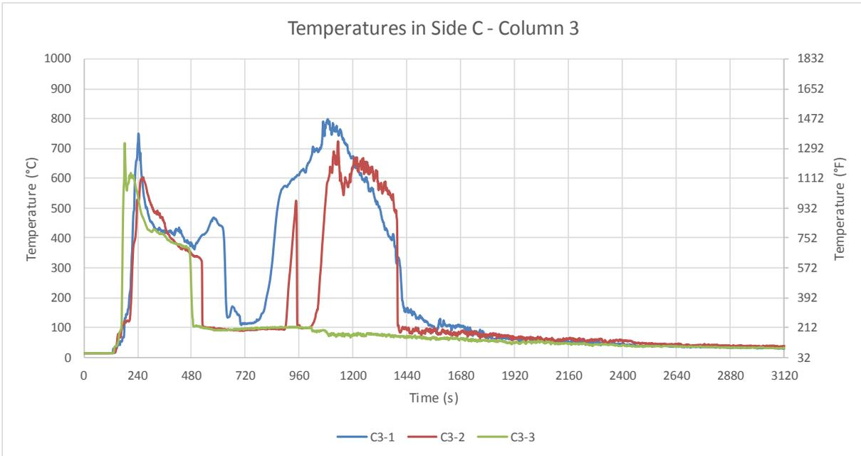
Figure B-51: Test 2 temperatures in Side C: Column 3.
