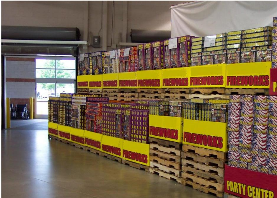
Figure 1-1: Example of fenced palletized arrangement.
