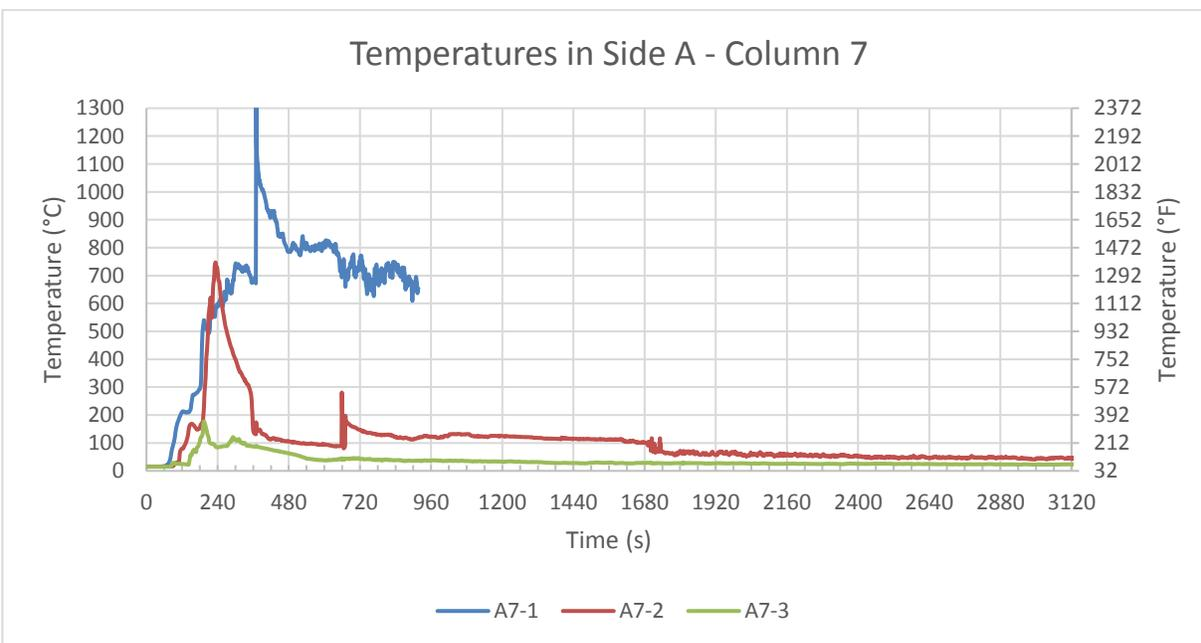
Figure B-42: Test 2 temperatures in Side A: Column 7. Note that TC A7-1 malfunctioned during the test and suspect data have not been plotted, additionally, it exceeded the maximum rating of a Type K TC at 06:10 after which time the temperature decreased. Its functionality was checked post-test and found to be inoperative. Note different temperature scale.
