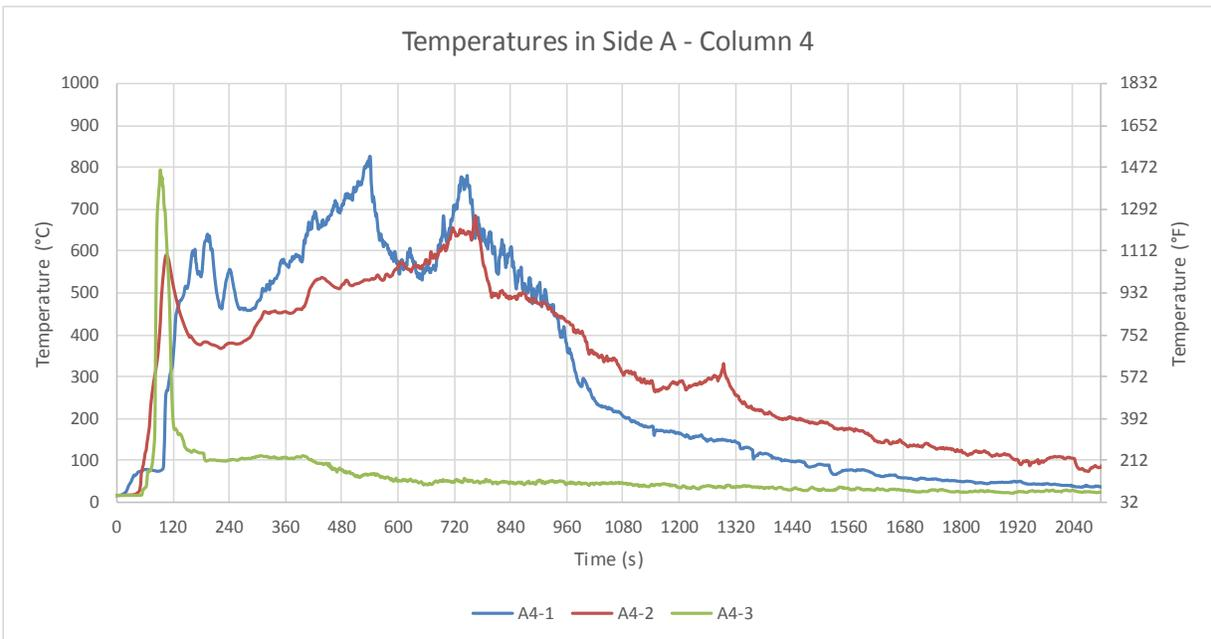
Figure B-10: Test 1 temperatures in Side A: Column 4.
