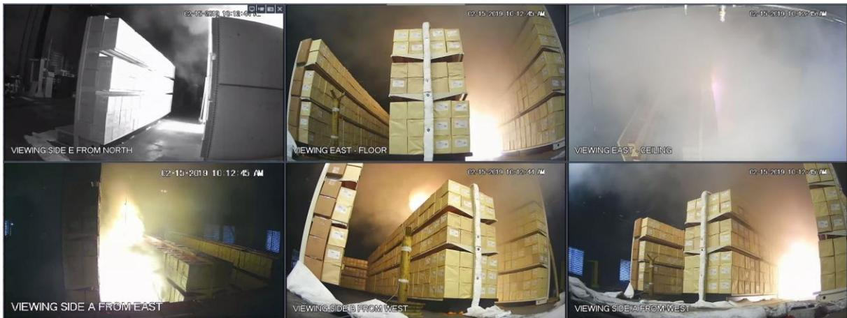
Figure A-4: Test 1 at 01:10: one sprinkler operating, fire and smoke production intensifying in Side A.
