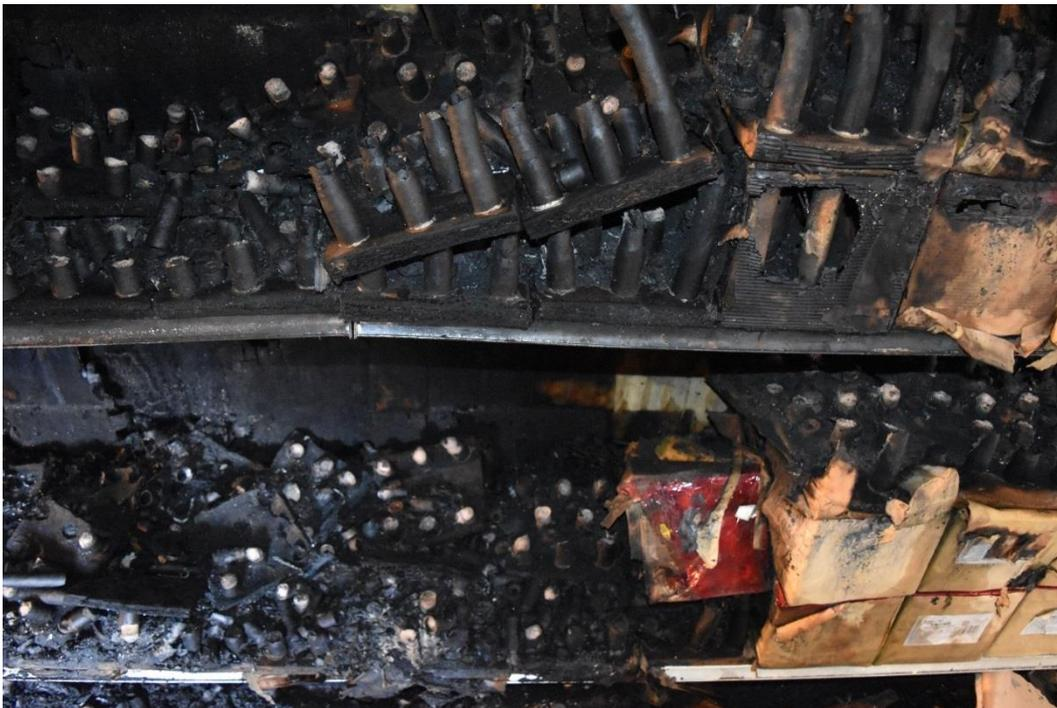
Figure C-10: Test 1 detail of typical residual commodity in regions where flame spread ceased.
