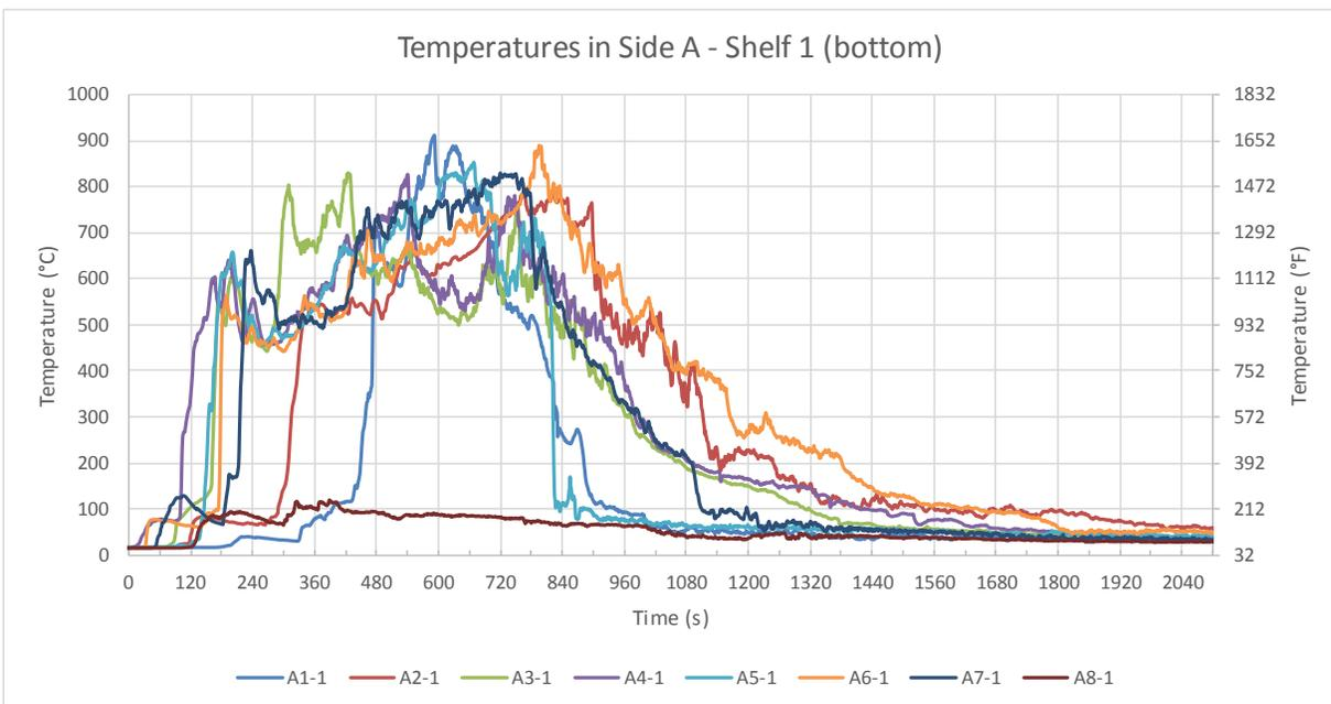
Figure B-4: Test 1 temperatures in Side A: Shelf 1 (bottom) Temperature increase at 05:30 at location A1-1 coincides with visual observation (Figure A-17) of flames reaching west end of Shelf 1.
