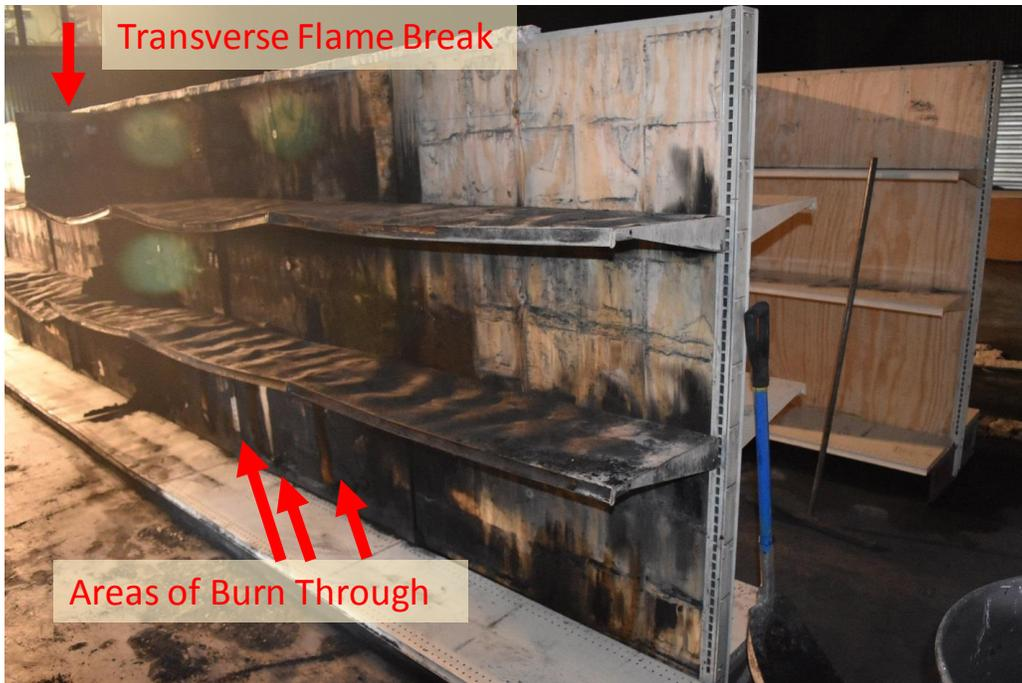
Figure C-18: Test 1 Side A (looking westward) after commodity has been removed showing transverse flame breaks on bottom and middle shelves consumed but intact on top shelf, examples of burn through of longitudinal flame break, and deformation of metal shelves.
