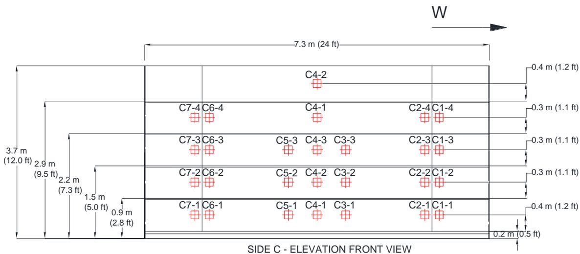
Figure 2-5: Front elevation view of Side C showing shelf height and thermocouple nomenclature and vertical dimensions of locations. Red crosses represent TCs.
