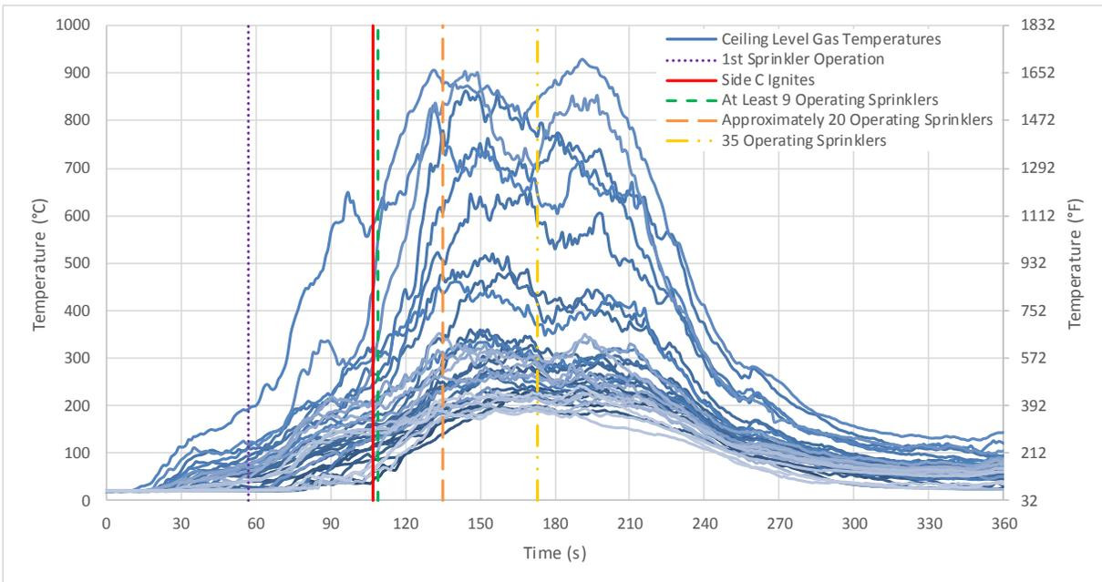
Figure 4-1: Test 1 ceiling-level gas temperatures and relevant events.
