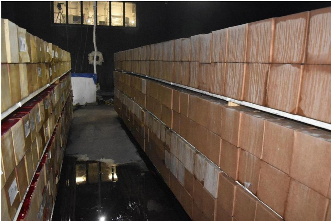
Figure C-26: Test 2 post-test image of Side B (left) and Side D (right) looking westward. Side D sustained water damage only (no fire). Fireworks on the top shelf of Side B sustained fire damage.
