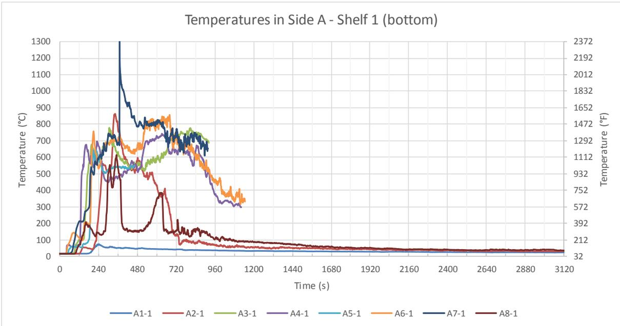
Figure B-33: Test 2 temperatures in Side A: Shelf 1 (bottom). Note that TCs A3-1, A4-1, A5-1, A6-1 and A7-1 malfunctioned during the test and suspect data have not been plotted. A7-1 exceed the maximum rating of a Type K TC at 06:10 after which time the temperature decreased. Their functionality was checked post-test and found to be inoperative. Note different temperature scale.
