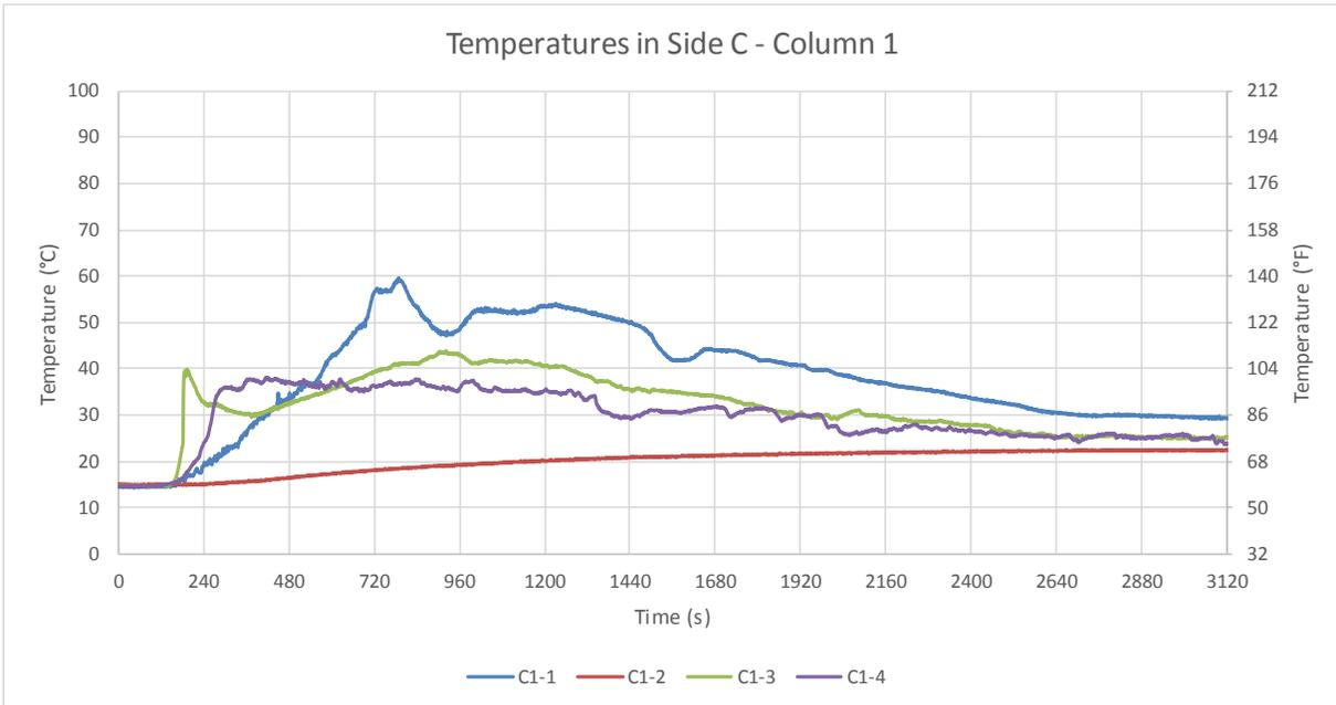
Figure B-49: Test 2 temperatures in Side C: Column 1. Note different temperature scale.
