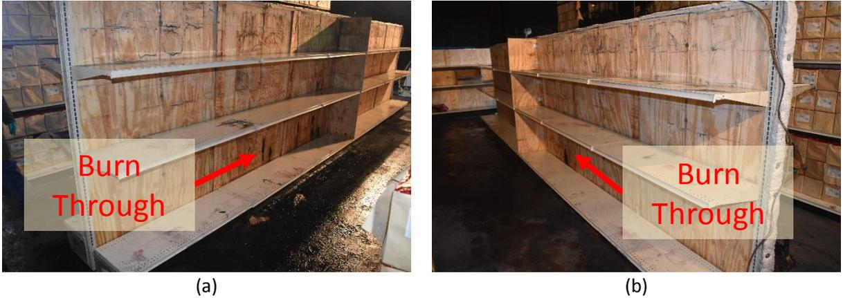
Figure D-15: Test 1 Side B after commodity has been removed showing localized areas of burn through of the longitudinal flame break from fire located in Side A (a) looking westward (b) looking eastward. Detail image shown in Figure C-16.
