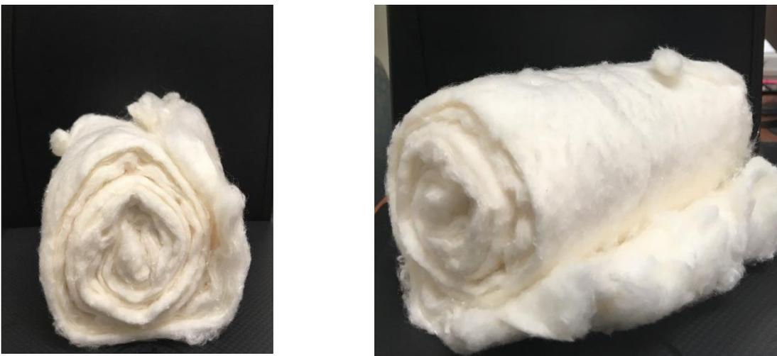
Figure 2-23: Standard full cellucotton ignitor (without bag and gasoline).
