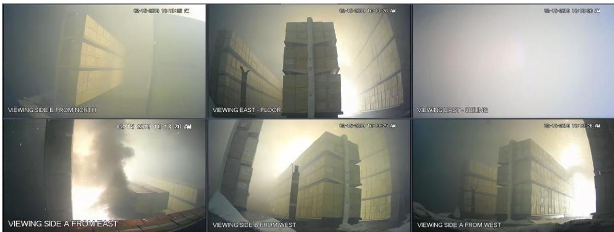
Figure A-8: Test 1 at 01:50: at least nine sprinklers operating, fire and smoke production intensifying.
