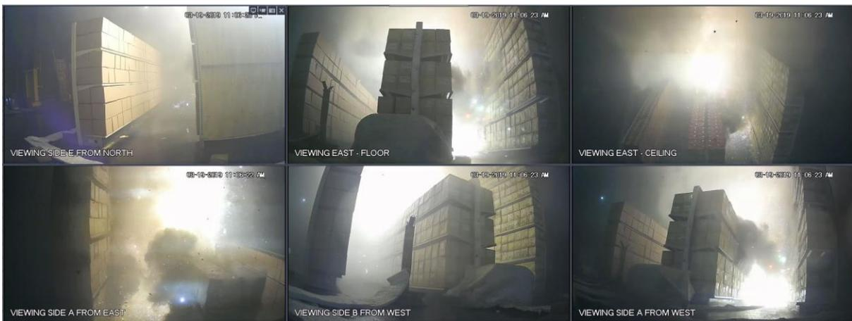
Figure A-27: Test 2 at 02:00: at least 10 sprinklers operating, fire continues to intensify and visibility is becoming obscured.
