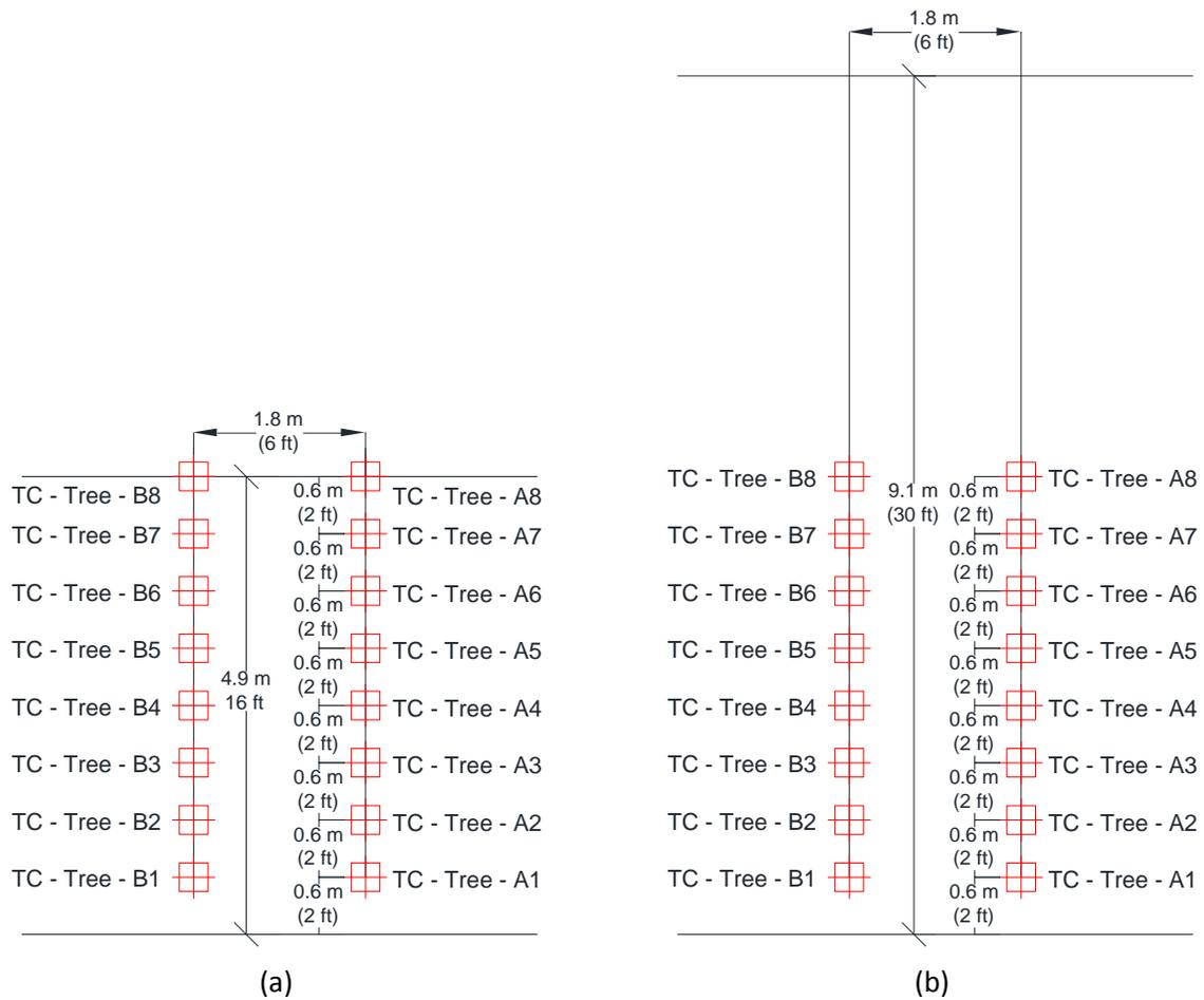
Figure 2-28: Front elevation of TC Tree A and B for (a) Test 1 and (b) Test 2.
