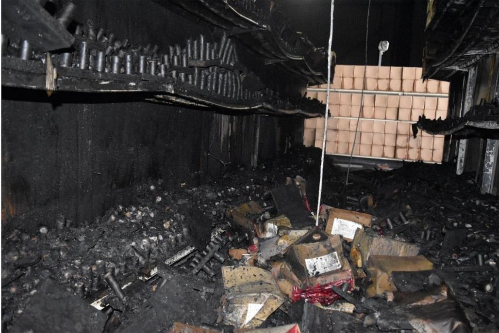
Figure C-21: Test 2 damage to Sides A (right) and C (left), looking toward east, with collapsed commodity in aisle which occurred during the test and not as a result of the firefighting efforts.
