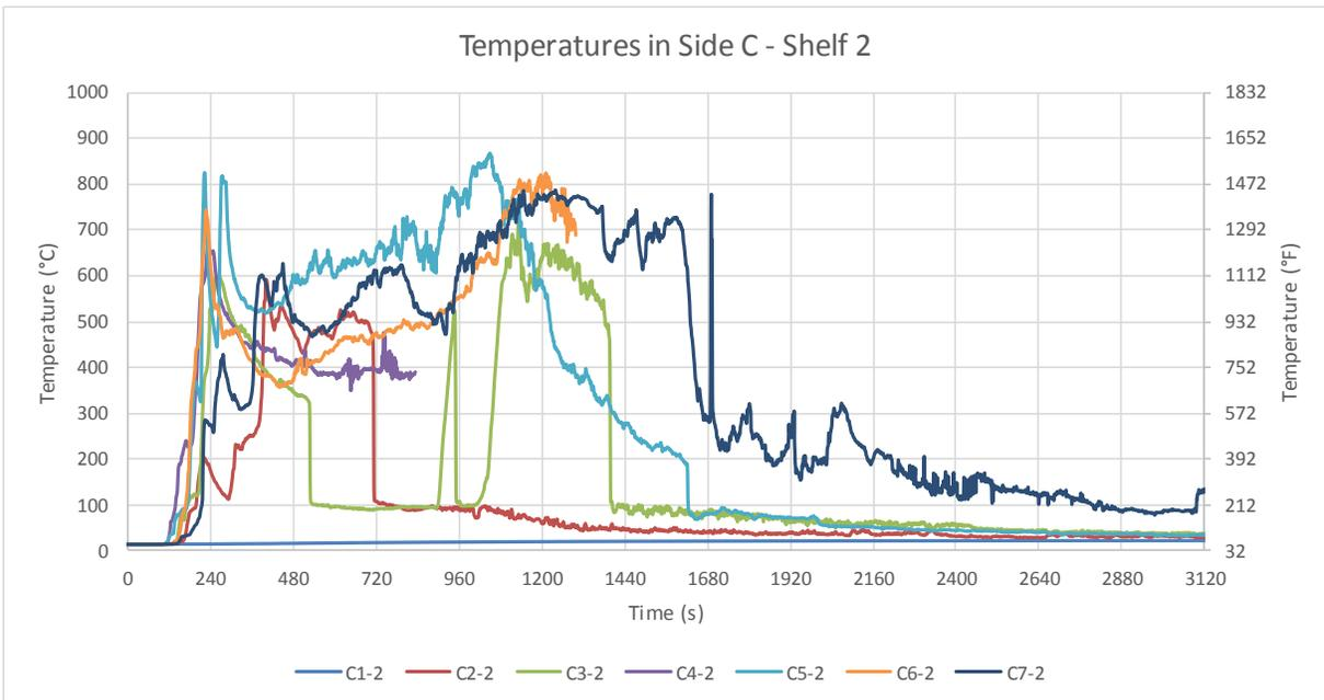
Figure B-46: Test 2 temperatures in Side C: Shelf 2. Note that TCs C4-2, C6-2 and C7-2 malfunctioned during the test and suspect data have not been plotted. Their functionality was checked post-test and found to be inoperative.
