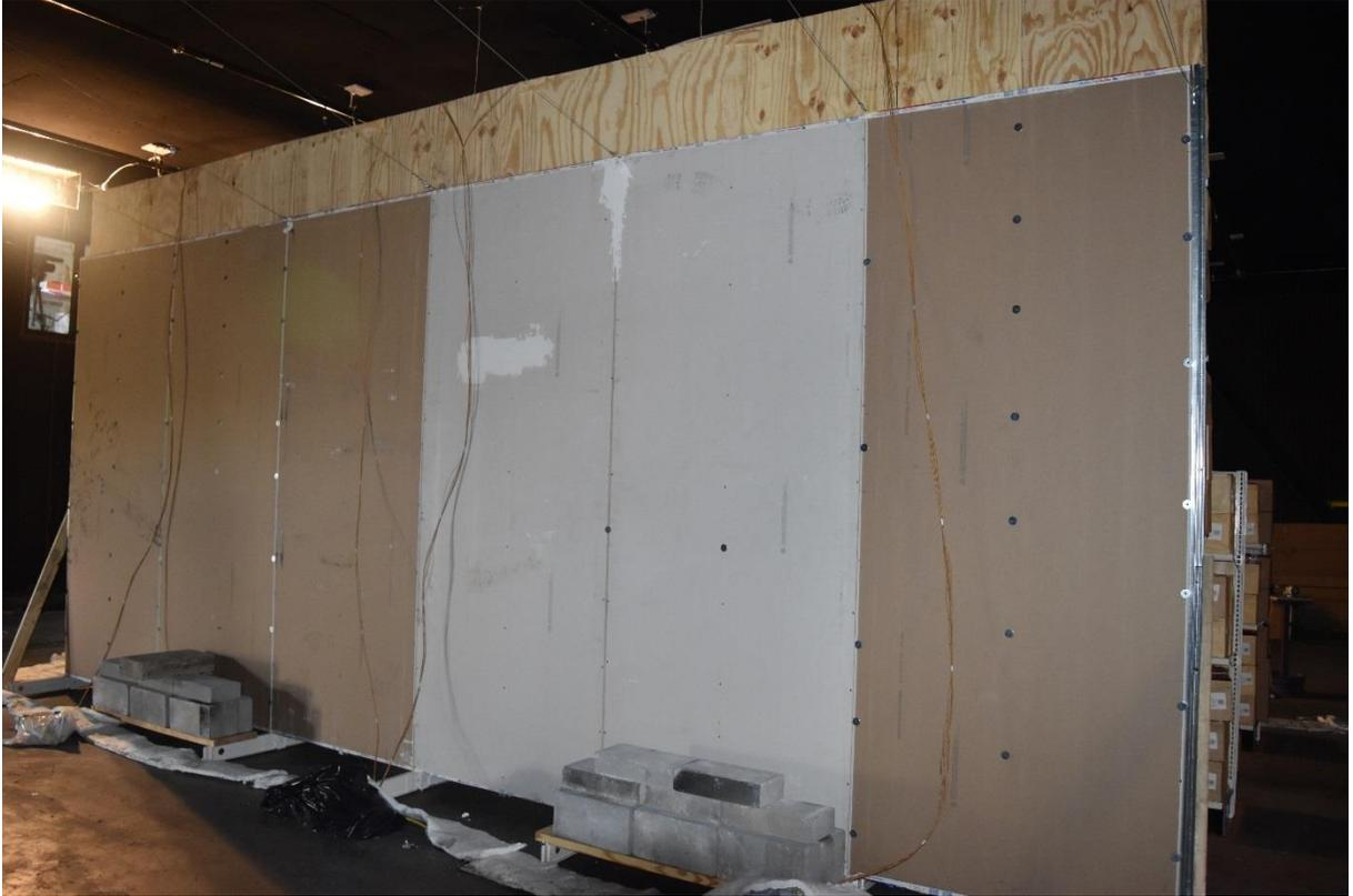
Figure 2-9: Sheet rock simulating interior wall on back of Side C.
