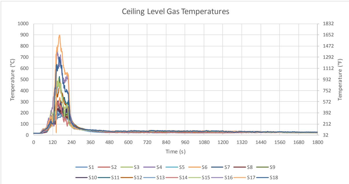
Figure B-30: Test 2 ceiling-level gas temperatures at TC locations 1-18.
