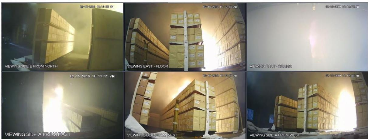
Figure A-5: Test 1 at 01:20: one sprinkler operating, fire and smoke production intensifying in Side A (camera 1 had transitioned from black and white colored infrared to full color due to the luminosity of the fire).
