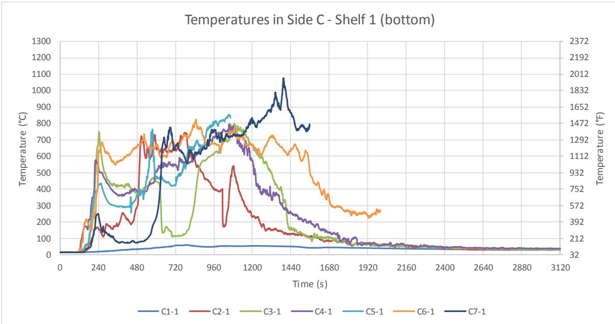
Figure B-45: Test 2 temperatures in Side C: Shelf 1 (bottom). Note that TCs C3-1, C4-1, C5-1, C6-1 and C7-1 malfunctioned during the test and suspect data have not been plotted. Their functionality was checked post-test and found to be inoperative. Note different temperature scale.
