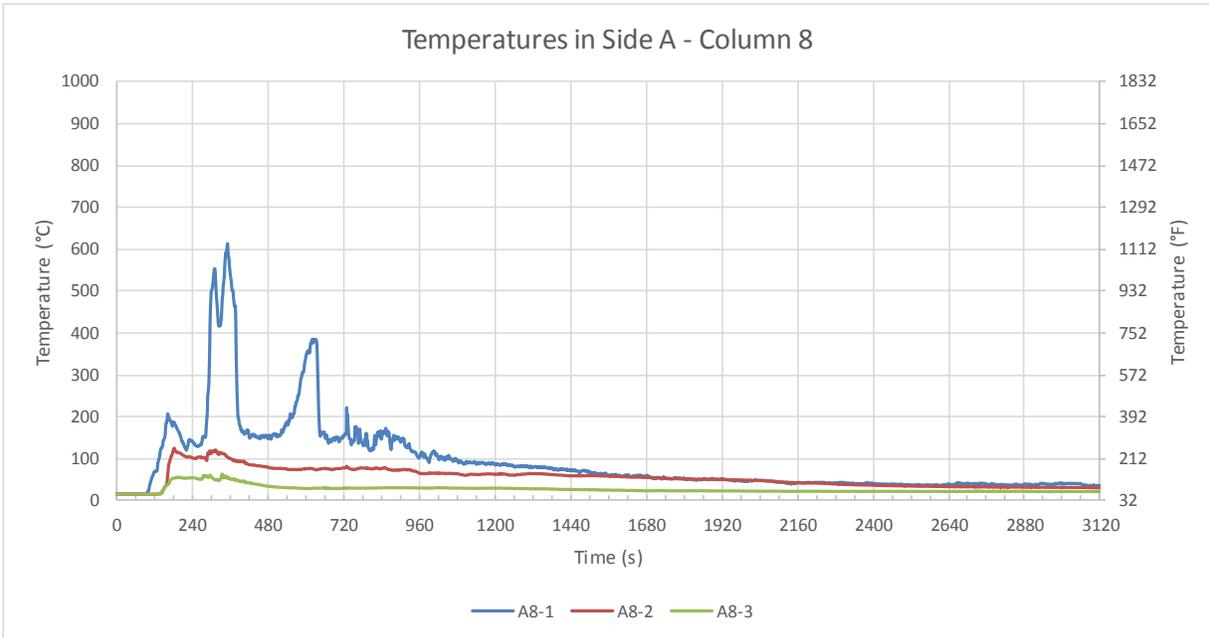
Figure B-43: Test 2 temperatures in Side A: Column 8.
