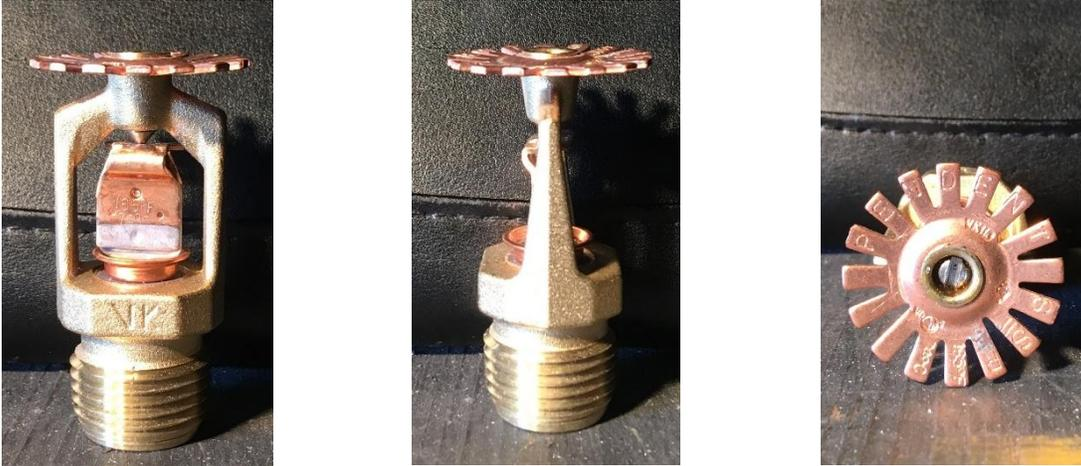
Figure 2-21: Ceiling-level sprinkler: K-factor 80 lpm/bar<sup>1/2</sup> (5.6 gpm/psi<sup>1/2</sup>), SR, Pendent, 74°C (165°F).
