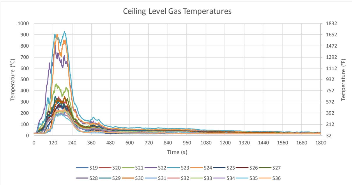
Figure B-2: Test 1 ceiling-level gas temperatures at TC locations 19-36.
