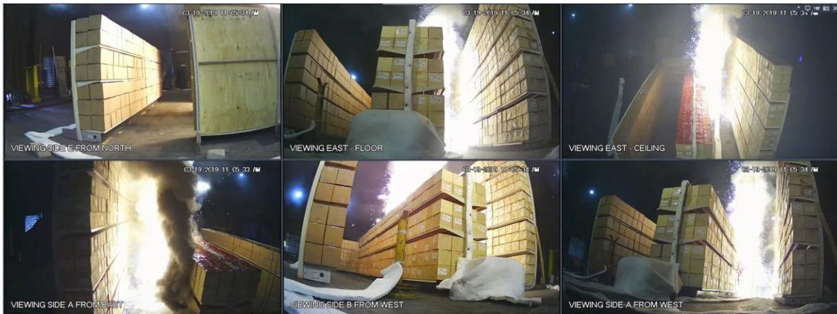
Figure A-22: Test 2 at 01:10: fire and smoke production intensifying in Side A.
