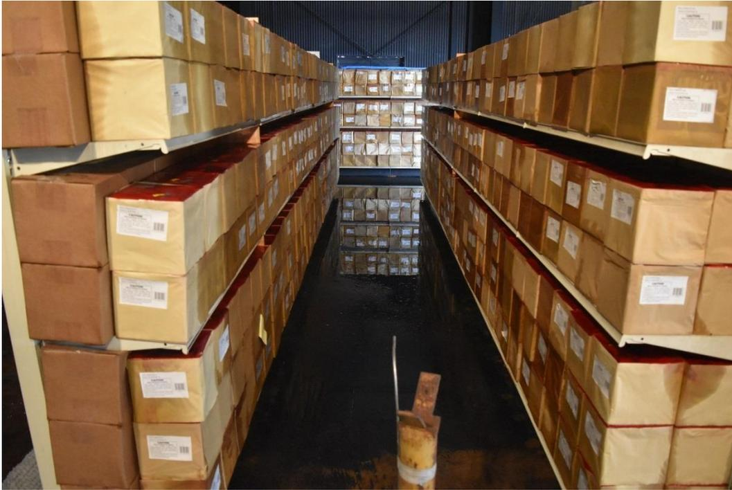
Figure C-13: Test 1 post-test image of Side B (right) and Side D (left) with Side E at the end of the aisle. These three shelving units sustained water damage only (no fire).
