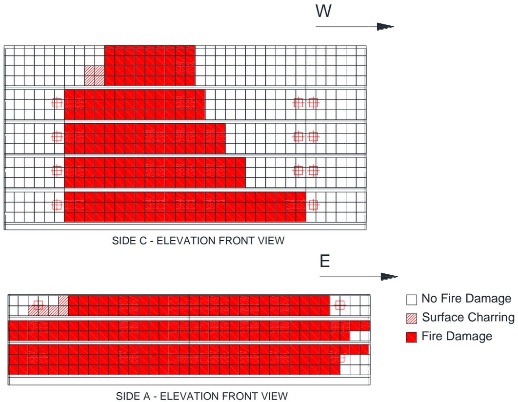
Figure 3-4: Test 1 elevation view of fire damage.
