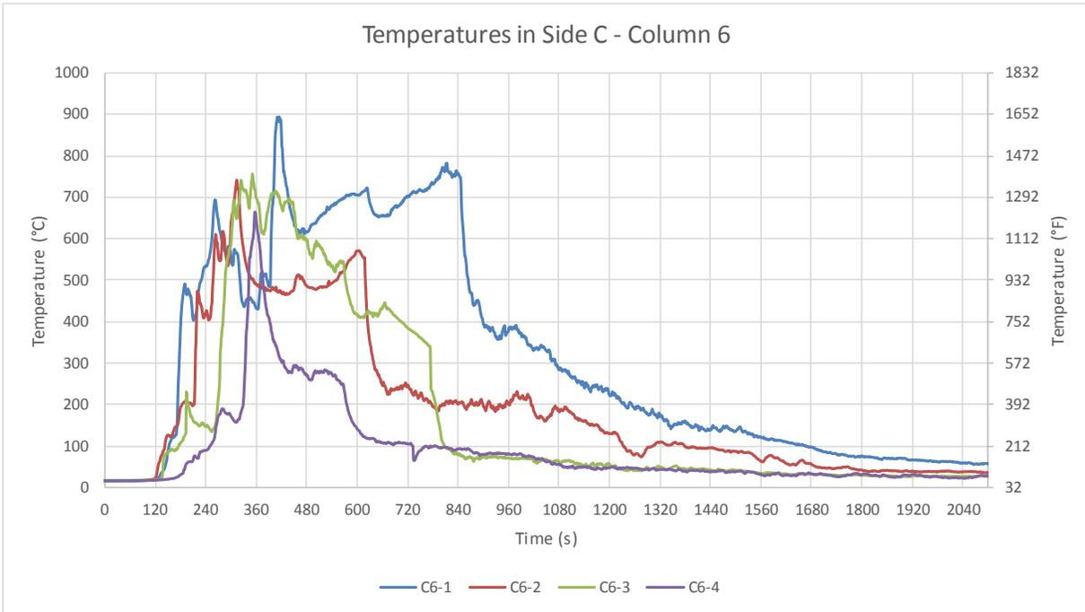
Figure B-25: Test 1 temperatures in Side C: Column 6.
