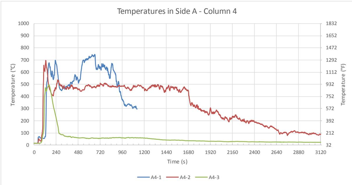
Figure B-39: Test 2 temperatures in Side A: Column 4. Note that TC A4 -1 malfunctioned during the test and suspect data have not been plotted. Its functionality was checked post-test and found to be inoperative.
