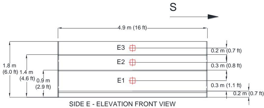
Figure 2-7: Front elevation view of Side E showing shelf height and thermocouple nomenclature and vertical dimensions of locations. Red crosses represent TCs.
