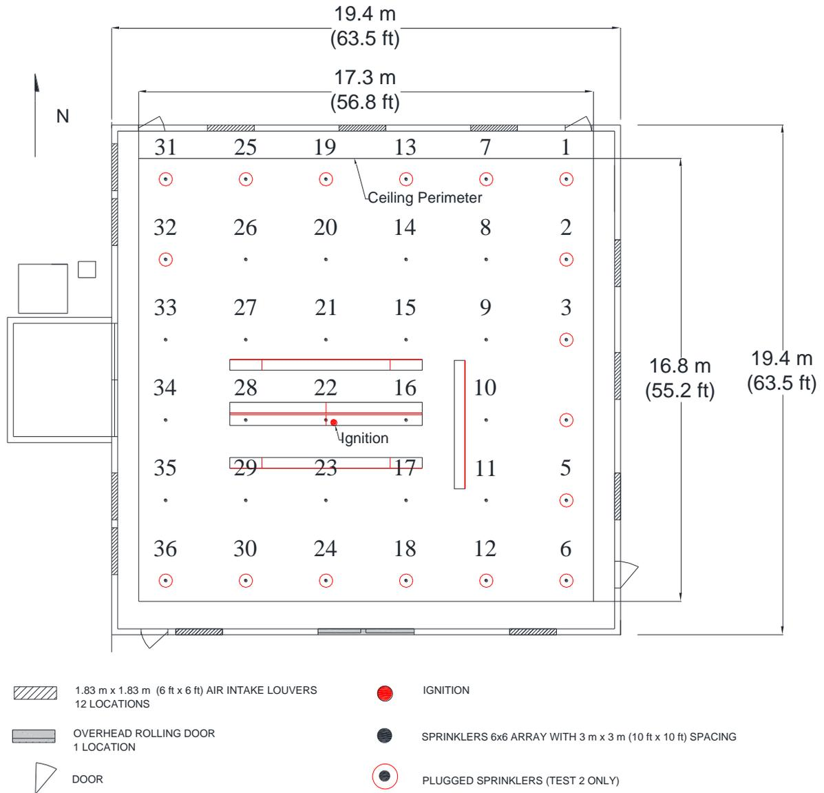
Figure 2-26: Plan view of test array and ceiling-level sprinklers within the laboratory space. Numbering above each sprinkler location is also associated with the TC at each location.
