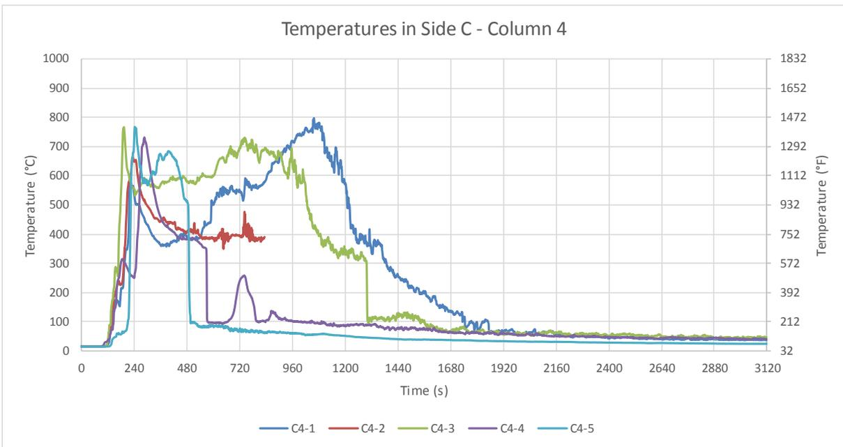
Figure B-52: Test 2 temperatures in Side C: Column 4. Note that TCs C4-1 and C4-2 malfunctioned during the test and suspect data have not been plotted. Their functionality was checked post-test and found to be inoperative.
