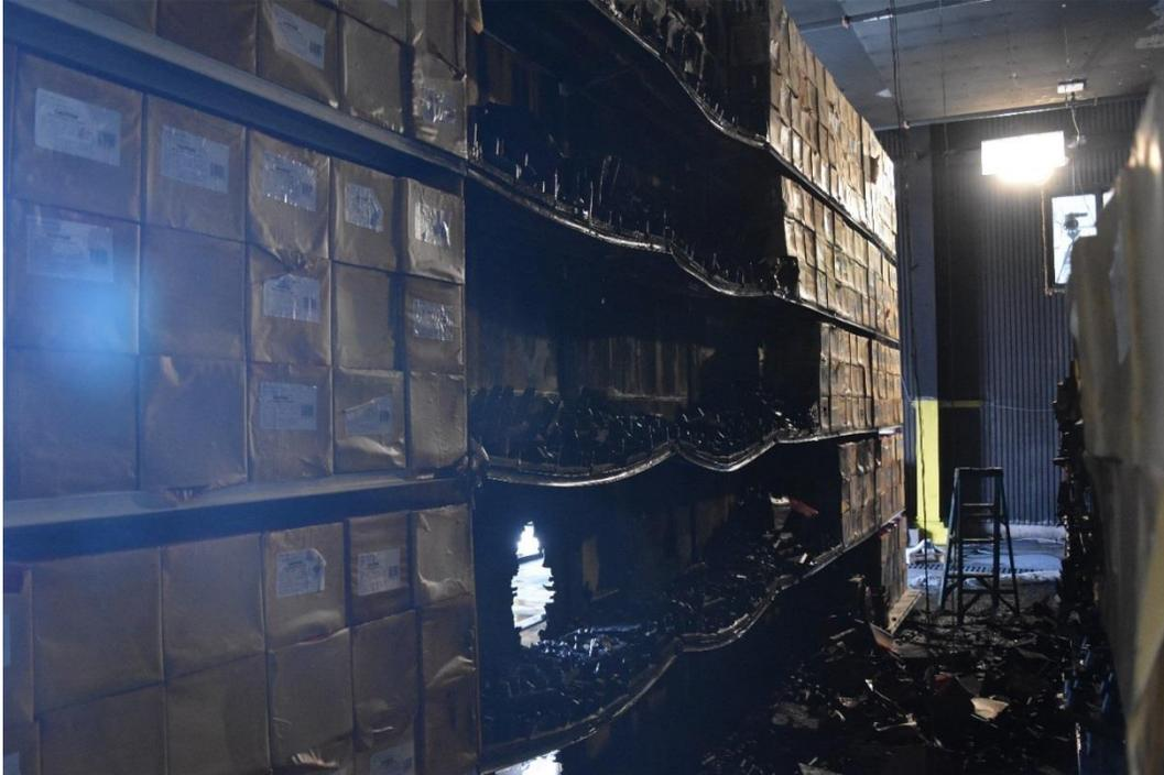
Figure C-7: Test 1 damage to Side C looking toward west. Transverse flame break located on left of image where commodity remains intact. Center of image shows burn through of longitudinal flame break (sheet rock backing remained intact at test conclusion and was removed post-test).
