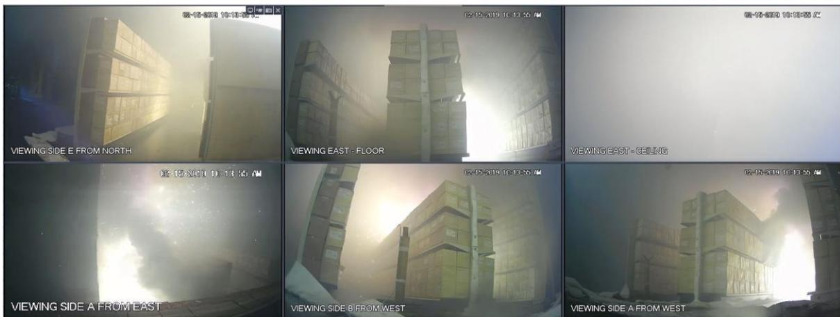
Figure A-11: Test 1 at 02:20: sprinklers continue to operate, ceiling-level gas temperatures (refer to Appendix B) are roughly steady state at maximum values.
