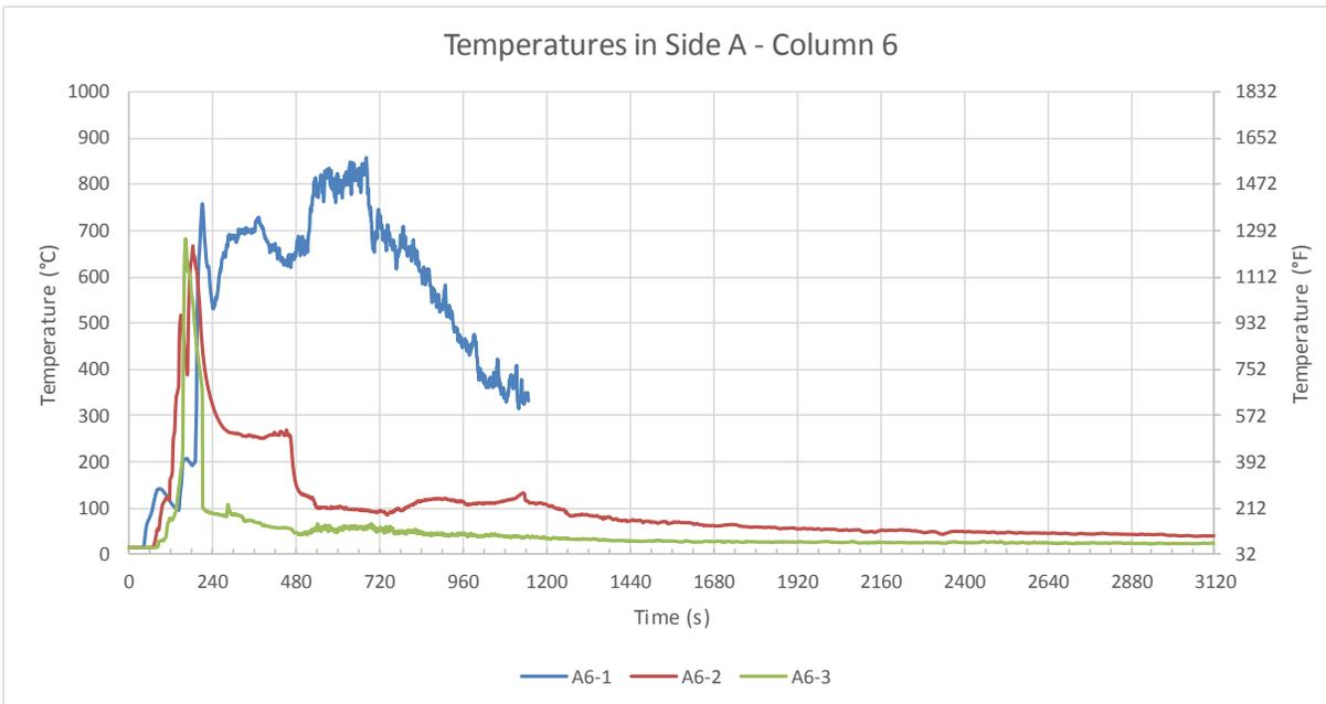
Figure B-41: Test 2 temperatures in Side A: Column 6. Note that TC A6-1 malfunctioned during the test and suspect data have not been plotted. Its functionality was checked post-test and found to be inoperative.
