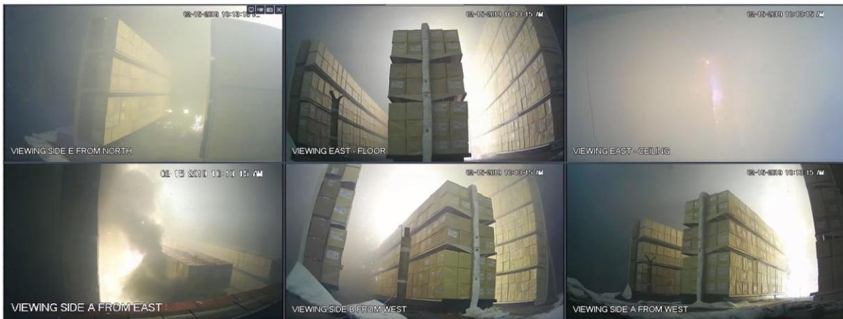
Figure A-7: Test 1 at 01:40: at least seven sprinklers operating, fire and smoke production intensifying. Side C ignited at 01:33, camera 1 showing sparks in aisle by Side E.
