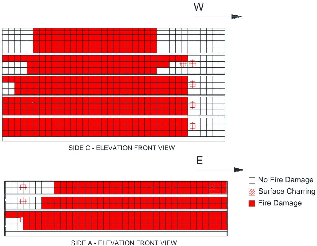
Figure 3-9: Test 2 elevation view of fire damage.
