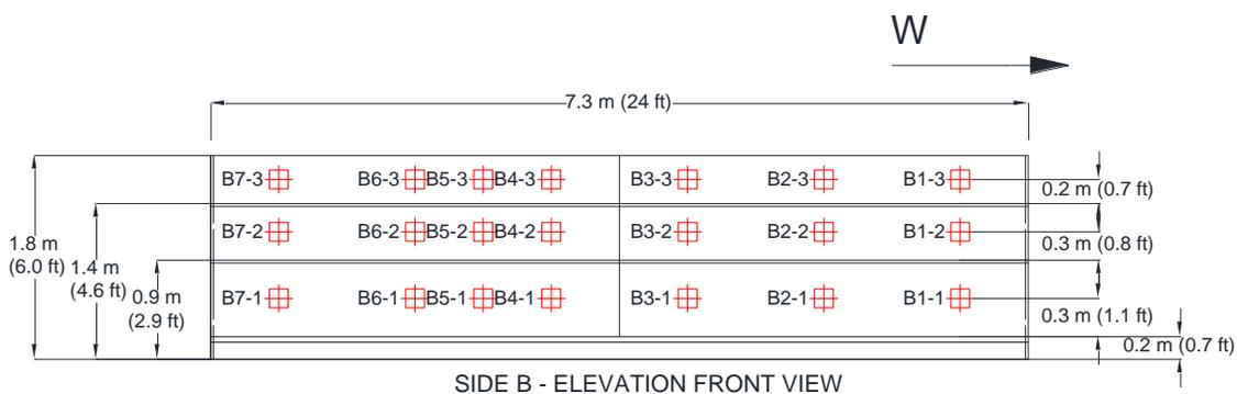
Figure 2-4: Front elevation view of Side B showing shelf height and thermocouple nomenclature and vertical dimensions of locations. Red crosses represent TCs.
