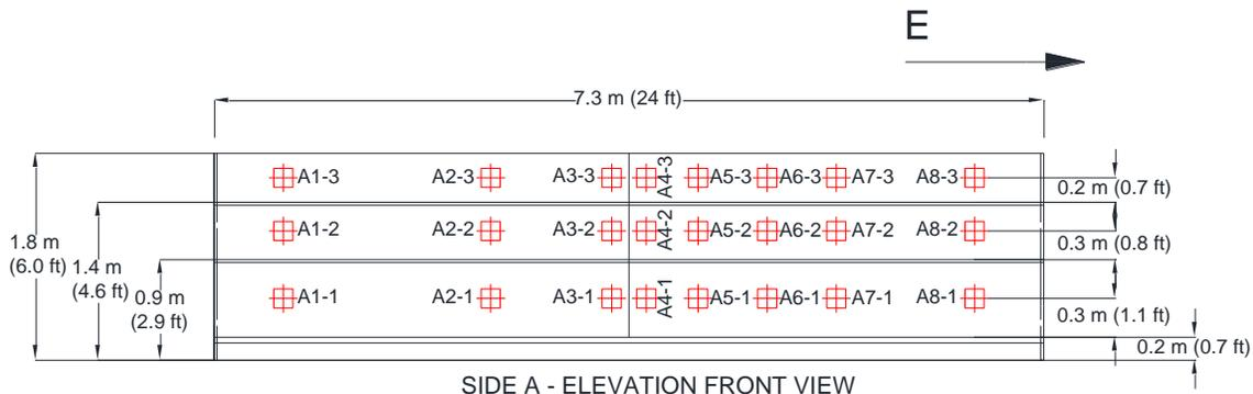
Figure 2-3: Front elevation view of Side A showing shelf height and thermocouple nomenclature and vertical dimensions of locations. Red crosses represent TCs.
