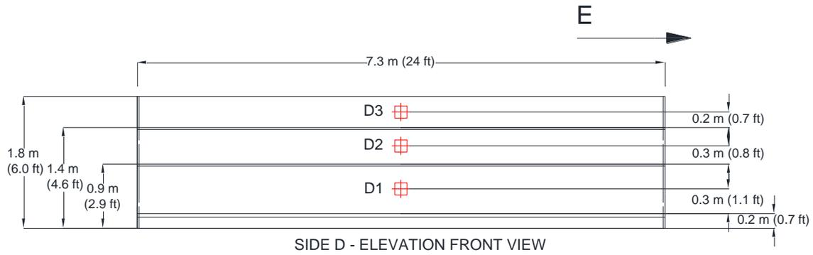
Figure 2-6: Front elevation view of Side D showing shelf height and thermocouple nomenclature and vertical dimensions of locations. Red crosses represent TCs.
