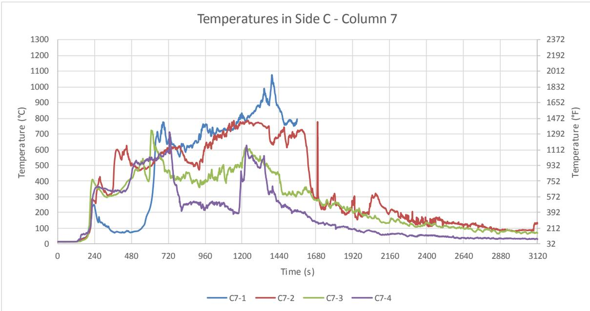
Figure B-55: Test 2 temperatures in Side C: Column 7. Note that TCs C7-1 and C7-2 malfunctioned during the test and suspect data have not been plotted. Their functionality was checked post-test and found to be inoperative.
