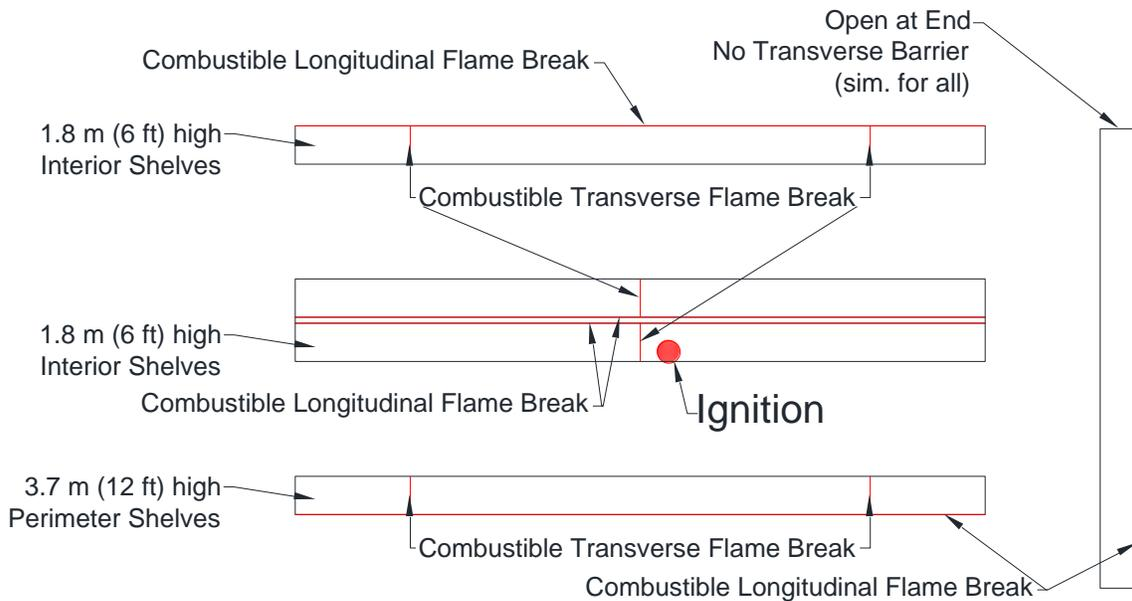
Figure 2-2: Plan view of shelving unit showing flame break locations.
