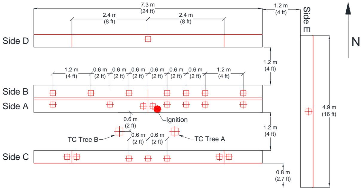
Figure 2-1: Plan view of shelving unit layout indicating nomenclature of sides and with thermocouple locations (red crosses).
