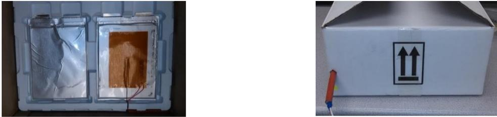
Figure 5-4: Photos of heater placement within ignition carton. Left photo shows a foil heater affixed to a battery on the fifth level (of ten levels) within the carton. Right photo shows the heater wiring exiting the carton.
