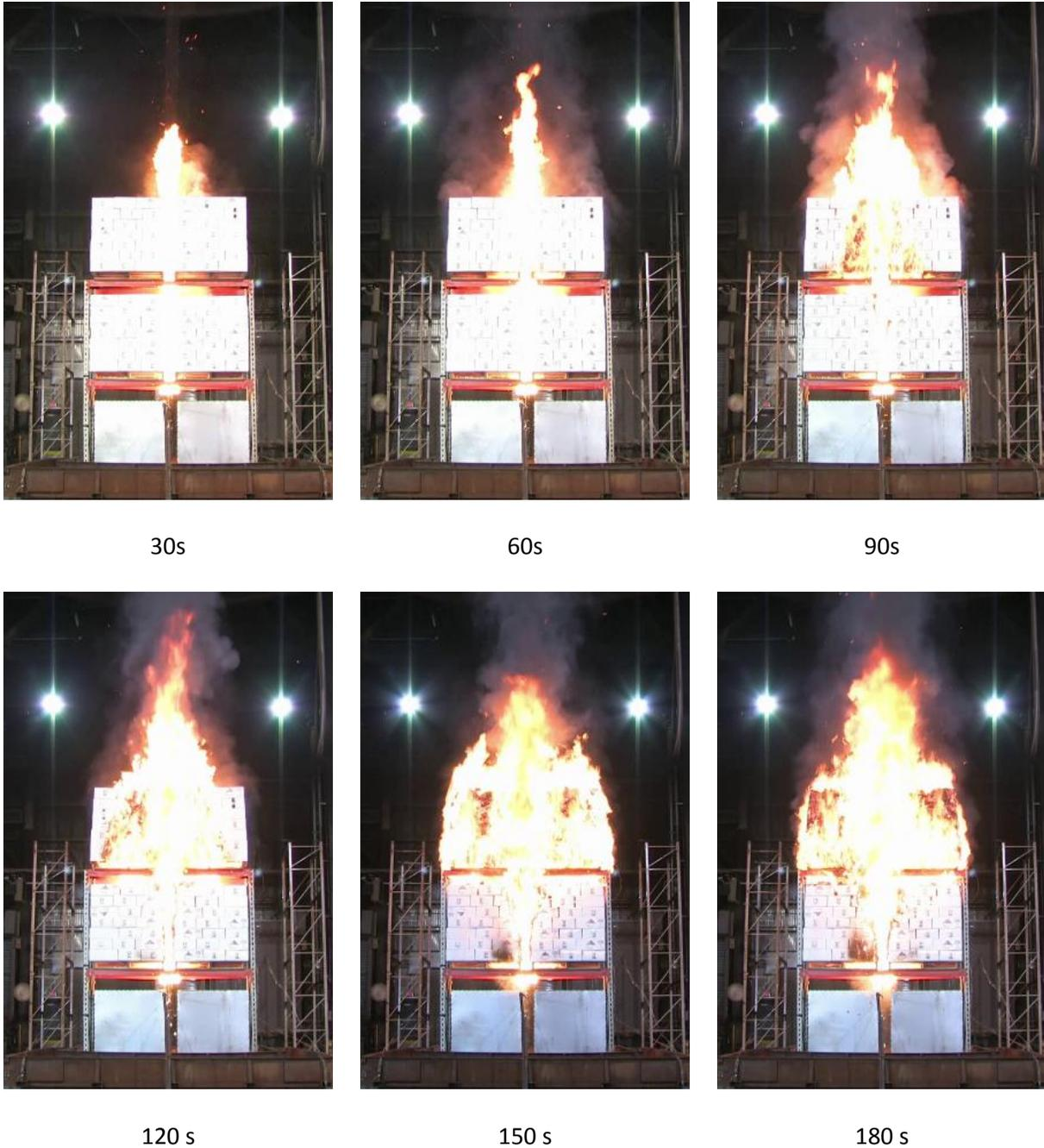
Figure 3-7: Test images shown in 30 s increments from ignition for the large-format polymer pouch batteries.
