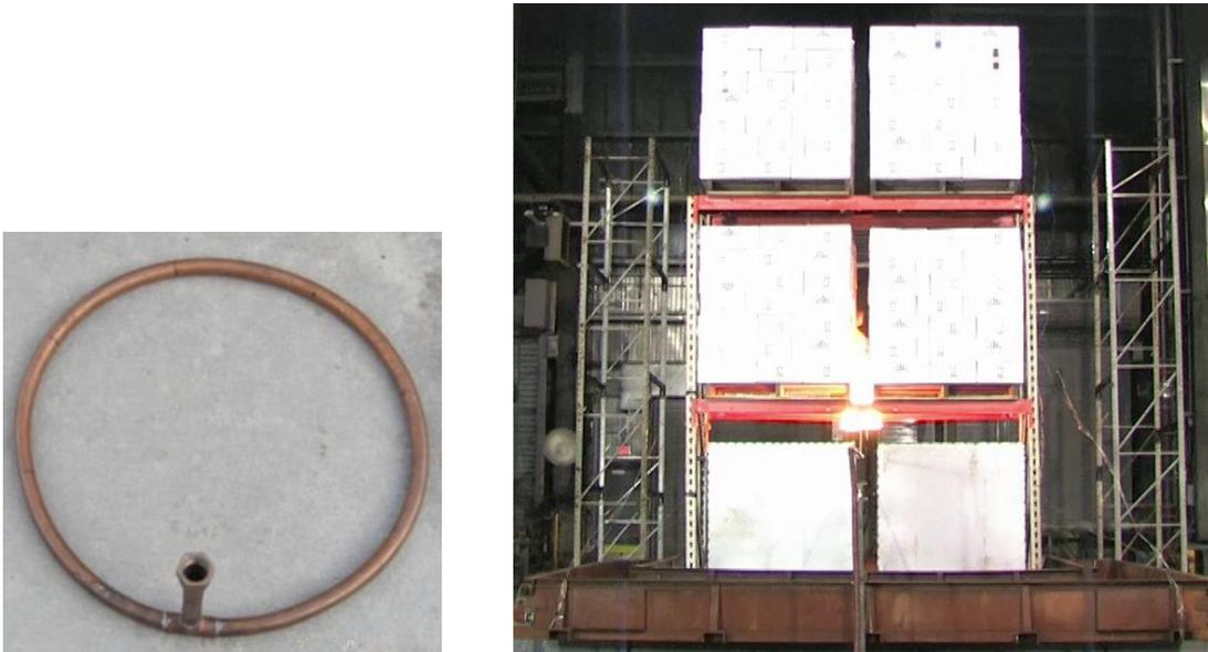
Figure 3-2: Propane ring burner (left) within the rack and fire size within rack (right).
