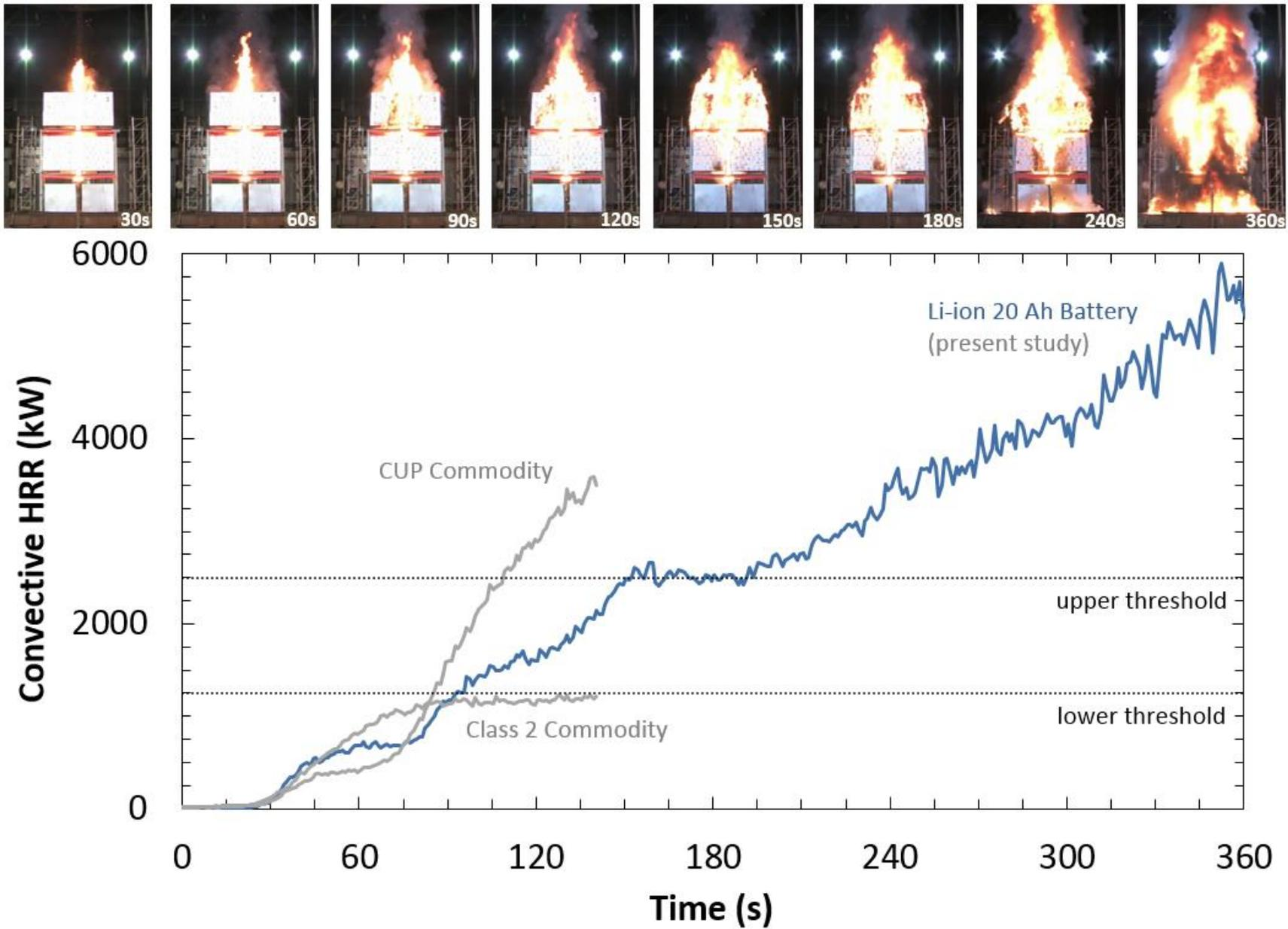
Figure 3-10: Determination of the time of battery involvement.
