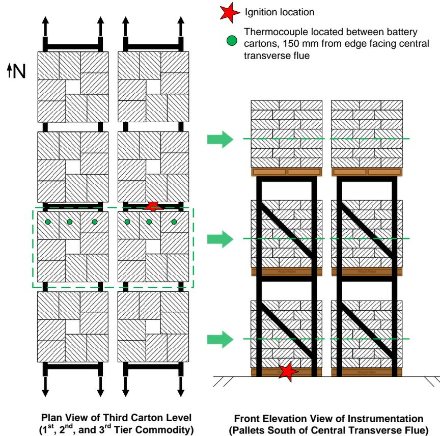
Figure 4-4: Thermocouple locations used during the large-scale test.
