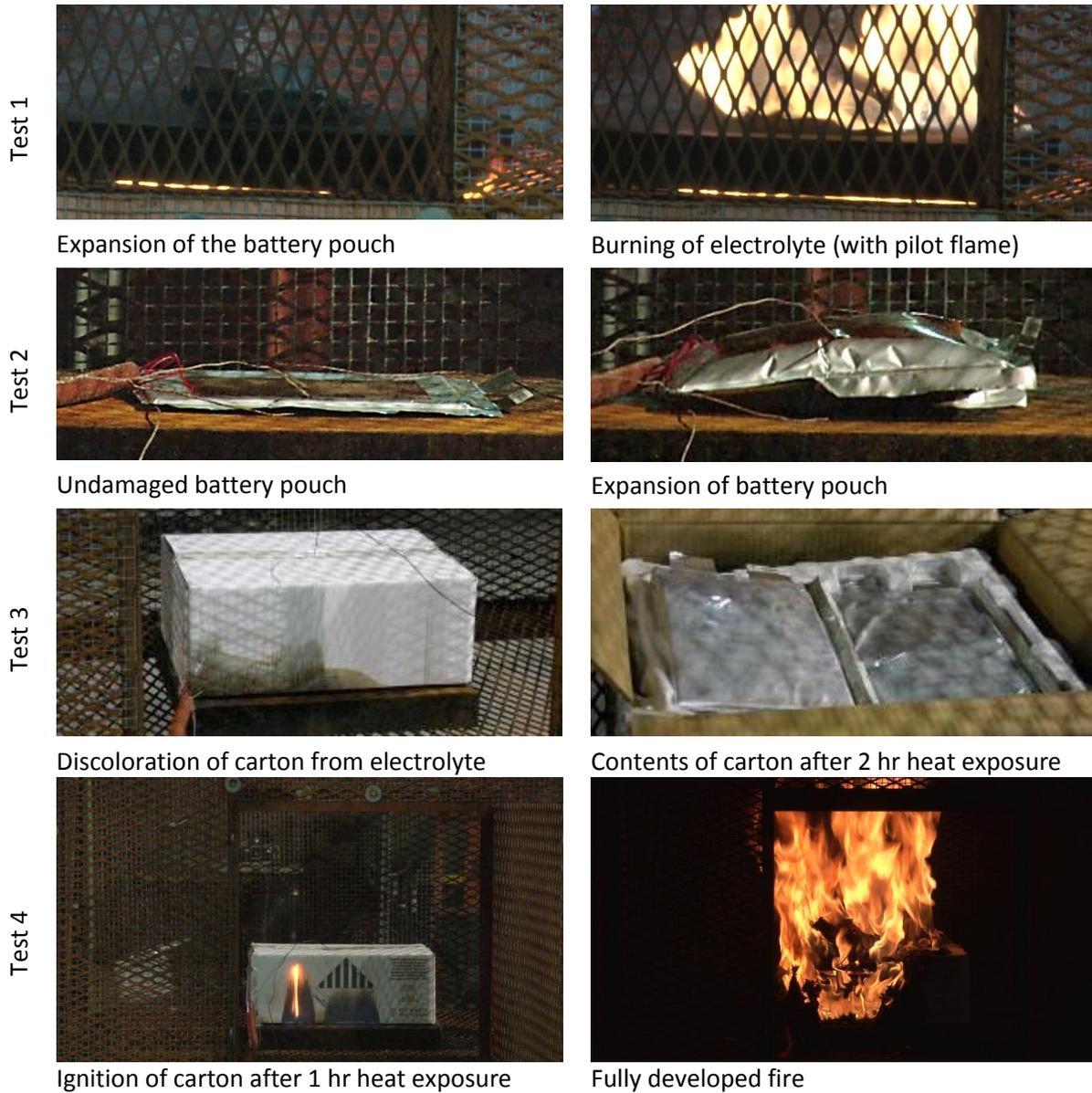
Figure 5-1: Photos of internal ignition evaluation tests.
