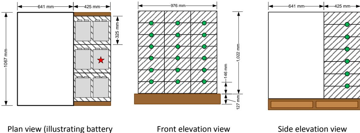
Figure 5-2: Intermediate-scale suppression test pallet design. The location of the ignition battery is identified with a red star and TC locations are shown with green circles.
