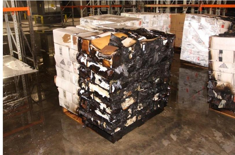
**Pallet load from second tier ignition flue**
