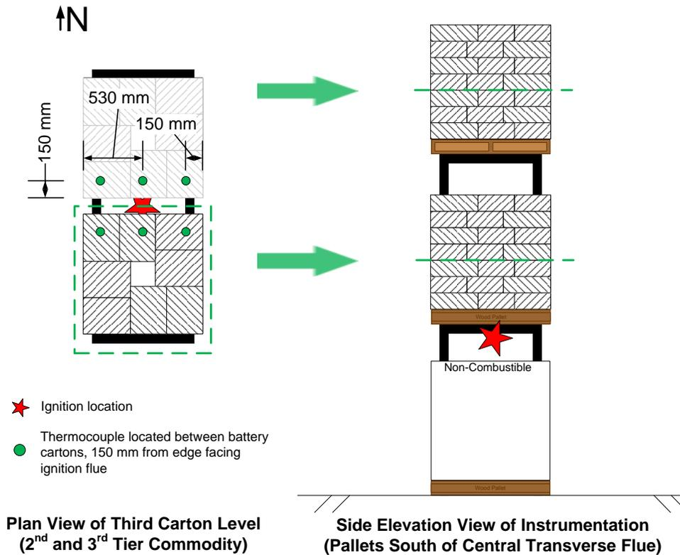
Figure 3-3: Thermocouple locations used during the reduced-commodity test.
