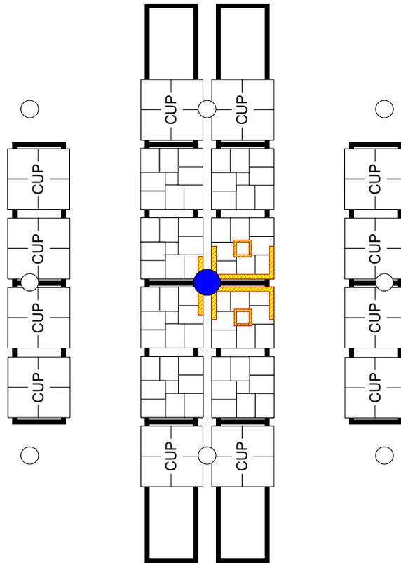
Figure 4-9: Sprinkler operation pattern and commodity damage.
