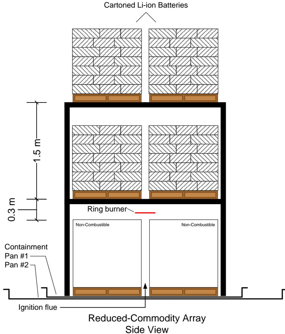
Figure 3-1: Elevation view of reduced-commodity test rack.
