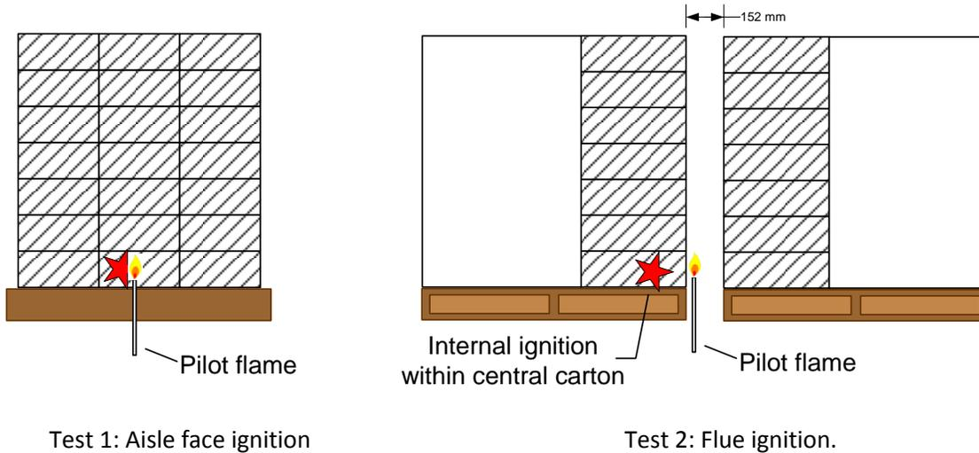
Figure 5-3: Intermediate-scale suppression test ignition location. The location of the carton containing the ignition battery is identified with a red star.
