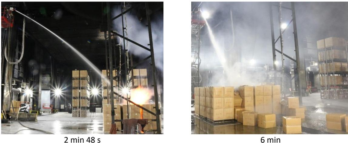
Figure 2-40: AWC Test 5 fire development at 2 min and 48 s and at 6 min from ignition.
