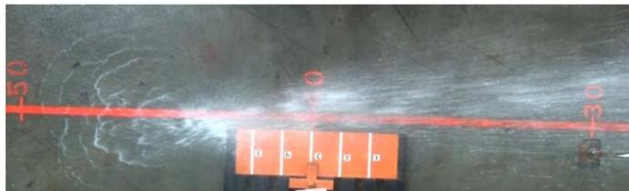
Figure 2-22: AWC test layout used to measure stream trajectory.
