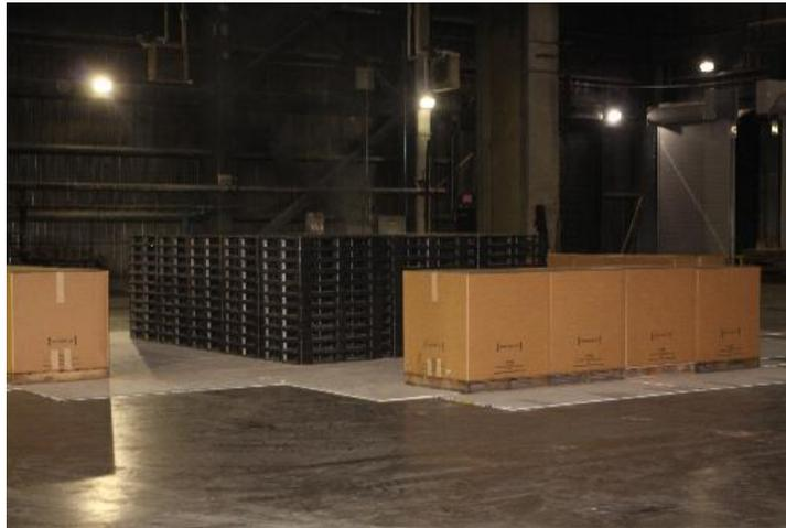
Figure 2-3: SMART sprinkler test setup with low-piled storage of UUP.
