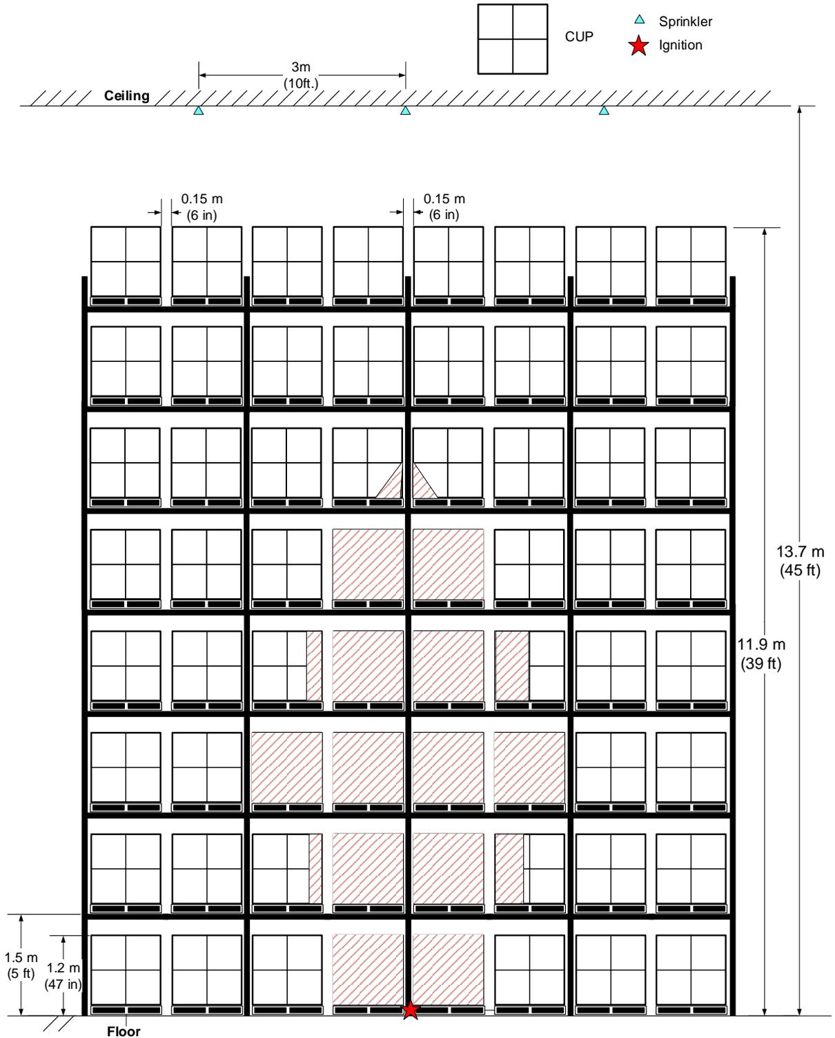
Figure 3-10: SMART sprinkler high-bay rack-storage Test 1 fire damage to east side of main array represented by red hatch marks.
