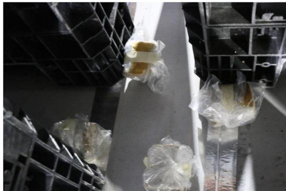
Figure 4-3: Ignitor placement for open-top container tests.
