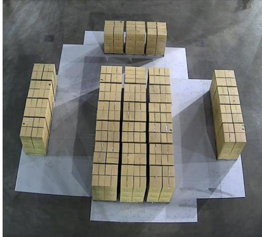
Figure 2-1: SMART sprinkler test setup with low-piled storage of CUP or CEP.
