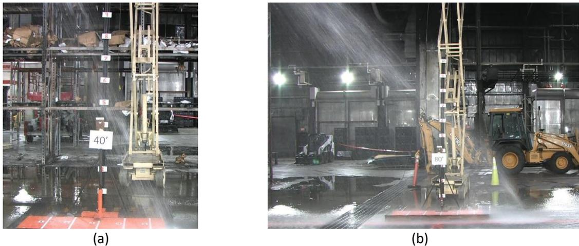
Figure 2-25: AWC stream trajectory at (a) 230 lpm (60 gpm), and (b) 450 lpm (120 gpm) with  $H_0 = 15$  m (50 ft),  $\theta = 0^\circ$ , and  $\alpha = 0^\circ$ .
