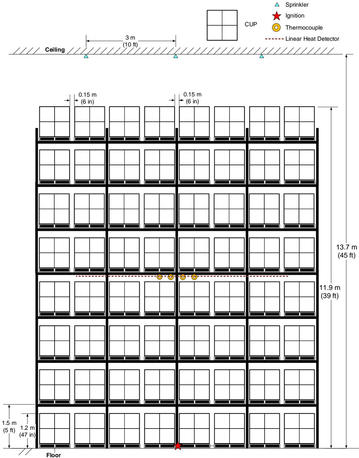
Figure 3-2: Elevation view of SMART sprinkler protection of high-bay rack-storage Test 1 main array using eight tiers of CUP under a 13.7 m (45 ft) ceiling.
