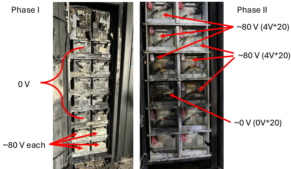
Figure 3-7: Images of the unit of origin and measured voltages after tests, left: Phase I test, right: Phase II test.
