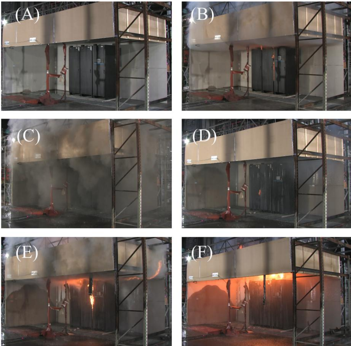
Figure D-1: Representative images of the Phase I fire test: (A) pretest, (B) at approximately 17 minutes flames emerge from the top surface and door seams of the initiating unit, (C) sprinkler activation at around 24 minutes, (D) ~29 minutes, reignition is observed with flames emerging from the initiating unit, (E) ~40 minutes, fire size increases and flames emerge from the partially open side walls, (F) ~42 minutes, fire heating damaged the ceiling structure, causing partial ceiling collapse, and flames emerge from the top of the room.
