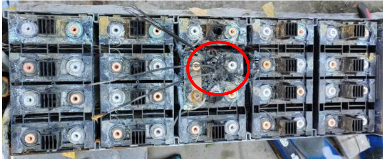
Figure 2-2: Post-test image of the initiating module [3].
