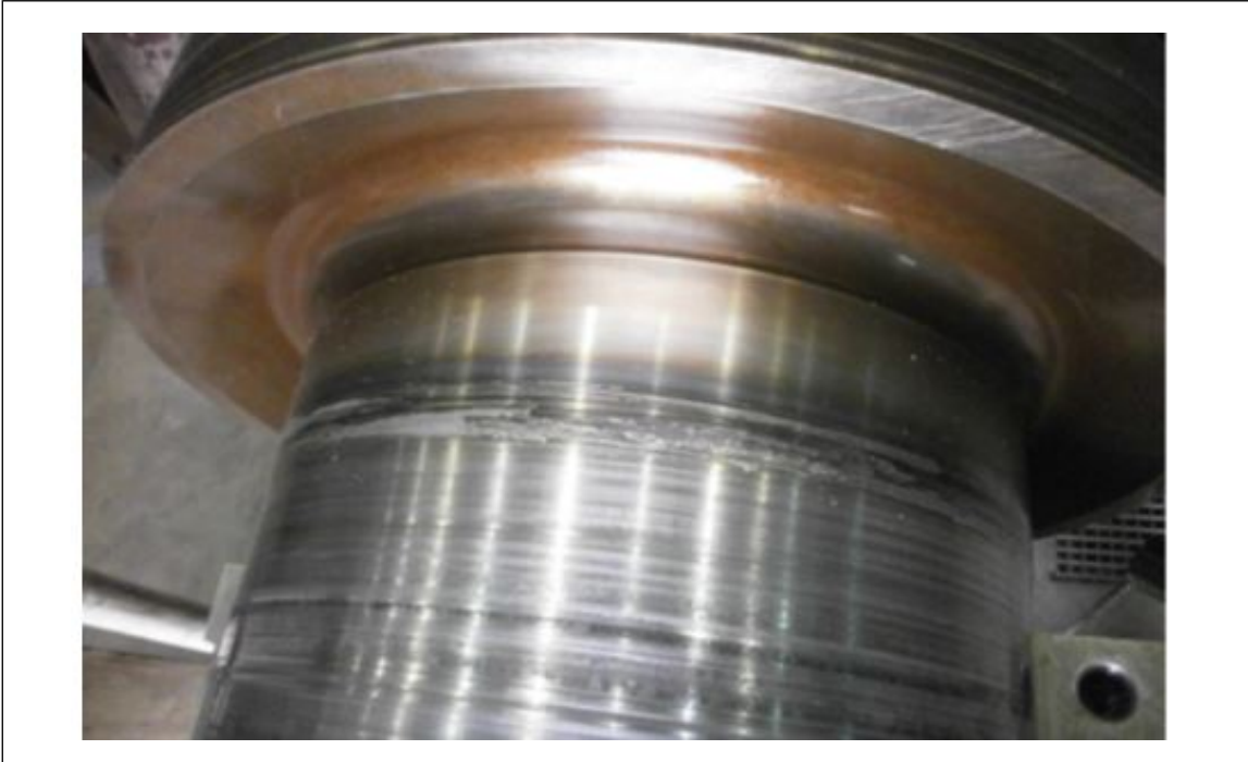
Fig. 4. Rotor journal scoring
