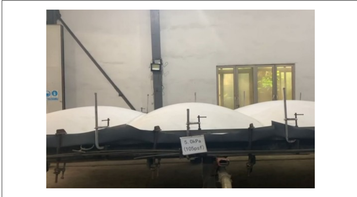
Fig. 3.4.1-1. Mechanically fastened roof cover billowing when subjected to wind pressure
