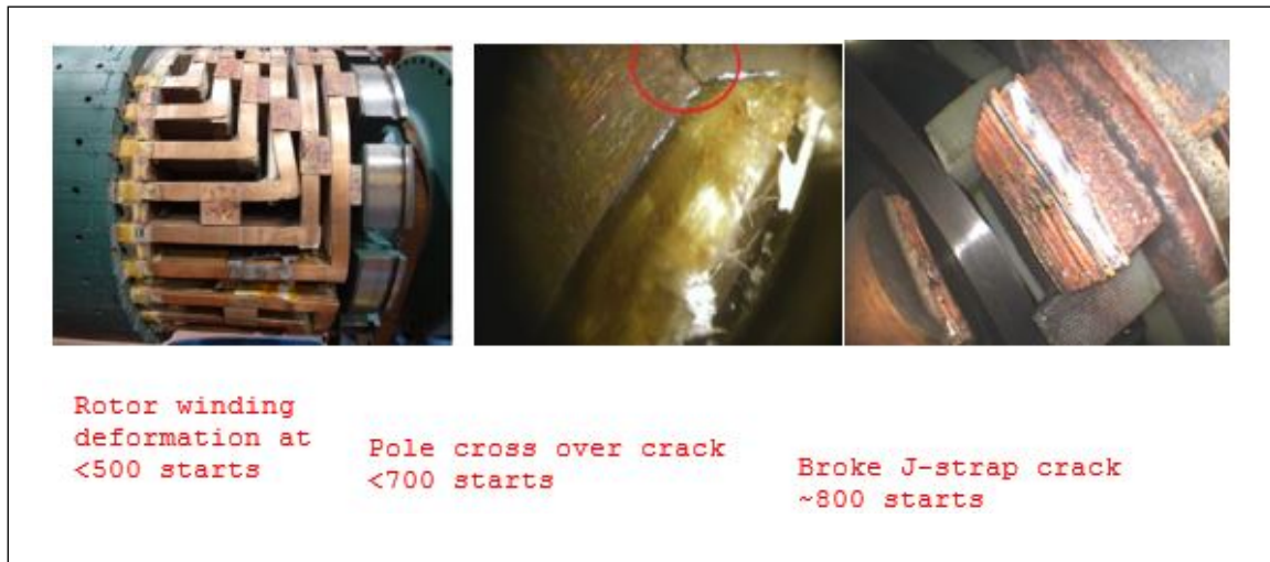
Fig. 3. Examples of generator rotor related losses due to excessive load cycling
