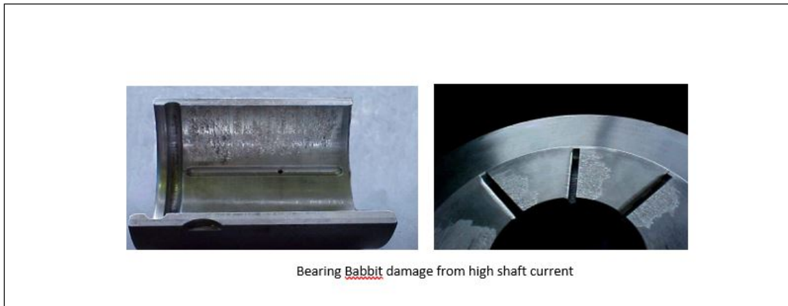
Fig. 4. Examples of damage caused by high level of shaft current (photos courtesy of J. E. Timperley)
