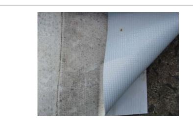
Fig. 3.5.2-4. Roof cut from hail-damaged roof in Figures 3.5.2-1 and 3.5.2-2
