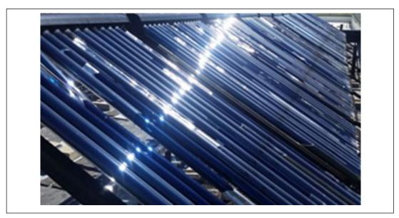
Fig. 3.4.1-1. Glass tube solar heat exchanger damaged by 1.5 in. (38 mm) diameter hail
