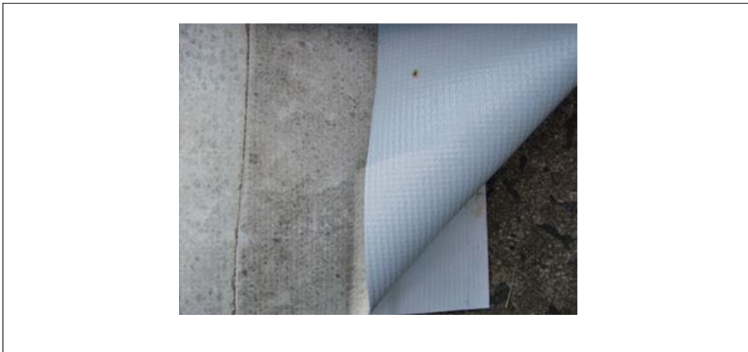
Fig. 3.5.2-4. Roof cut from hail-damaged roof in Figures 3.5.2-1 and 3.5.2-2
