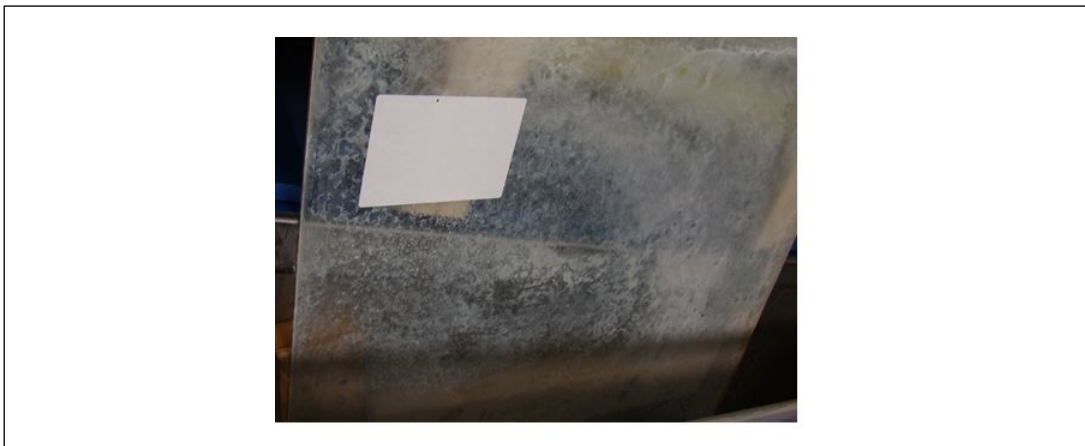
Fig. 3.2.1-4. Weathered greenhouse roof glass panel
