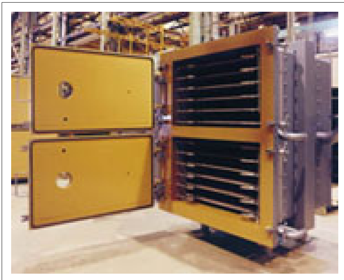
Fig. 1. Batch tray dryer
