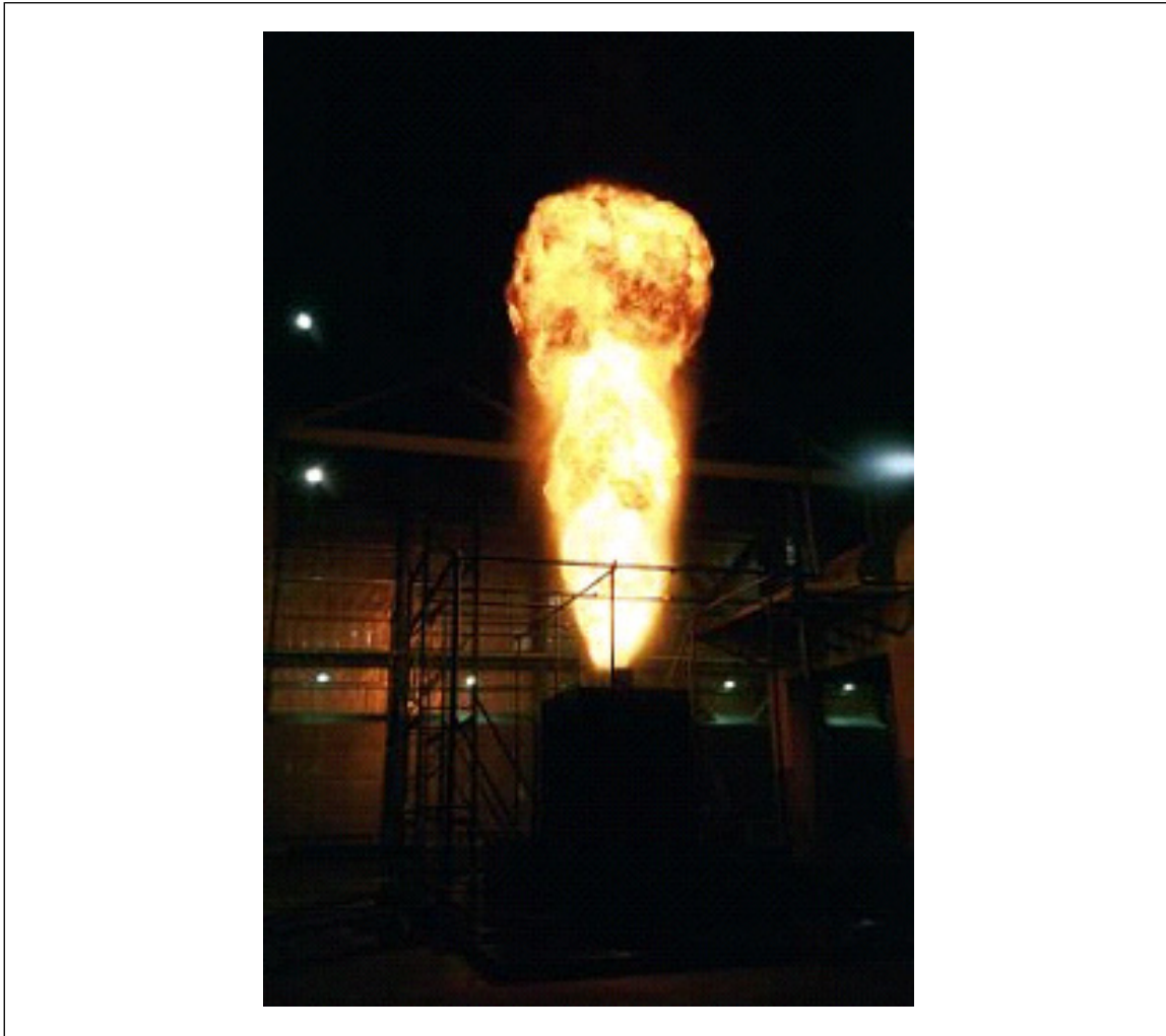
Fig. 3.1.3. Mineral oil spray fire (90 psig [6 barg]) demonstration test performed by FM
