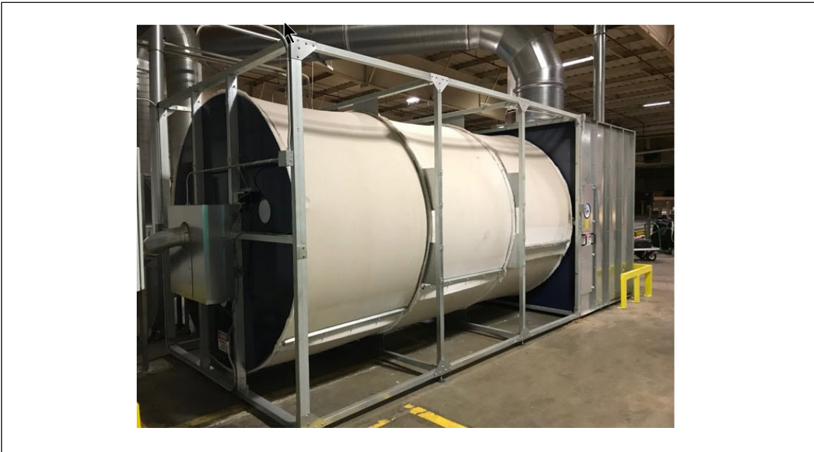
Fig. 3.4.1.2-1. Example of an enclosureless drum filter
