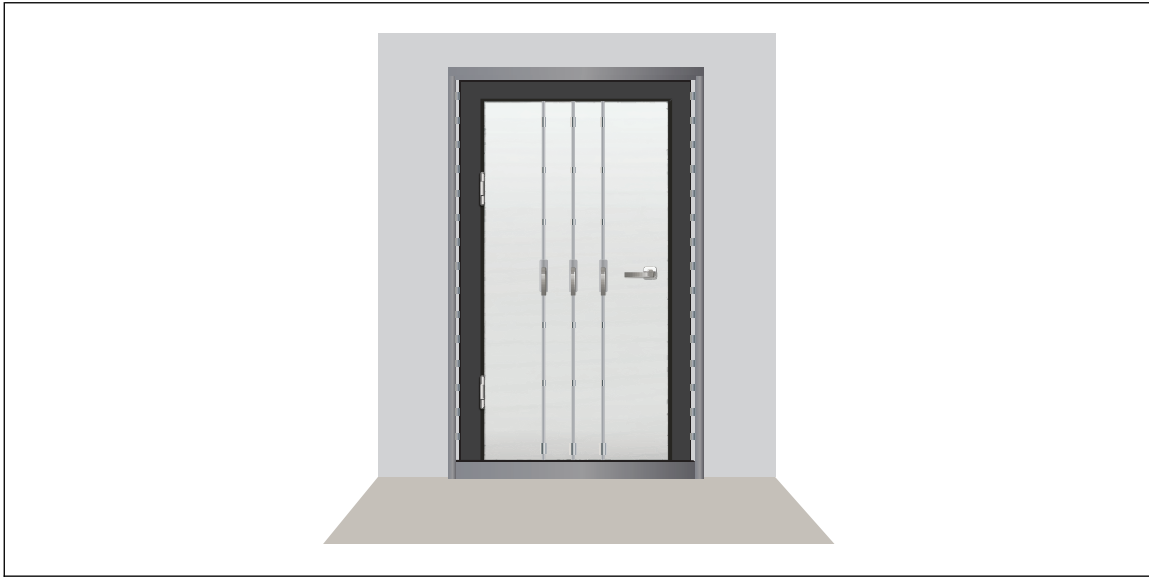
Fig. 3.7.4.2-1. Personal flood door inside – this door has additional vertical latches that must be manually deployed
