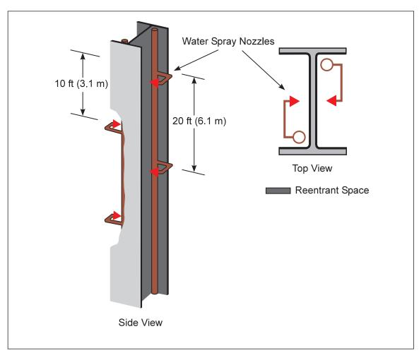
Fig. E.1.B. Water spray protection for steel columns
