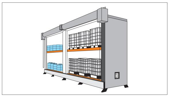
Fig 2.2.3.3. Ignitable liquid storage locker
