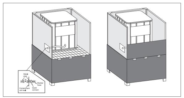
Fig. 2.2.3.1. Storage container for IBC
