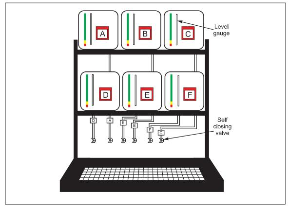
Fig. 2.5.1.13. Metal container dispensing arrangement
