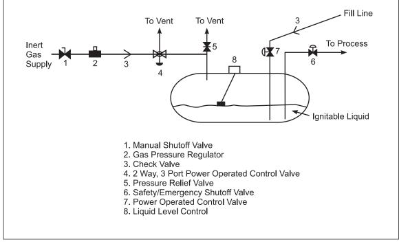
Fig. 2.5.4.3.4. Compressed inert-gas transfer method
