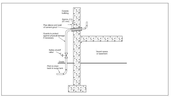
Fig. 2.2.4.7.A. Preferred arrangement for above-grade pipe entrance into building
