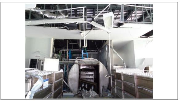
Fig. 29. Autoclave after the steam explosion
