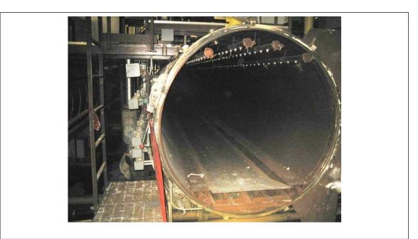
Fig. 27. Autoclave front seal area with remains of locking rings
