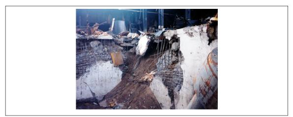
Fig. 1. Collateral damage following catastrophic failure of a hot isostatic press
