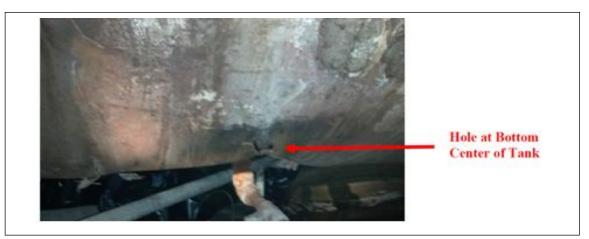
Fig. 8. Photograph of failure location at center of tank
