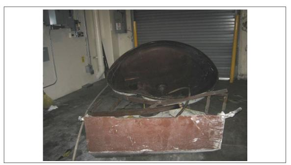
Fig. 28. Autoclave door that failed and separated from the autoclave
