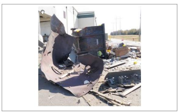
Fig. 12. The deaerator after colliding with the dumpster; part of one head is attached to the shell (the other head went out the front of the boiler room)
