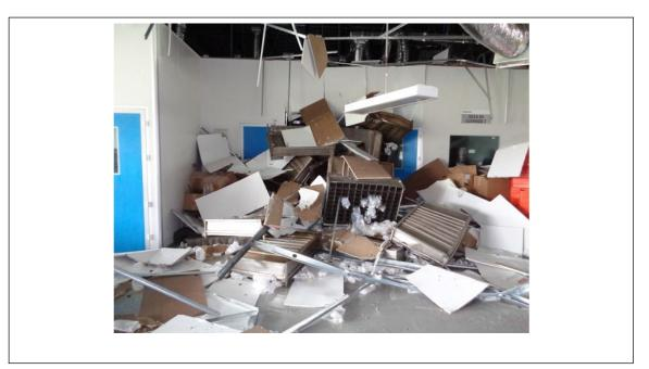
Fig. 30. Autoclave door and internal trays that were propelled 50 ft (15.2 m) across the room
