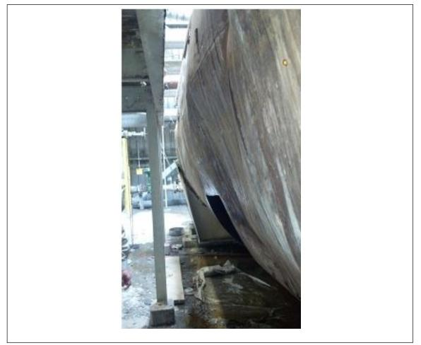
sizes appearing to fish mouth inwardly. All adjacent piping and instrumentation were damaged. Photographs of the damage to the deaerator are provided in Figures 7 through 9.
