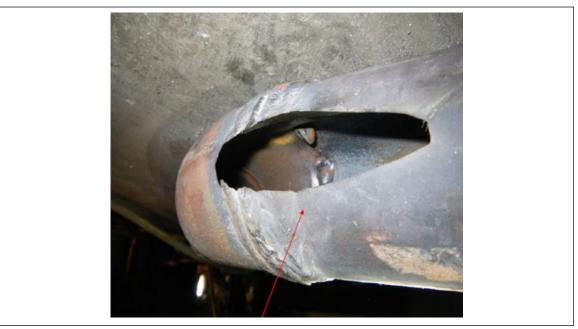
Fig. 6. Solid particle erosion at a change in direction led to the failure of this pipe at a power generating station
