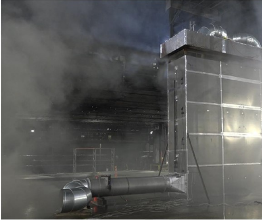
Fig. 3.3.4.3.1-3. Smoke generation post sprinkler activation from the stocker setup
