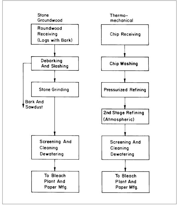
Fig. 1. Flowchart of alternative mechanical pulping techniques.
