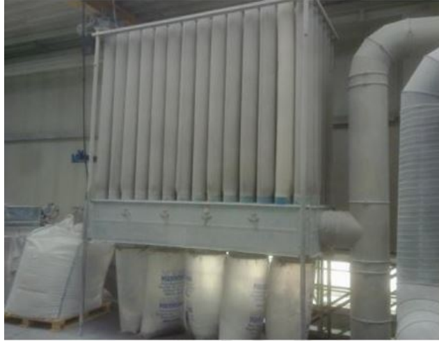
Fig. 3.4.1.1-1. Example of an enclosureless collector
