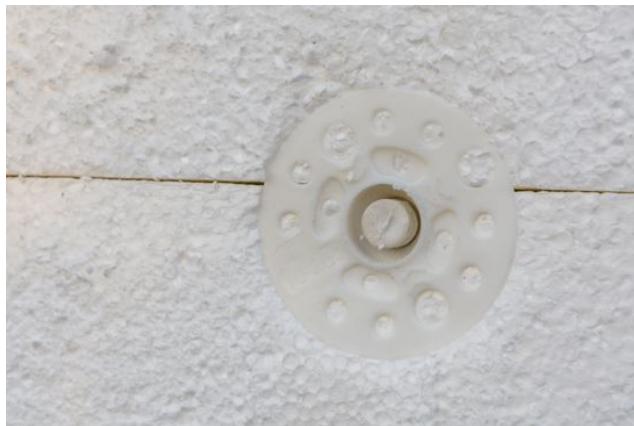
Fig. 3.2.1.1-2. Expanded Polystyrene Foam Core Example (usually white in color)
