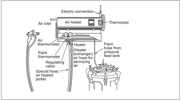
Fig. 10. Hot spraying system; this type heats both atomizing air and coating material
