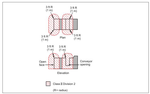
Fig. 8. Class II, Division 2 area equipment adjacent to a closed-top, open-face, or open-front spray booth
