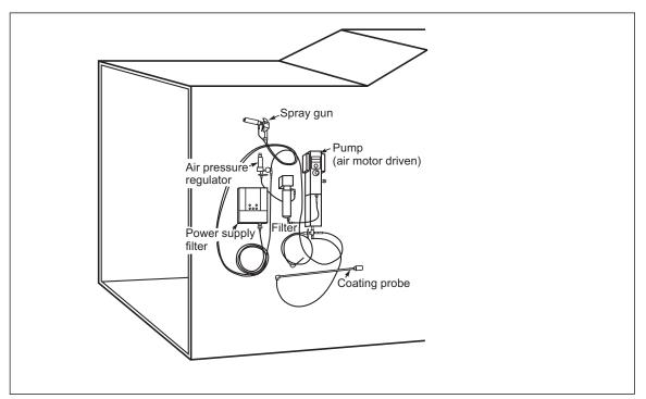
Fig. 11. Airless electrostatic spray system
