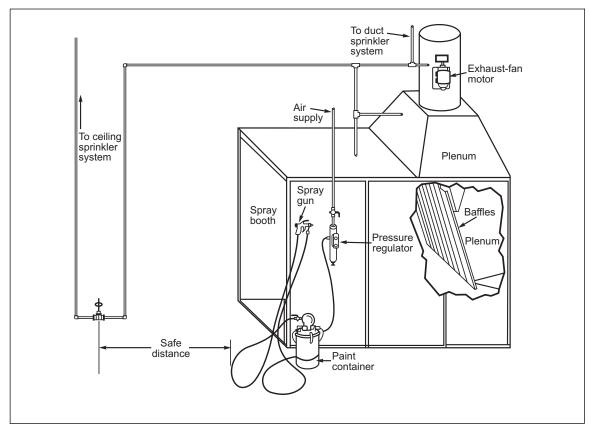
Fig. 12. Dry filter spray booth equipped with baffles
