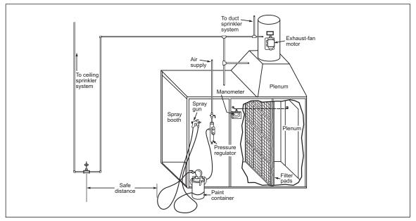
Fig. 3. Dry filter (open-face) spray booth equipped with filter pads; gauge used to indicate minimum air velocity is also shown
