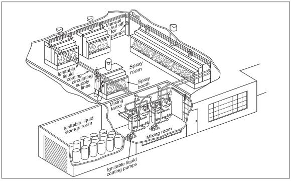
Fig. 1. Spray room with water wash spray booths, cut-off ignitable liquid mixing room, ignitable liquid distribution system and cut-off ignitable liquid storage room (sprinkler protection and automatically actuated remote shutoff for pumps not shown)
