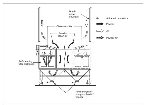
Fig. 15. Integrated booth design with cartridge filter system in upper part of booth hopper
