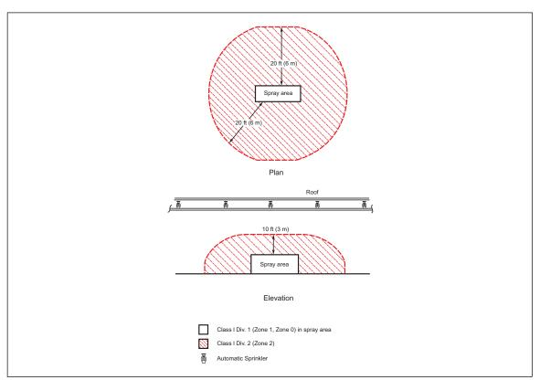
Fig. 5. Class I Division 2 (Zone 2) areas adjacent to an unenclosed spray operation
