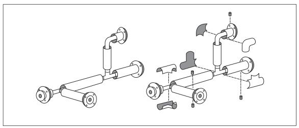
Fig. C.1.3-1. Prefabricated jacketed section
