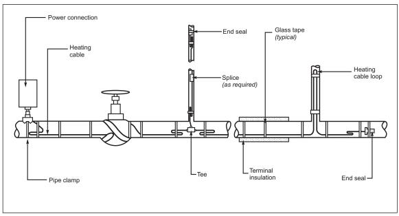
Fig. C.1.1-1. Typical heat tracing system
