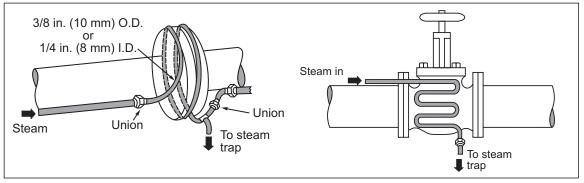
Fig. C.1.5-1. Steam tracer on a flange, on a straight pipe and a valve
