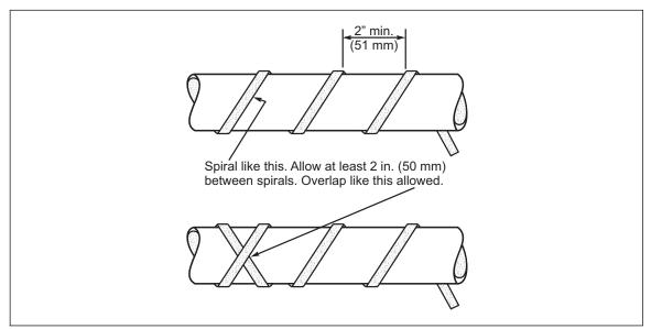
Fig. C.1.2-1. Installation of self-regulating heating cable
