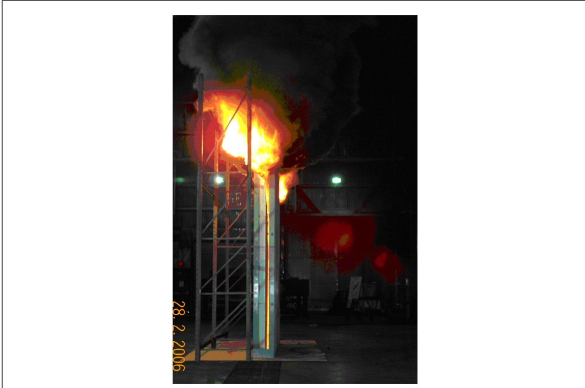
Fig. 3.3-1. Fire Test of cavity wall assembly using foam polystyrene insulation
