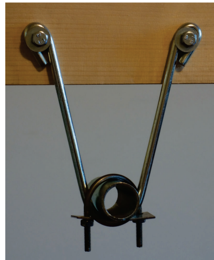
U-hanger with U-bolt retainer preventing upward movement
