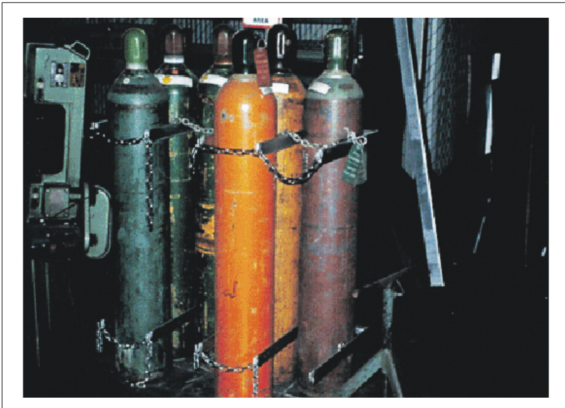
Fig. 2.3.2.1B. Example of multiple cylinder restraint arrangement
