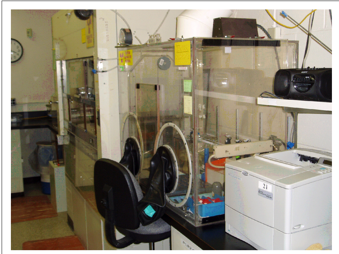
Fig. 4 Plastic enclosure containing a Class A combustible and an ignitable solvent
