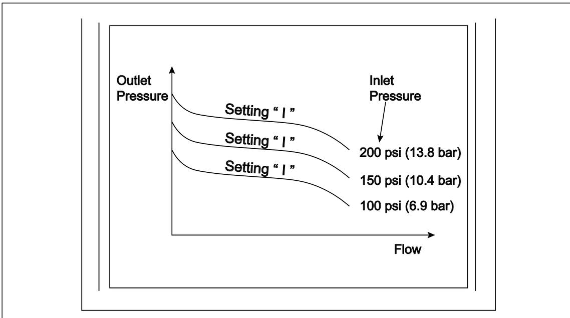
Fig. 3.3.1-2. Flow chart showing plot of outlet pressure versus flow rate through the valves for a given inlet pressure range
