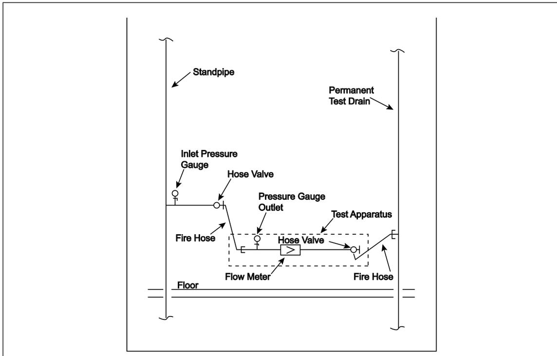
Fig. 2.3.6.1-1. Arrangement of annual full flow test on valves used in hose connections
