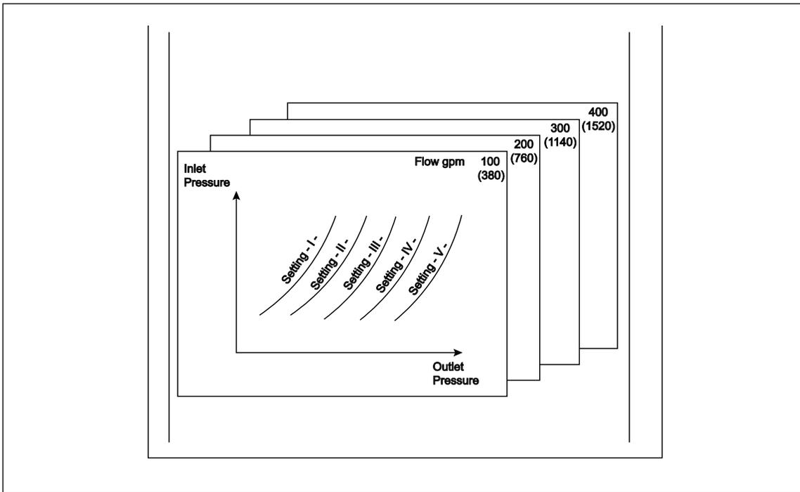
Fig. 3.3.1-1. Flow chart showing pot of outlet pressure versus inlet pressure for a given flow rate.
