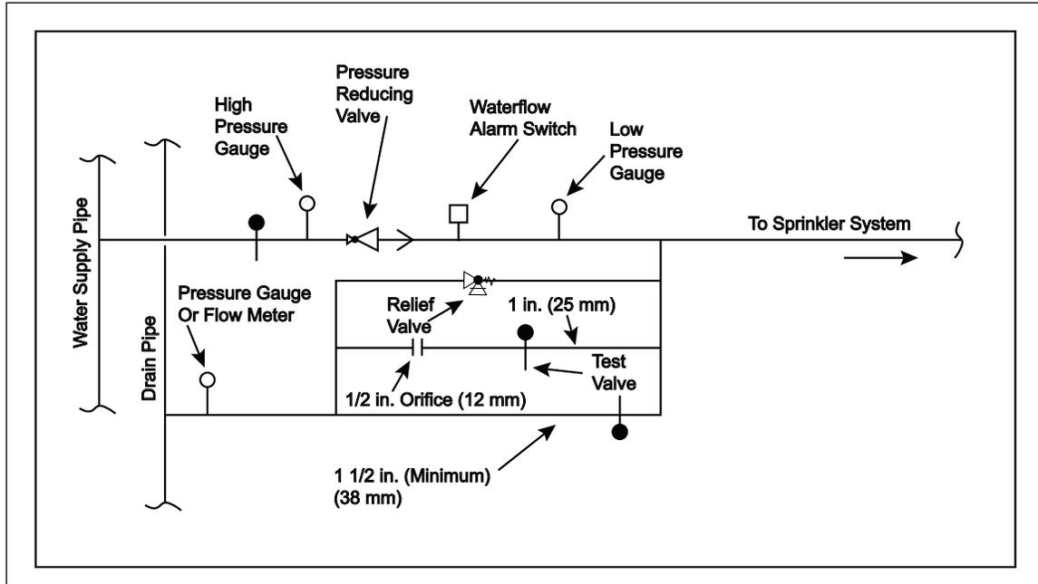
Fig. 2.3.5.1-1. Pressure reducing valve installation for individual sprinkler system (Note: A check valve is not needed for pressure reducing valves that have a check valve function incorporated in their design.)
