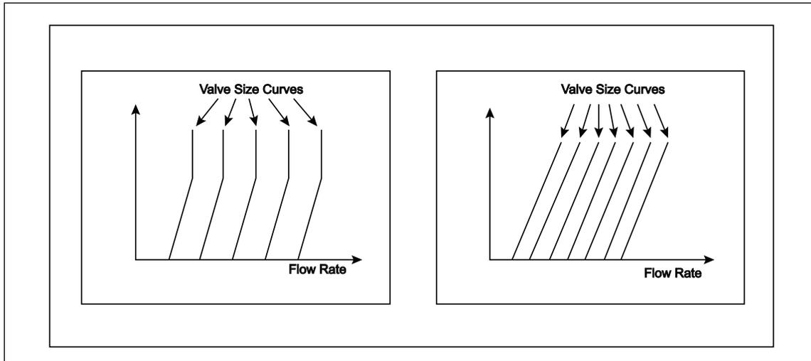
Fig. 3.3.2-1. Flow sizing graphs showing plot of maximum pressure drop across valve as a function of flow rate
