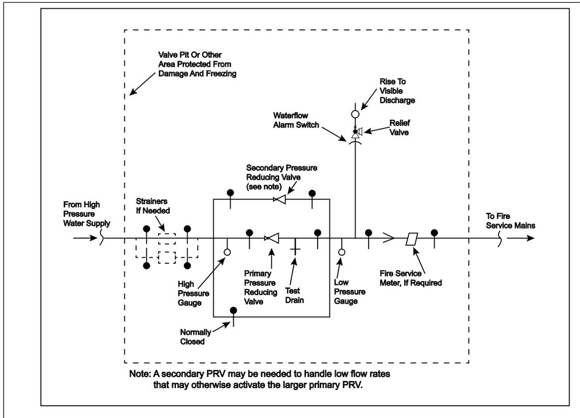
Fig. 2.3.4.6-1. Arrangement of pressure reducing valve for fire service
