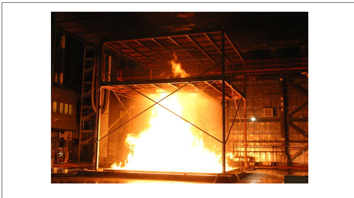
Fig. 3.2.1.2.1. Process structure test, ethanol fire in 25 ft x 25 ft (7.6 m x 7.6 m) pan with one level of sprinklers
