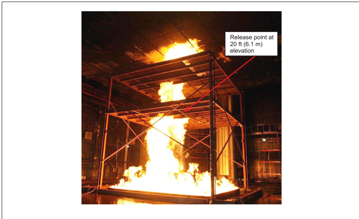
Fig. 3.2.1.2.2-2. Three-dimensional spill fire before sprinkler activation (22 gpm [83 L/min] ethanol flow rate)
