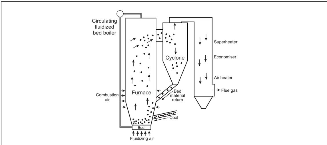
Fig. 7. Circulating fluidized bed boiler with hot cyclone
