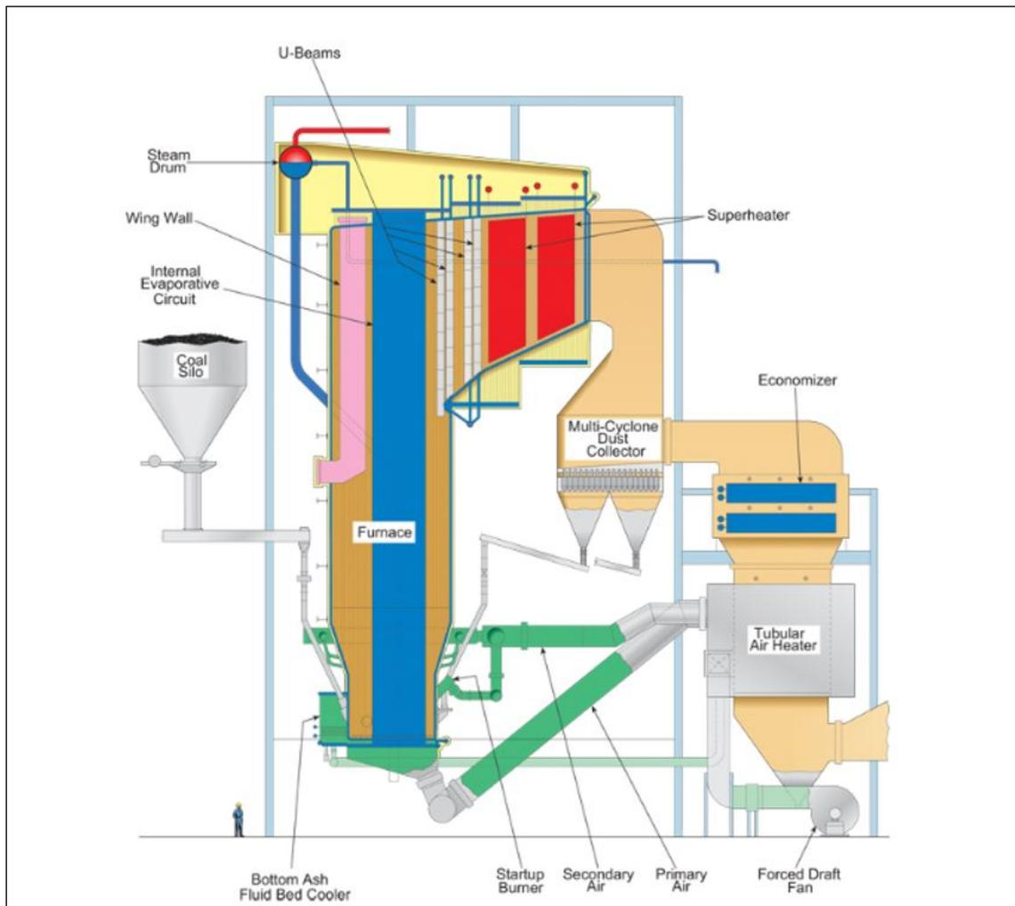
Fig. 8. Circulating fluidized bed boiler with U-Beam bed recirculation system (courtesy of the Babcock & Wilcox Co.)
