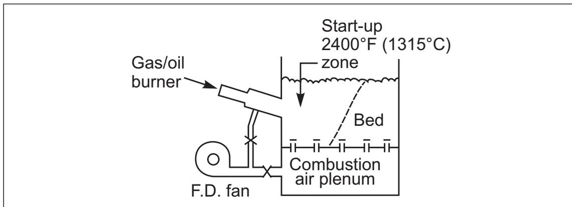
Fig. 4. Internal bed heater
