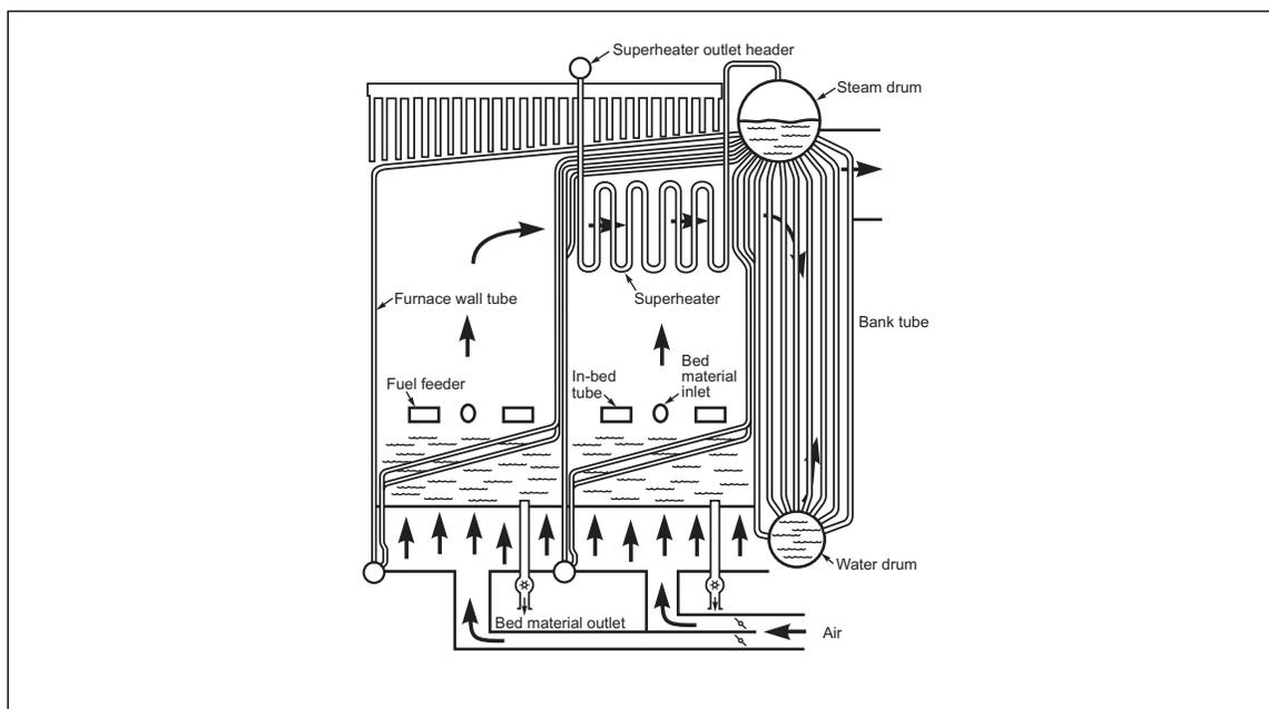
Fig. 5. Bottom-supported bubbling fluidized bed boiler
