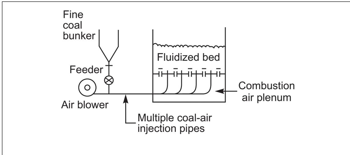
Fig. 9. In-bed solid fuel feed, pneumatic injection
