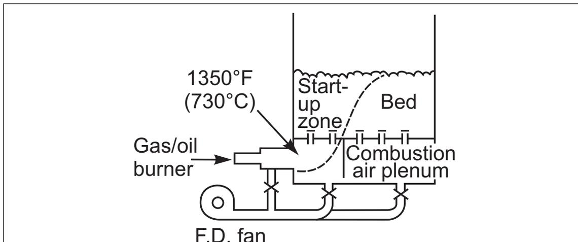
Fig. 3. Internal plenum heater
