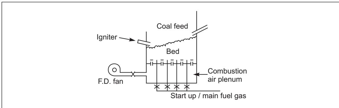
Fig. 1. Burn-in bed, surface ignitor
