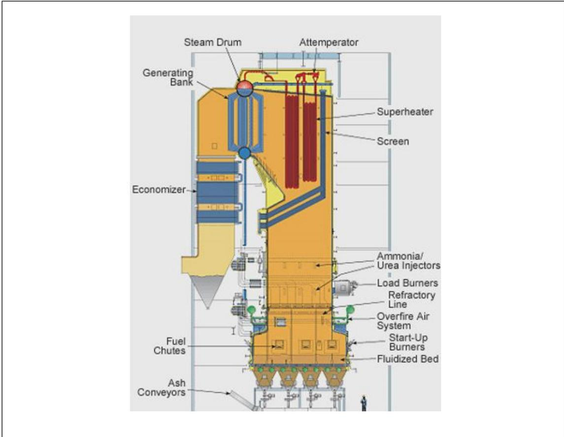
Fig. 6. Top supported bubbling fluidized bed boiler (courtesy of the Babcock & Wilcox Co.)
