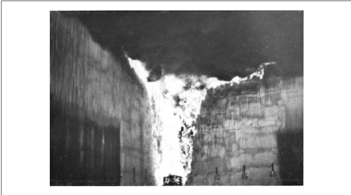
Fig. 21. FM corner test (This polyurethane was rated “self extinguishing” by a small-scale test.)
