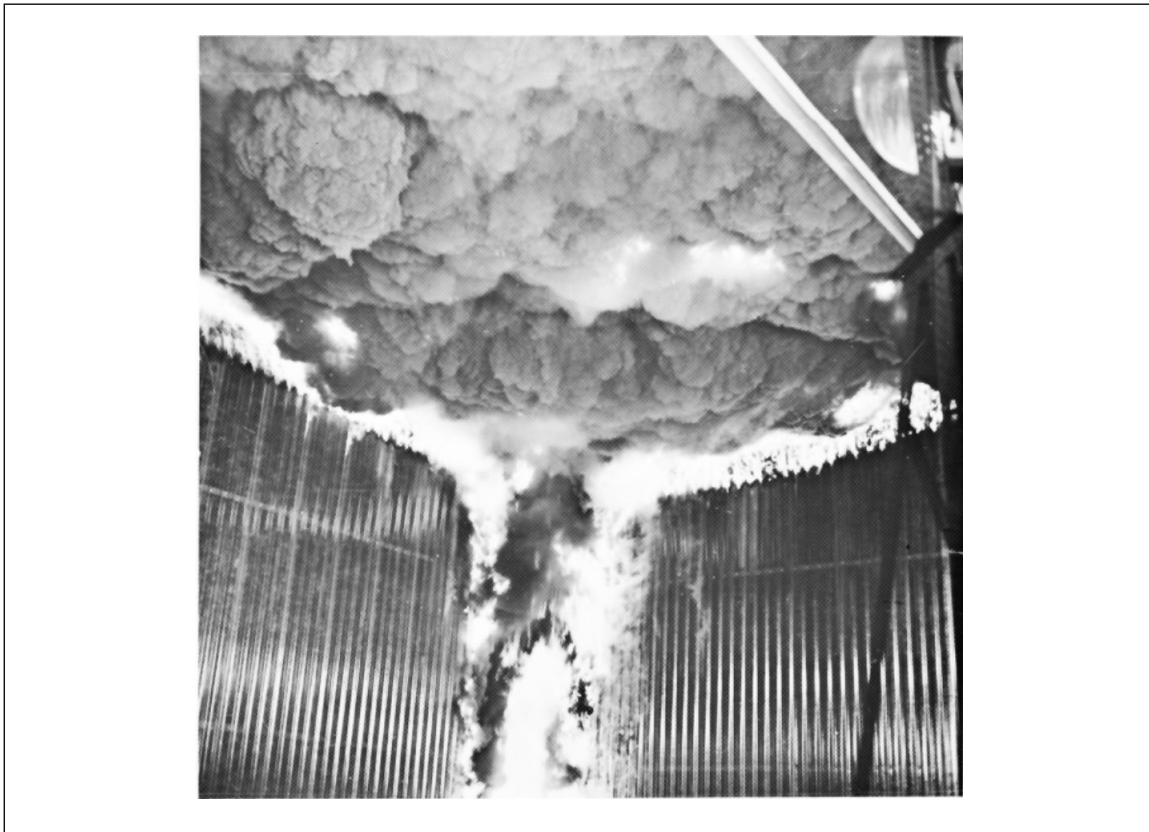
Fig. 20. FM corner test of reinforced plastic (flame spread = 25).
