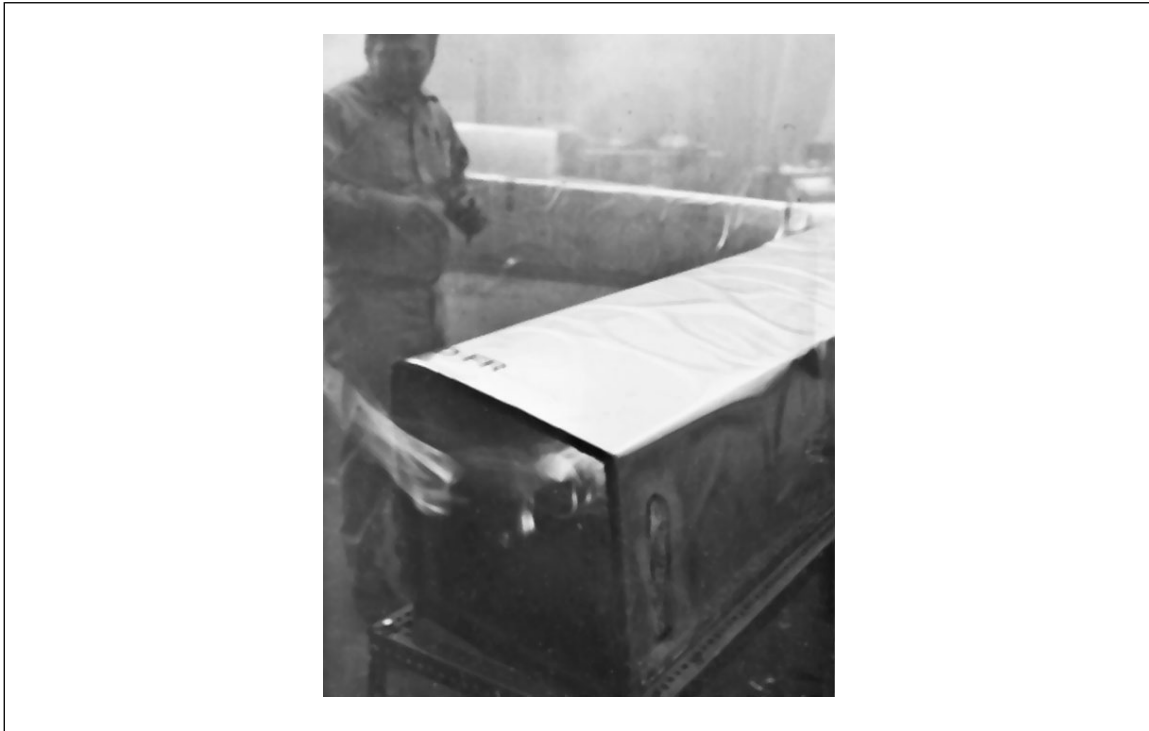
Fig. 2. FM duct test (This fibrous glass specimen has a 25 flame spread.)
