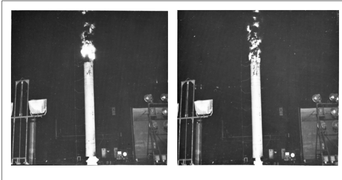
Fig. 3. Vertical duct test (Passed Parallel Panel Test and had 25 flame spread.)
