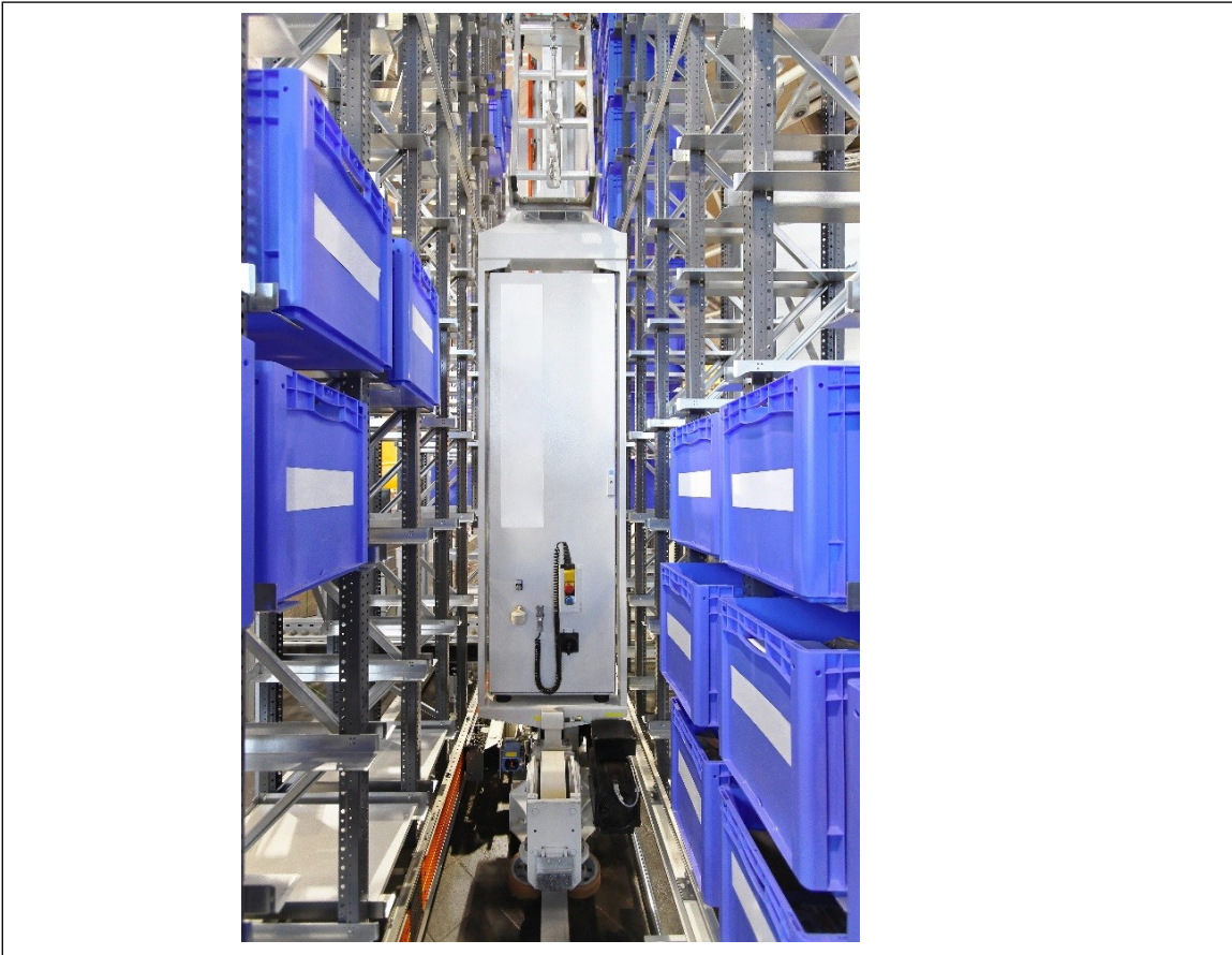
Fig. 3.1.1(d). Example of a crane robot that moves within the storage aisle on a rail located at ground level
