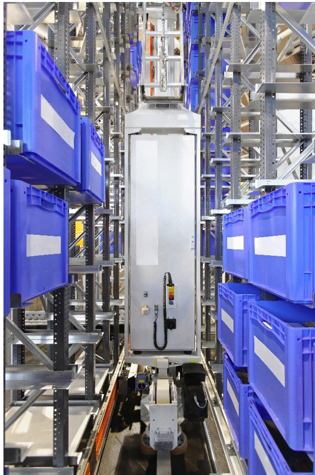
Fig. 60. Example of motorized automated picking robot in a mini-load ASRS storage arrangement with open-top unexpanded plastic containers
