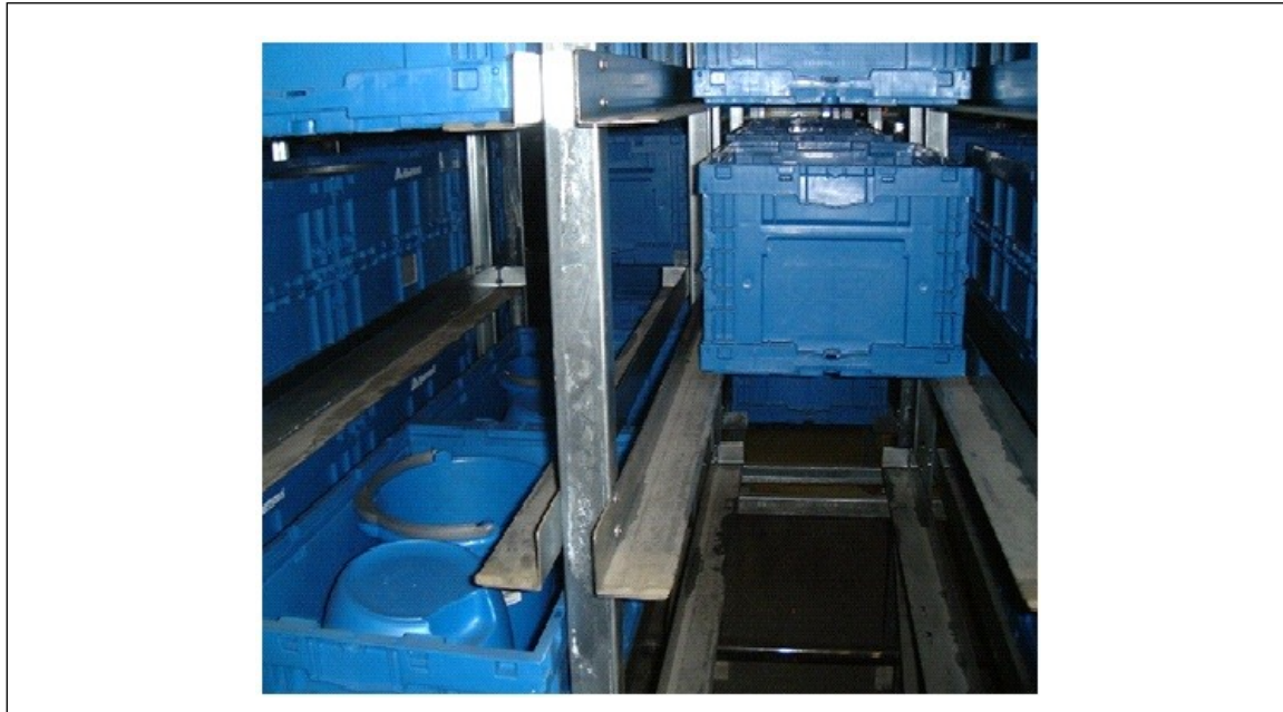
Fig. 57. Example of open-top plastic containers in mini-load ASRS storage arrangement
