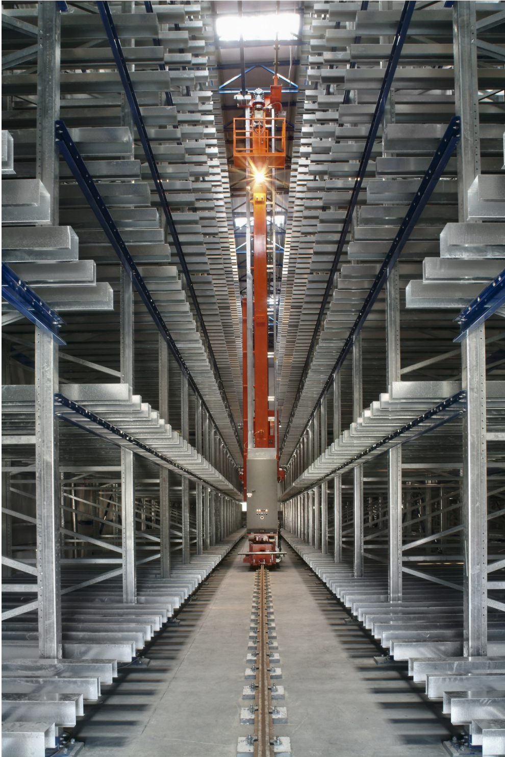
Fig. 58. Example of an empty mini-load ASRS storage arrangement where rack uprights are about 2 to 3 in. (50 to 75 mm) wide and about 2 ft (0.6 m) horizontally apart
