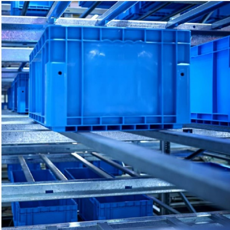
Fig. 2. Example of a shuttle horizontal-loading ASRS
