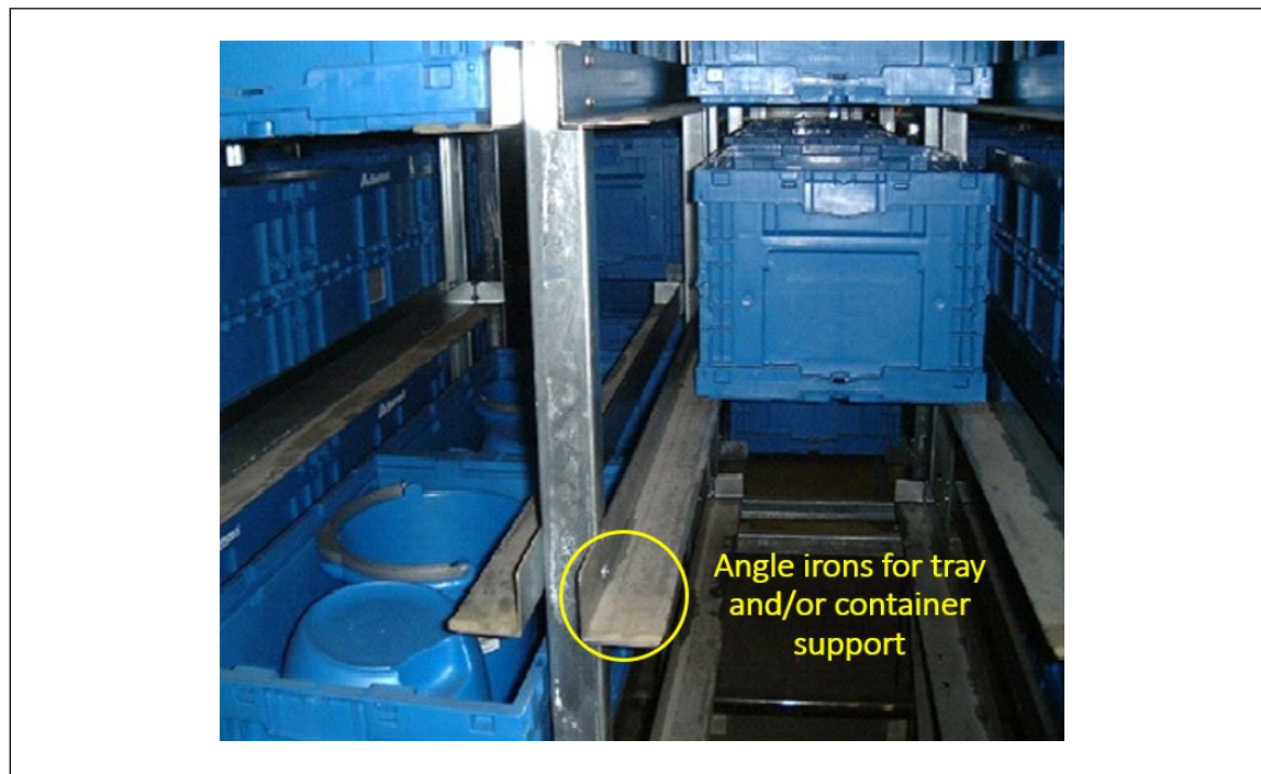
Fig. 3. Example of a mini-load ASRS having angle irons that support the trays and/or containers
