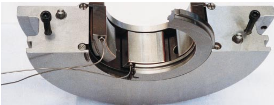
Fig. 3.1.1-2. Typical tilting-pad journal bearing with temperature detective devices (General Electric Company, all rights reserved, used with permission)
