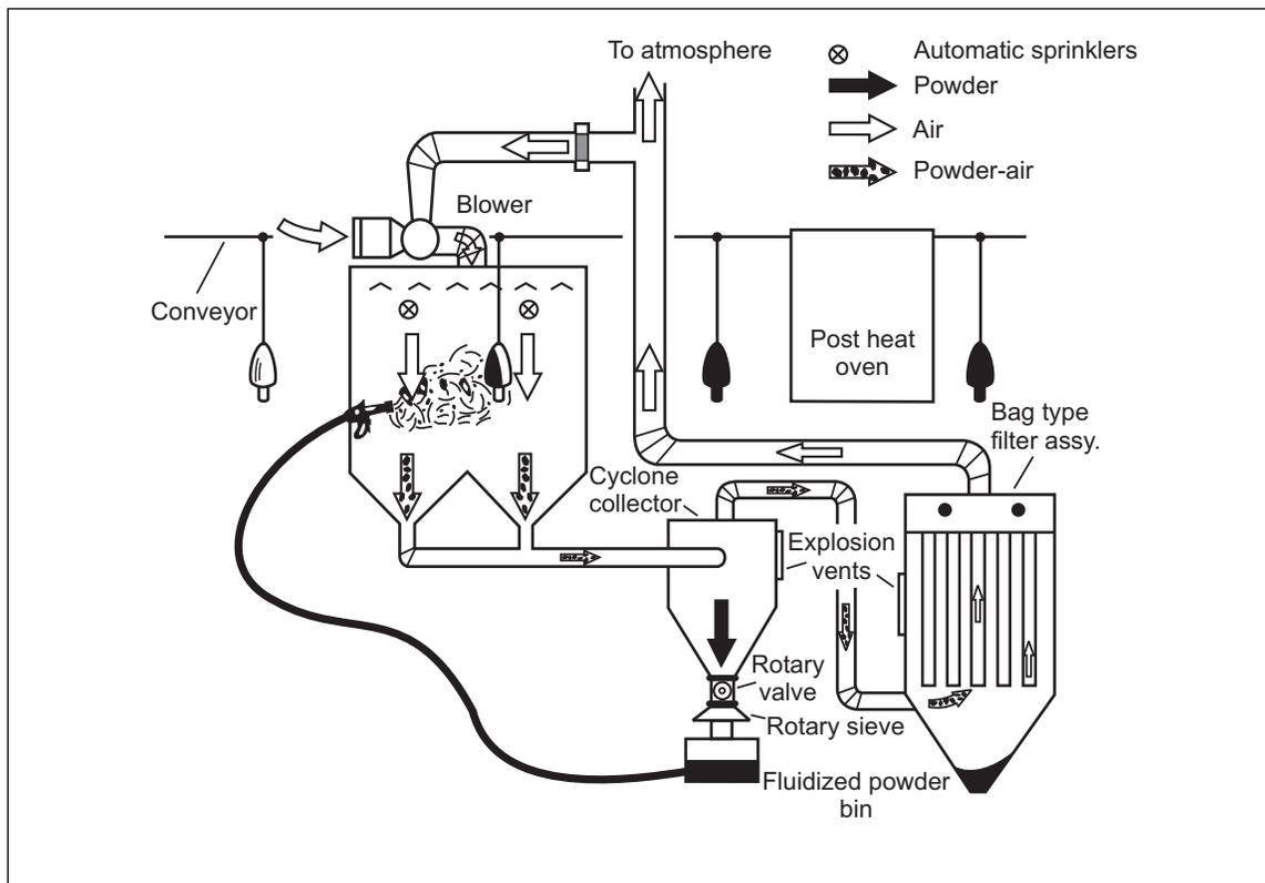
Fig. 14. Manual spray booth with partial recirculation of filtered air
