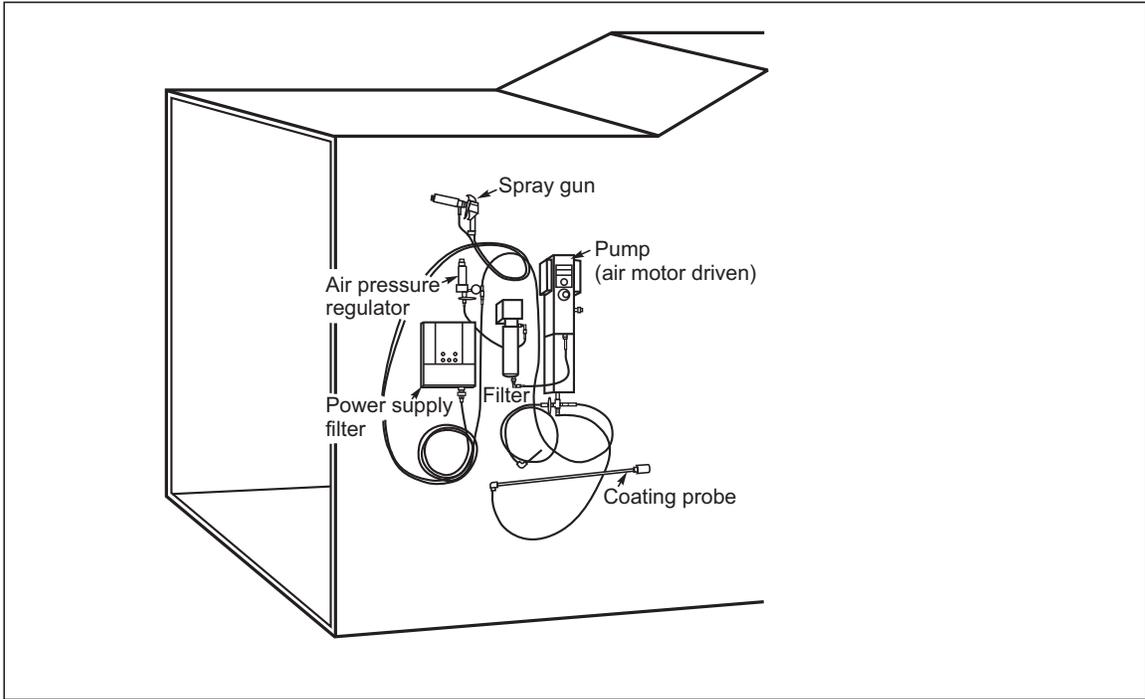
Fig. 11. Airless electrostatic spray system
