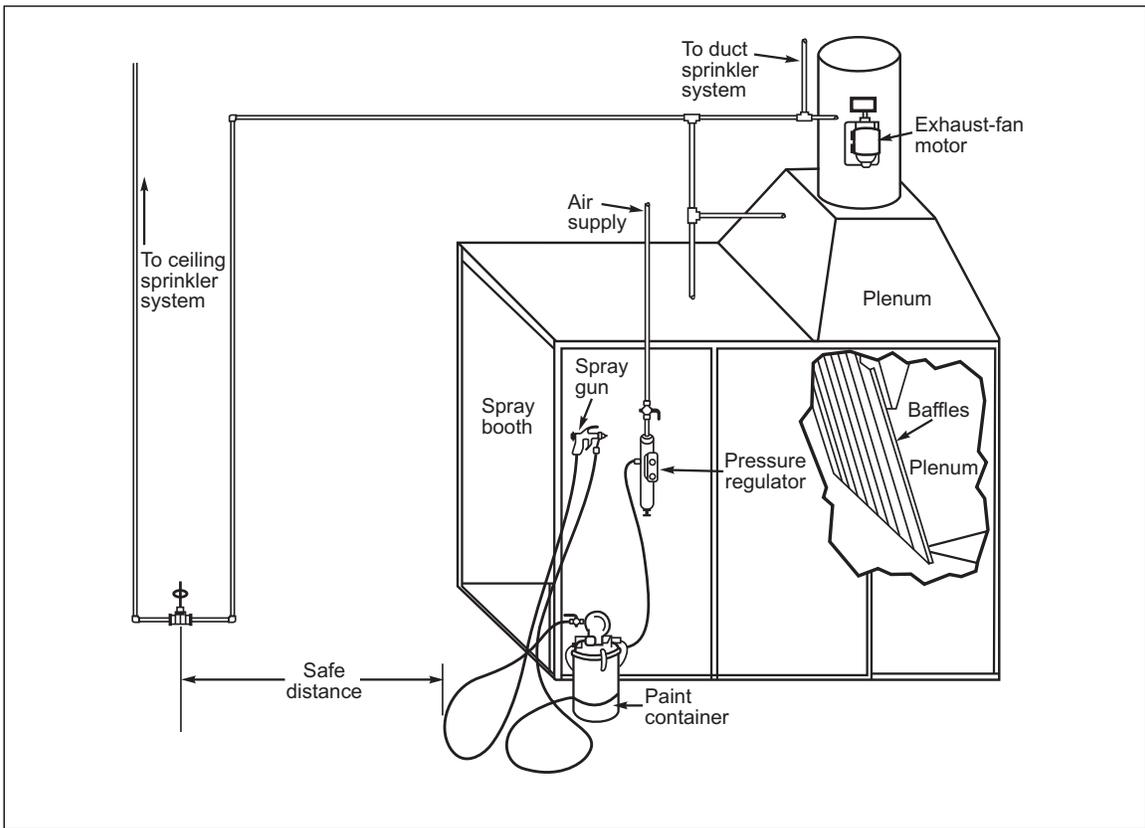
Fig. 12. Dry filter spray booth equipped with baffles
