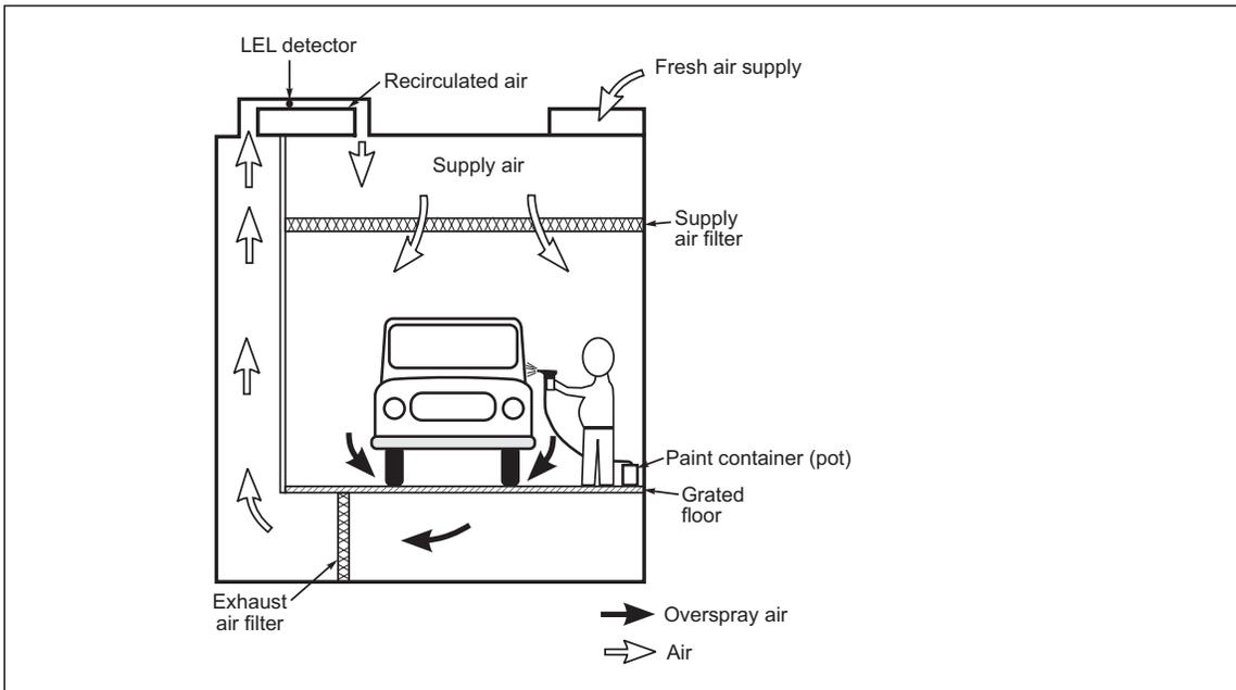
Fig. 2. Dry filter (down draft) spray booth with air being recirculated into booth; LEL detector is also shown (sprinkler protection is not shown)
