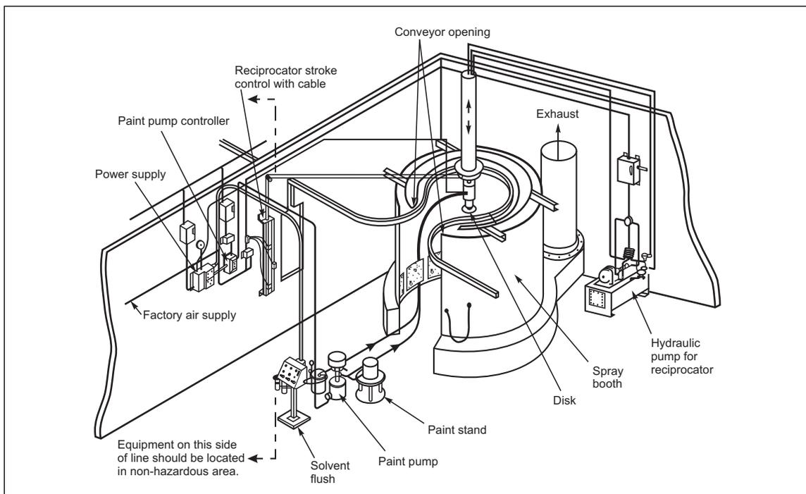
Fig. 9. Electrostatic spray system, rotating disk type
