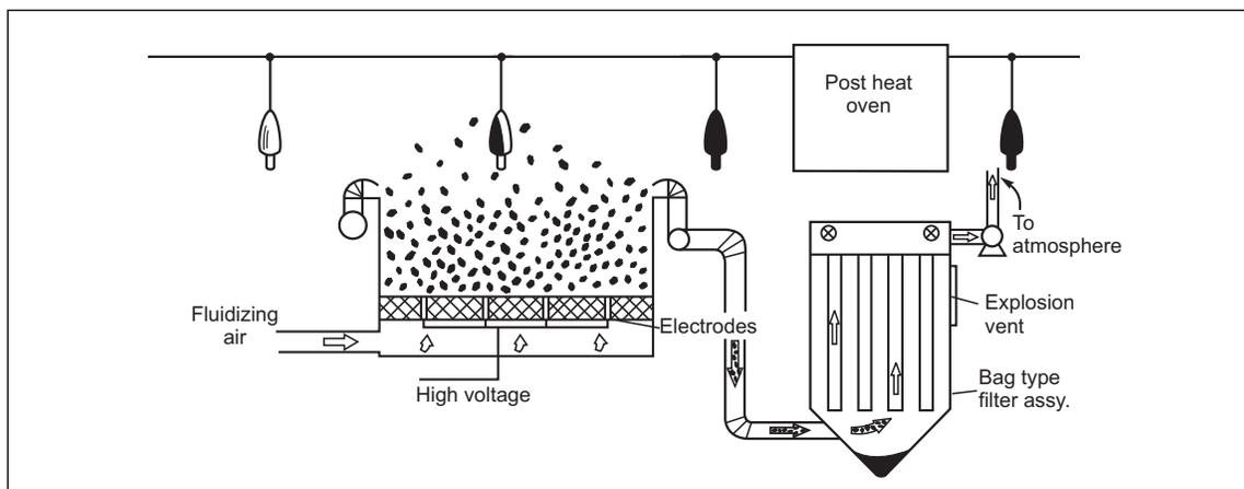
Fig. 16. Electrostatic fluidized bed with perimeter exhaust system
