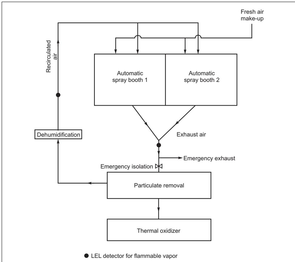
Fig. 17. Example of an off-gas treatment system for a multiple automatic ignitable liquid spray booth operation
