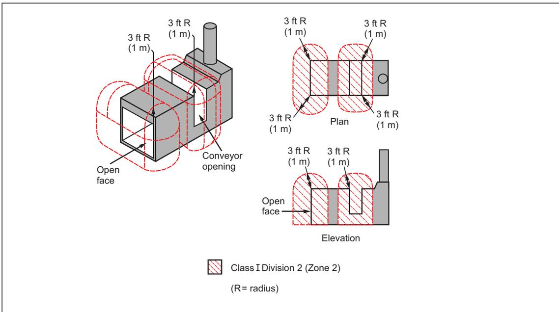
Fig. 6. Class I Division 2 (Zone 2) areas adjacent to a closed-top, open-face or open-front spray operation
