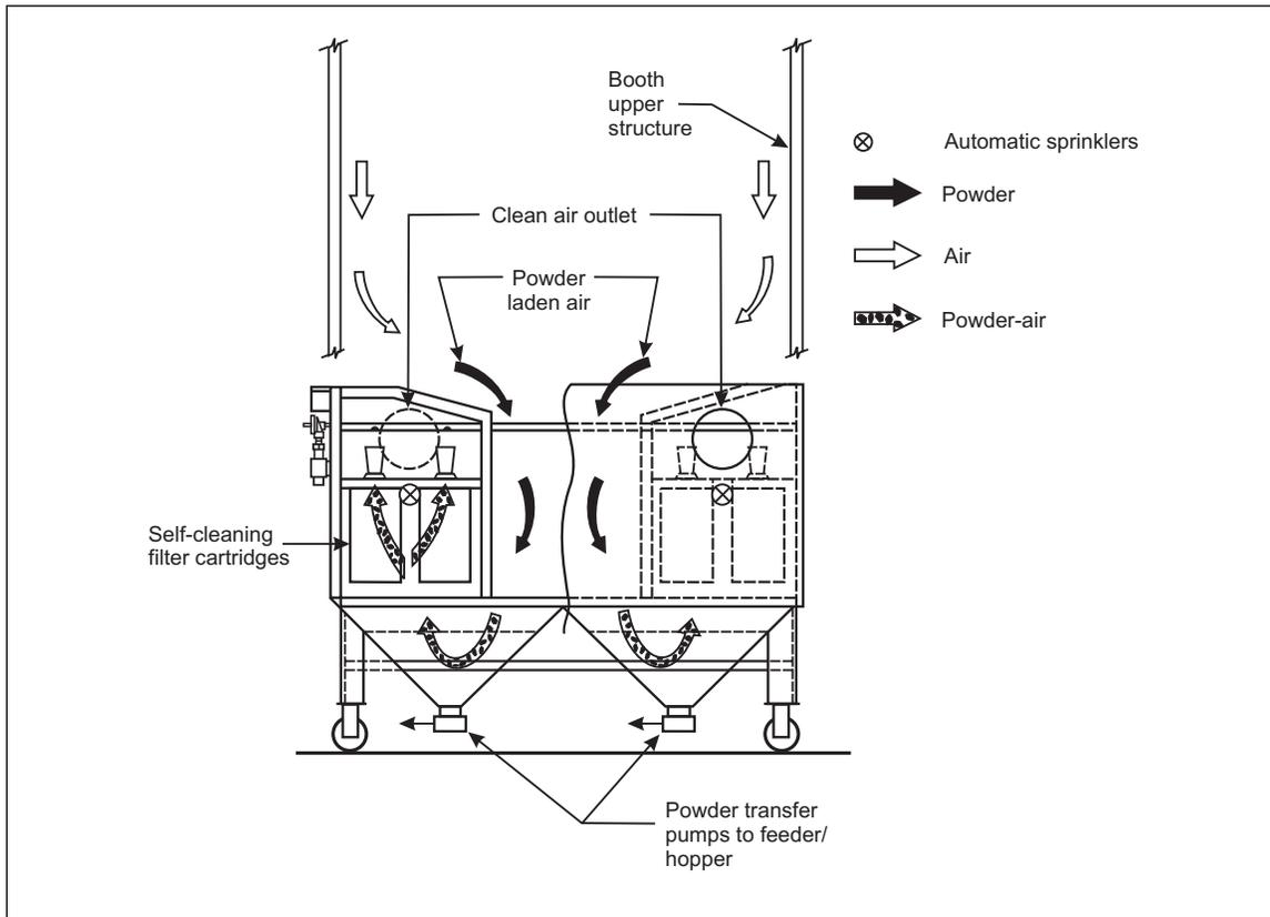
Fig. 15. Integrated booth design with cartridge filter system in upper part of booth hopper
