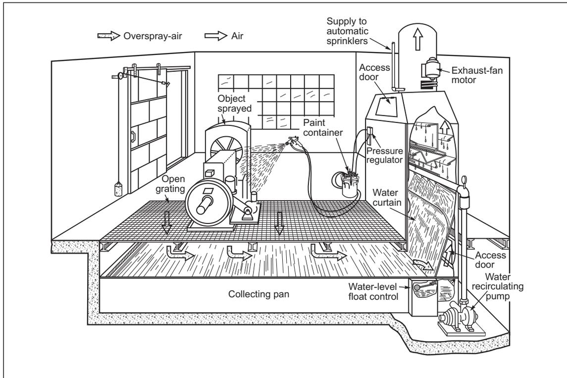
Fig. 13. Downdraft water wash spray booth (room sprinkler system not shown)
