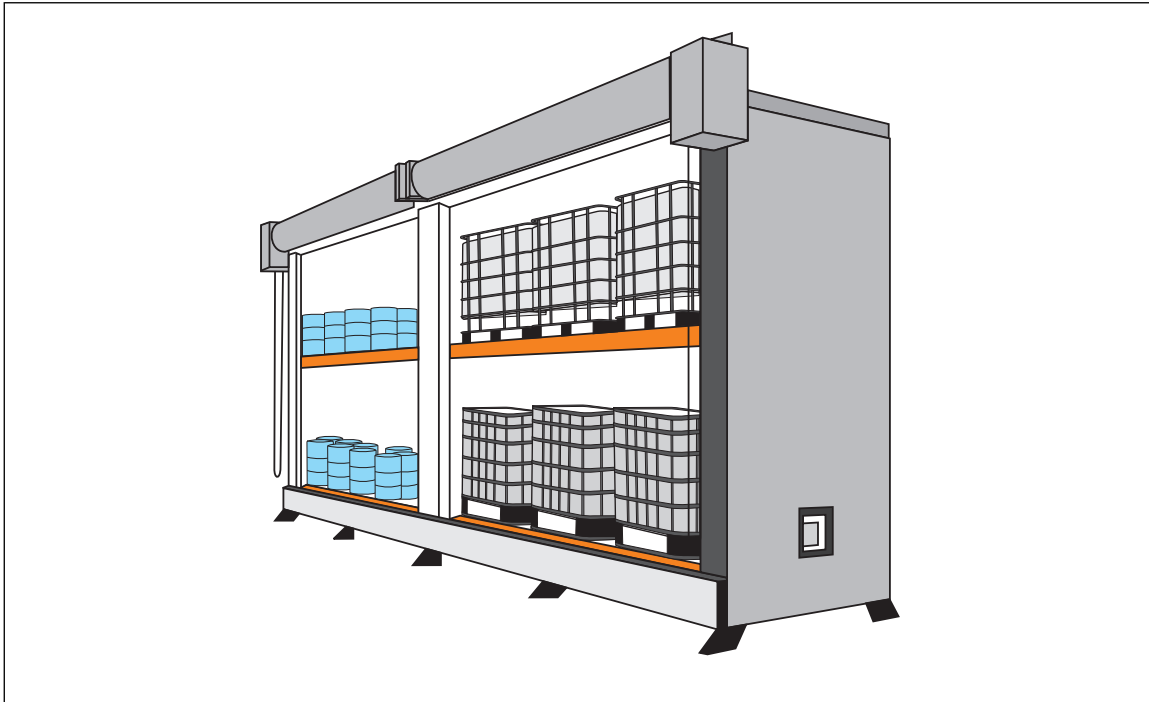
Fig. 2.2.3.2. Ignitable liquid storage locker
