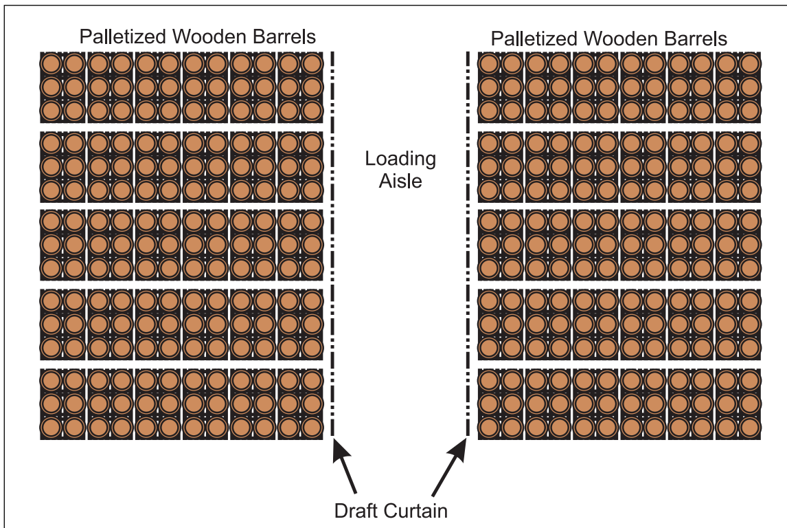
Fig. 2.4.8.3.A. Loading aisle draft curtain arrangement (plan view)
