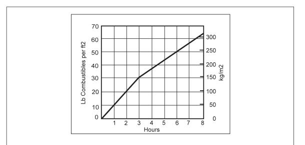
Fig. 1. Weights per square foot and square meters of ordinary (Class A) combustibles required to produce fire severities approximately the ASTM curve for various periods of duration. (Data from Bureau of Standards tests as reported in BM S92.)
