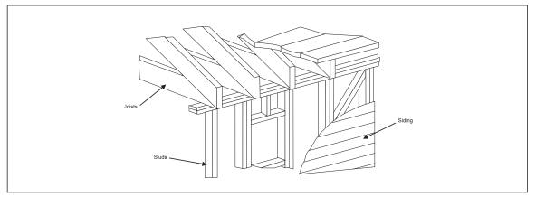
Fig. 14. Wood frame construction.
