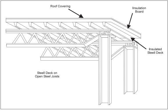
Fig. 11. Insulated steel deck on steel framing. (Note: above deck assembly should be of limited combustibility—see Section C.4)
