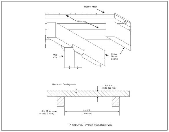
Fig. 12. Plank-on-timber construction.
