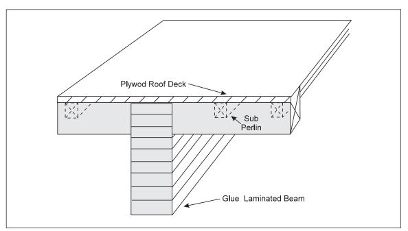
Fig. 15. Typical plywood diaphragm roof deck (not to scale).
