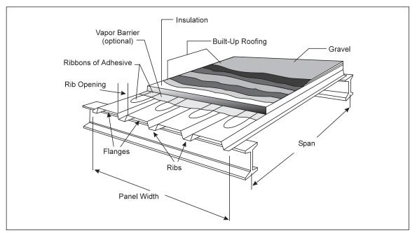
Fig. 17. "Old Style" Class 1 insulated steel deck roof using limited quantities (ribbons) of adhesive to secure insulation and vapor barrier.
