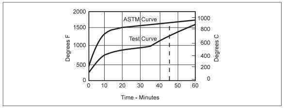
Fig. 2. The area, in degree-hours, under the test curve for 60 minutes is the same as the area under the ASTM curve for 45 minutes. Therefore, the severity of the fire exposure under both curves, up to these respective time limits, is approximately the same.
