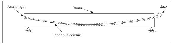
Fig. 9. Post-tensioned concrete beam.
